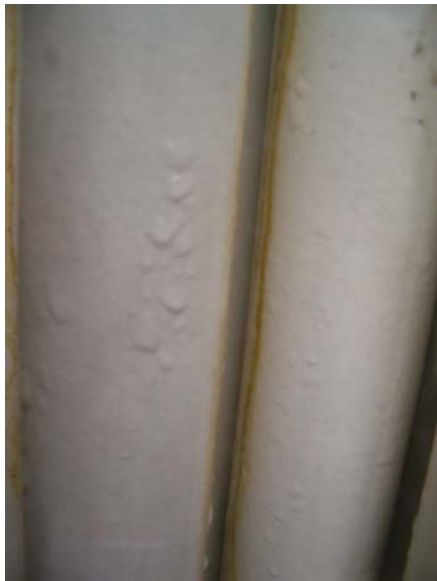
Figure 22. Photograph of the device and operation evolution working as an indirect evaporative cooler under condensation conditions
