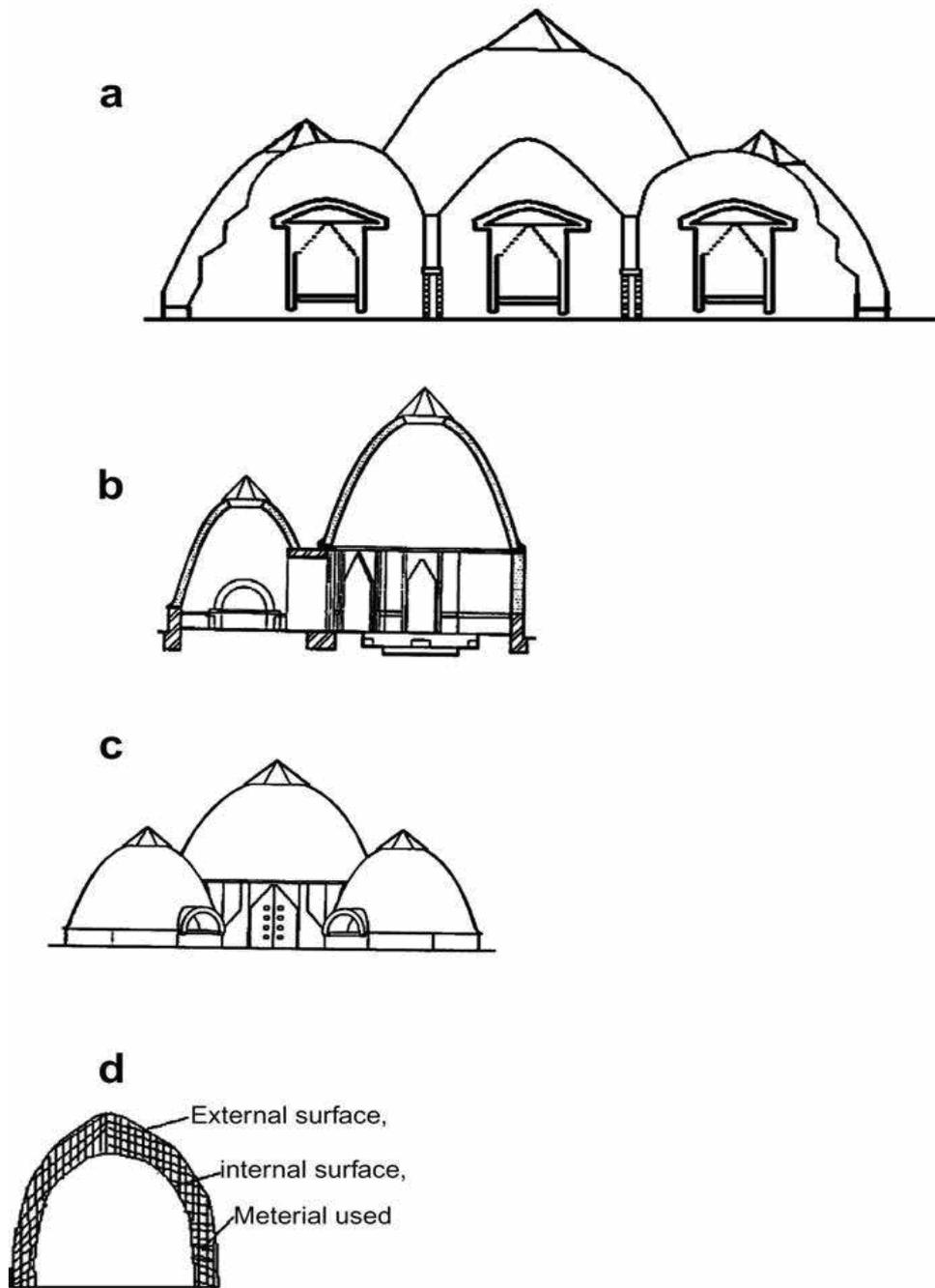
Figure 13. Adobe house (a) front view (b) side view (c) rear view (d) schematic diagram for material calculation
