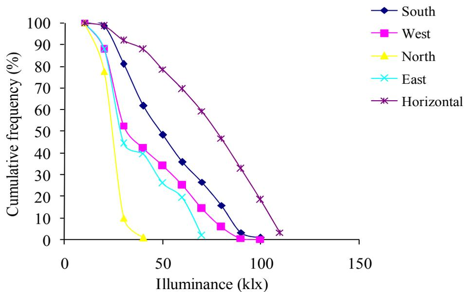
Figure 11. Cumulative frequency distribution for the hourly global illuminances for the horizontal and four vertical places
