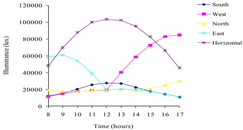
Figure 7. Average global illuminance for horizontal and four vertical surfaces in June
