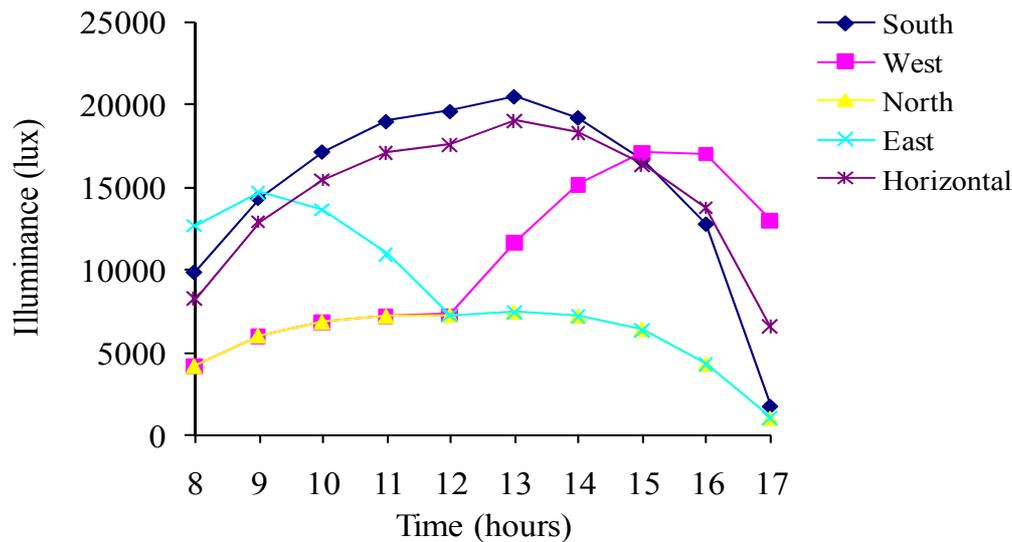
Figure10. Average diffuse illuminance for horizontal and four vertical surfaces in January
