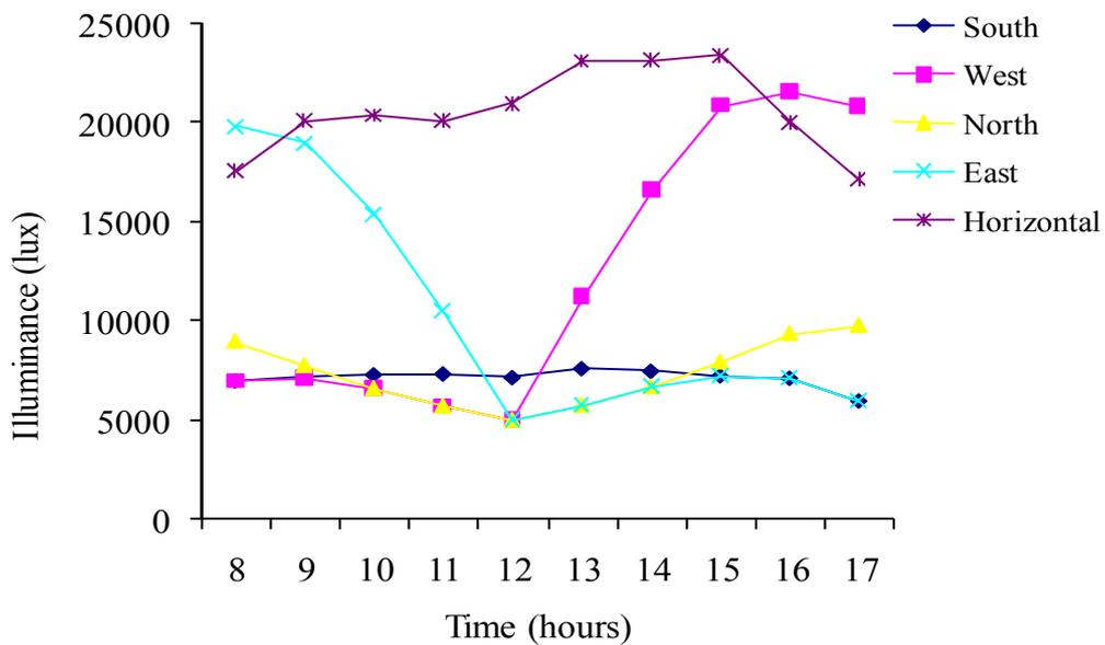
Figure 8. Average diffuse illuminance for horizontal and four vertical surfaces in June
