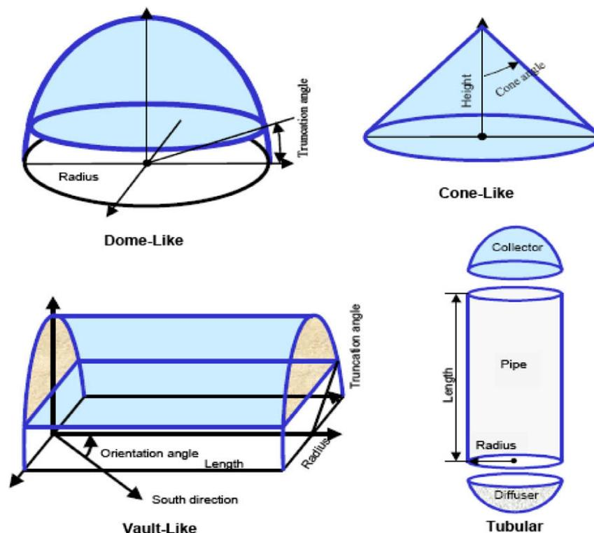
Figure 12. Types of skylight for daylighting in buildings (Laouadi and Atif [18])
