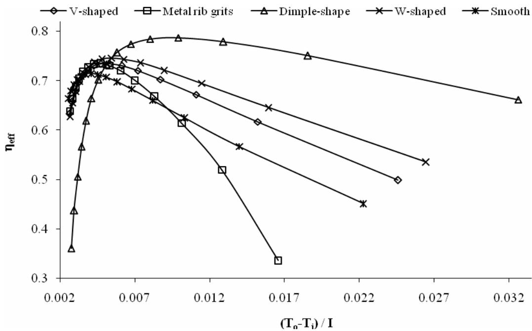
Figure 3. Variation of effective efficiency with temperature rise parameter for various roughness geometries (at  $e/d = 0.025$ ,  $I = 800 \text{ W/m}^2$  and  $U_L = 5 \text{ W/m}^2\text{K}$ )
