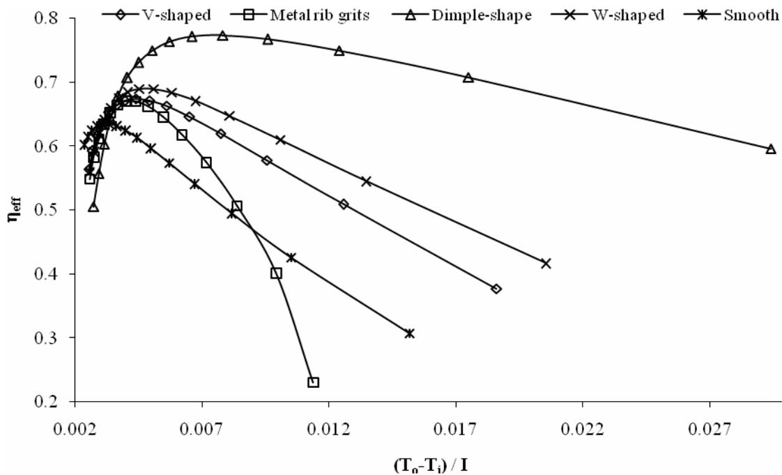
Figure 8. Variation of effective efficiency with temperature rise parameter for various roughness geometries (at  $e/d = 0.035$ ,  $I = 800 \text{ W/m}^2$  and  $U_L = 10 \text{ W/m}^2\text{K}$ )
