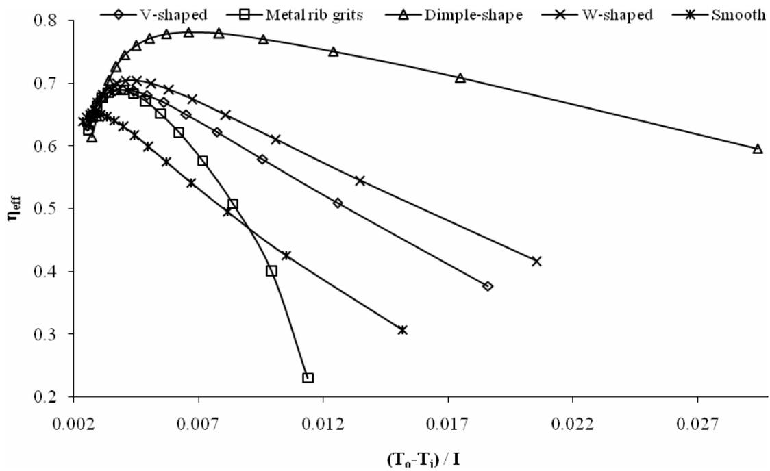
Figure 6. Variation of effective efficiency with temperature rise parameter for various roughness geometries (at  $e/d = 0.035$ ,  $I = 1200 \text{ W/m}^2$  and  $U_L = 10 \text{ W/m}^2\text{K}$ )
