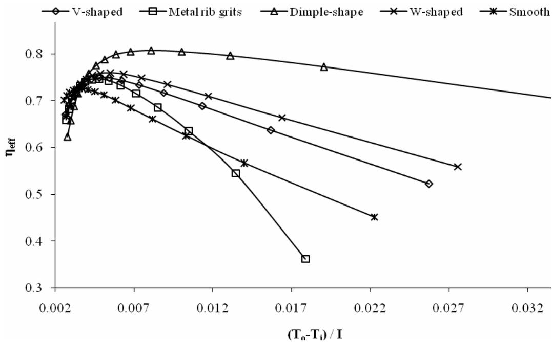
Figure 5. Variation of effective efficiency with temperature rise parameter for various roughness geometries (at  $e/d = 0.035$ ,  $I = 1200 \text{ W/m}^2$  and  $U_L = 5 \text{ W/m}^2\text{K}$ )
