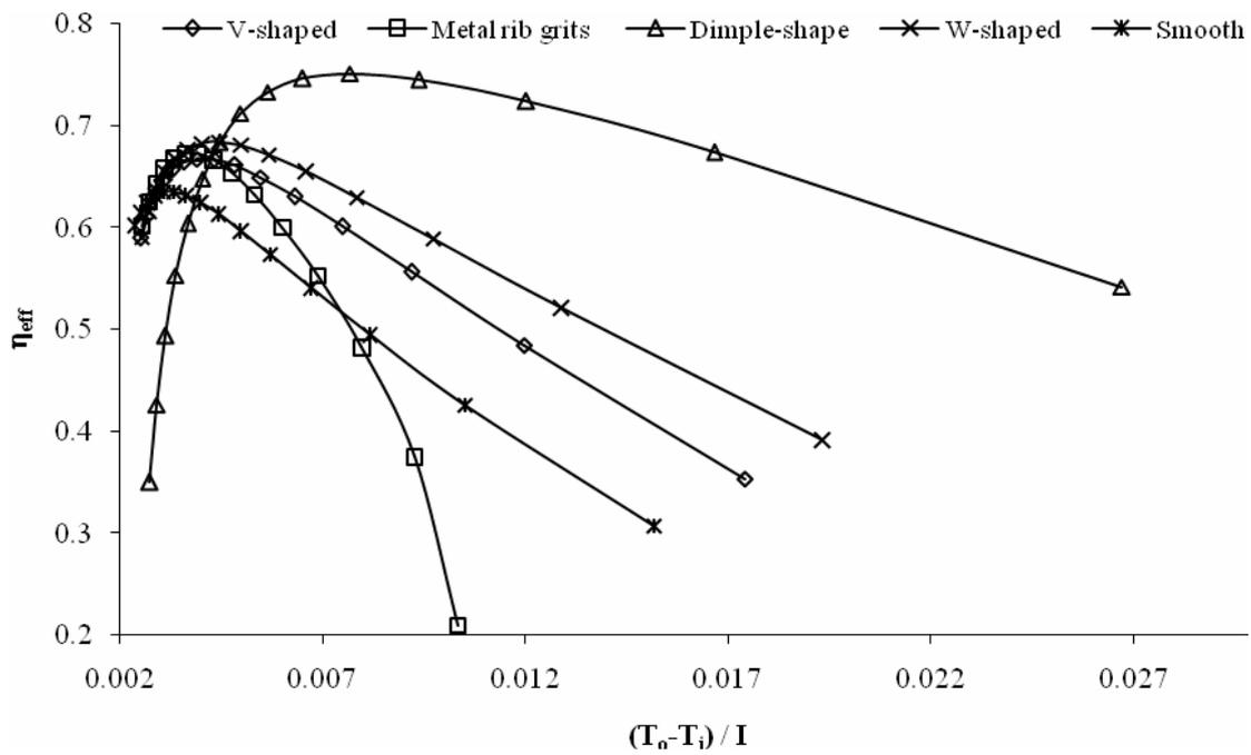
Figure 4. Variation of effective efficiency with temperature rise parameter for various roughness geometries (at  $e/d = 0.025$ ,  $I = 800 \text{ W/m}^2$  and  $U_L = 10 \text{ W/m}^2\text{K}$ )
