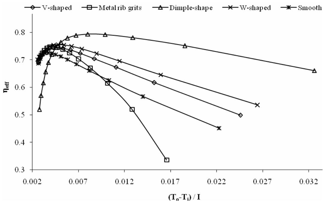
Figure 1. Variation of effective efficiency with temperature rise parameter for various roughness geometries (at  $e/d = 0.025$ ,  $I = 1200 \text{ W/m}^2$  and  $U_L = 5 \text{ W/m}^2\text{K}$ )
