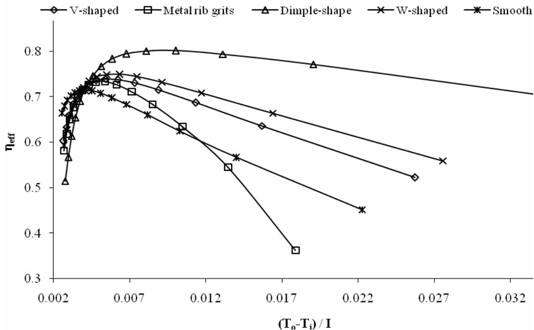
Figure 7. Variation of effective efficiency with temperature rise parameter for various roughness geometries (at  $e/d = 0.035$ ,  $I = 800 \text{ W/m}^2$  and  $U_L = 5 \text{ W/m}^2\text{K}$ )
