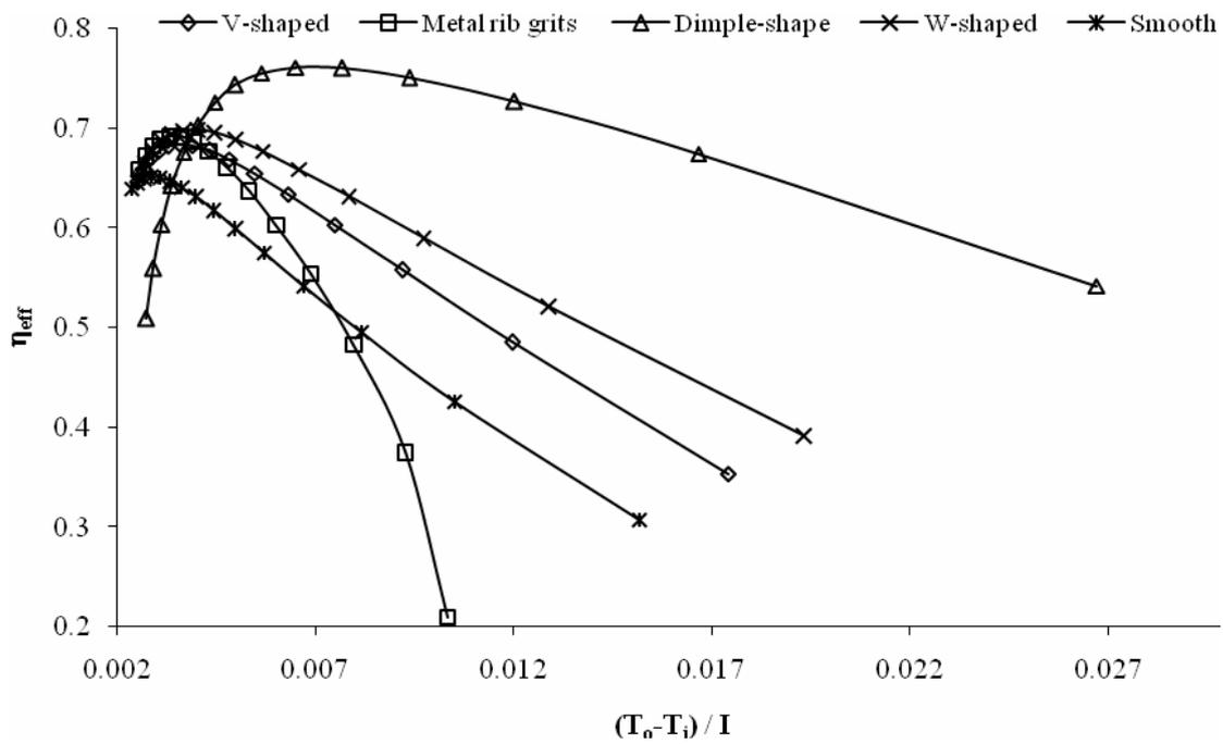
Figure 2. Variation of effective efficiency with temperature rise parameter for various roughness geometries (at  $e/d = 0.025$ ,  $I = 1200 \text{ W/m}^2$  and  $U_L = 10 \text{ W/m}^2\text{K}$ )
