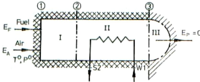
Figure 7. The boiler regions (I: combustion, II: heat transfer, III: exhaust)
