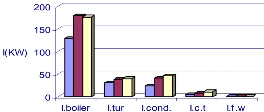
Figure 3. Irreversibility of components at the boiler pressure of 5 bar
