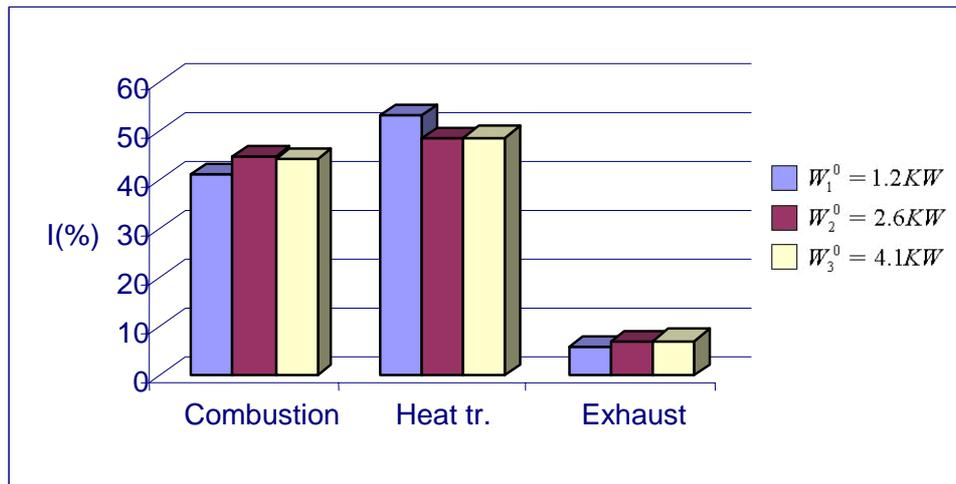
Figure 10. Percentage ratio of irreversibility in the boiler regions at the boiler pressure of 6 bar and different output works
