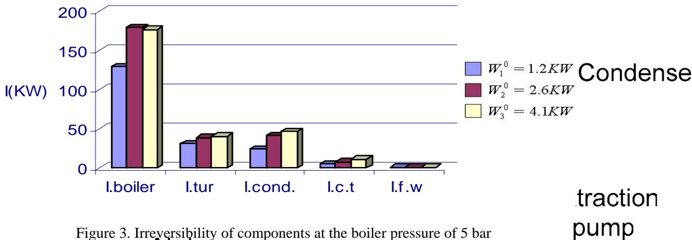
Figure 3. Irreversibility of components at the boiler pressure of 5 bar
