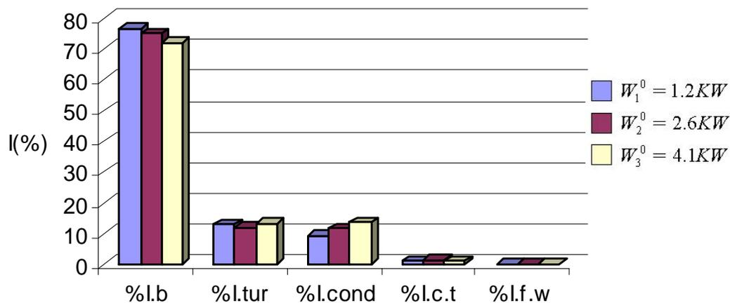
Figure 5. Percentage ratio of irreversibility in components at the boiler pressure of 7 bar
