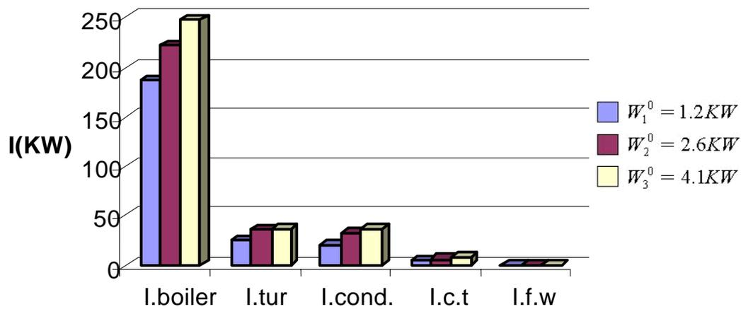
Figure 4. Irreversibility of components at the boiler pressure of 8 bar
