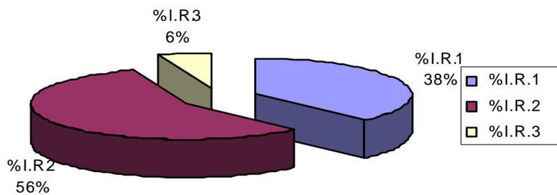
Figure 9. Percentage ratio of irreversibility in the boiler regions at the boiler pressure of 8 bar and output work of 1.2 kW
