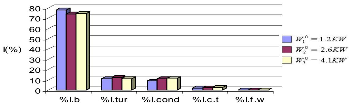
Figure 6. Percentage ratio of irreversibility in components at the boiler pressure of 8 bar
