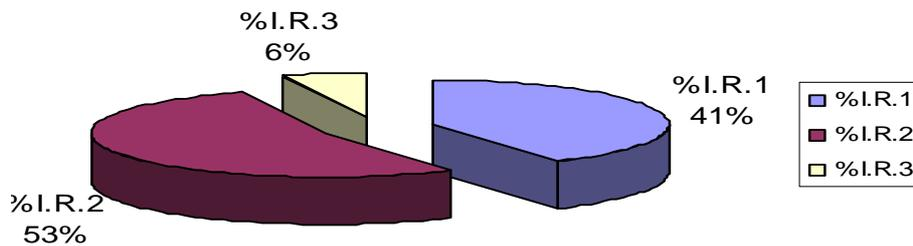
Figure 8. Percentage ratio of irreversibility in the boiler regions at the boiler pressure of 6 bar and output work of 1.2 kW
