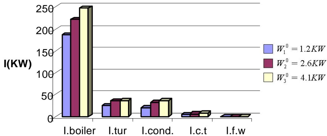
Figure 4. Irreversibility of components at the boiler pressure of 8 bar
