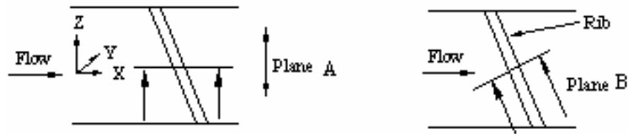
Figure 4. Laser sheet arrangement for PIV measurement of single rib
