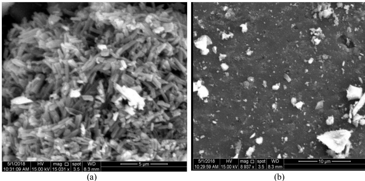
Figure 5. SEM images of  $\text{TiO}_2$  powder Annealing at 500 C° [A] 5 $\mu\text{m}$ , [B] 10 $\mu\text{m}$ .
