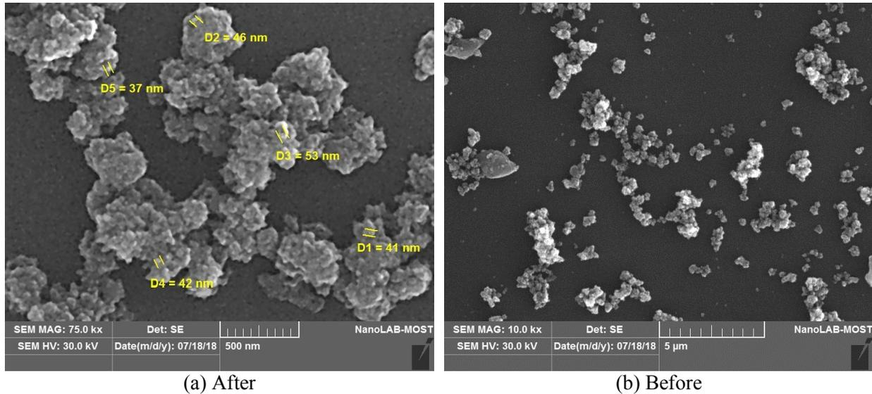
Figure 4. SEM images of  $\text{TiO}_2$  prepared powder [A] 500nm, [B] 5 $\mu\text{m}$ .
