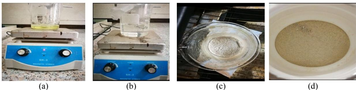
Figure 1. Preparation steps of TiO<sub>2</sub> nanoparticle: (a) TiCl<sub>4</sub> solution added to ethanol, (b) Distilled water was added, (c) The final sol-gel solution dried at 50 °C for 16 h, (d) after treated it at 500 °C to form TiO<sub>2</sub> powder.
