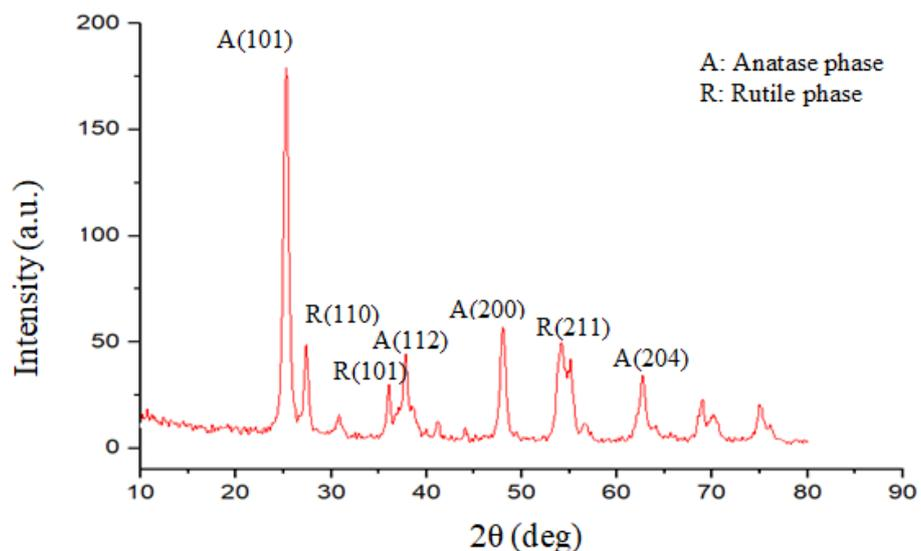
Figure 3. X-ray diffraction pattern of  $\text{TiO}_2$  powder at  $500^\circ\text{C}$ .
