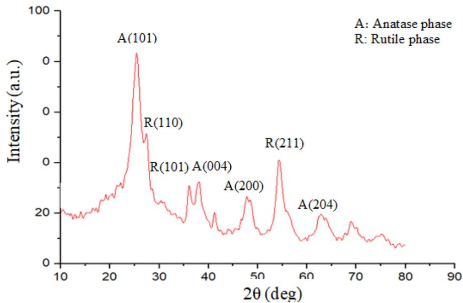
Figure 2. X-ray diffraction of prepared  $\text{TiO}_2$  nano-particles.
