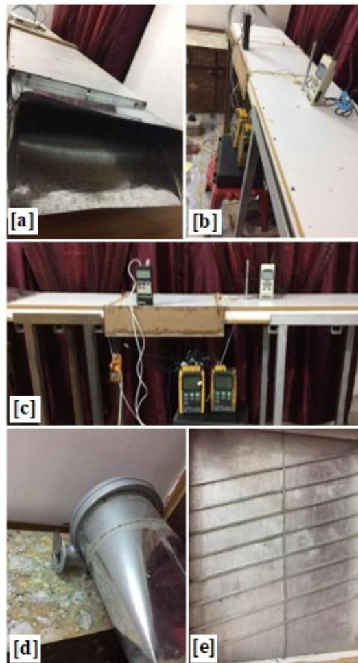
Figure 3. A photograph of the experimental set-up, (a) air intake, (b) inlet section, (c) test section and instrumentations, (d) blower, (e) test plate with attached ribs.
