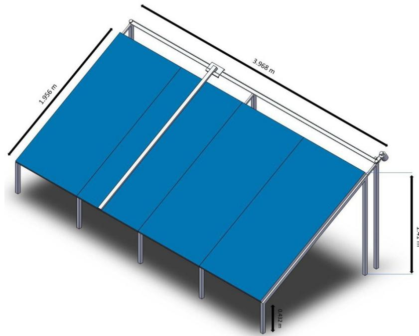
Figure 3. Schematic diagram of solar panels and cleaning system.
