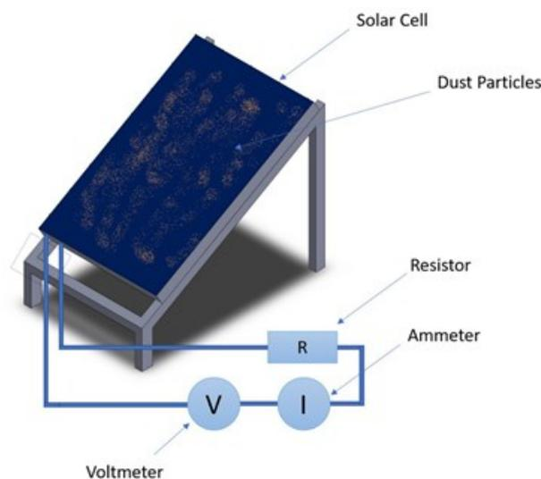
Figure 2. Schematic diagram of solar panel in case of power measuring.
