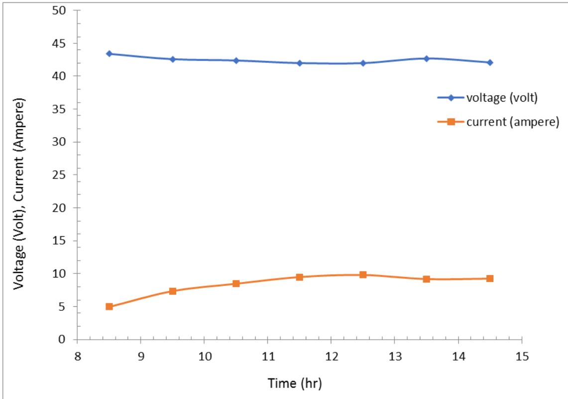
Figure 8. Variation of voltage and current with time during one day for hourly cleaning.
