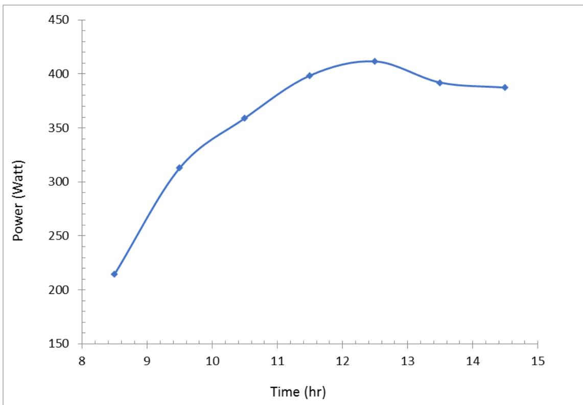
Figure 9. Variation of power with time during one day for hourly wet cleaning.
