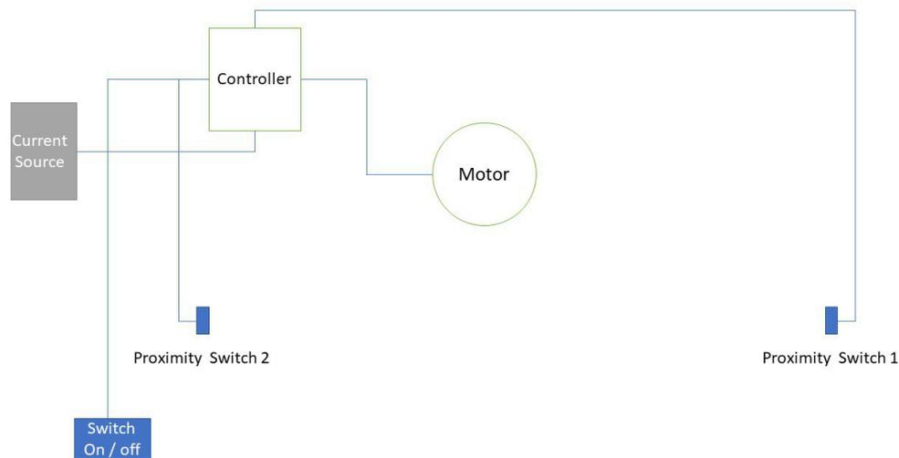
Figure 4. Sketch control circuit for cleaning system.
