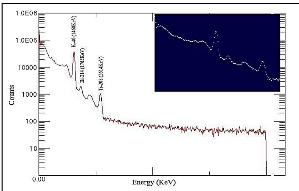
Figure 4. The spectrum of sample B1 (Loof, made in Iraq) in Maestro-32.
