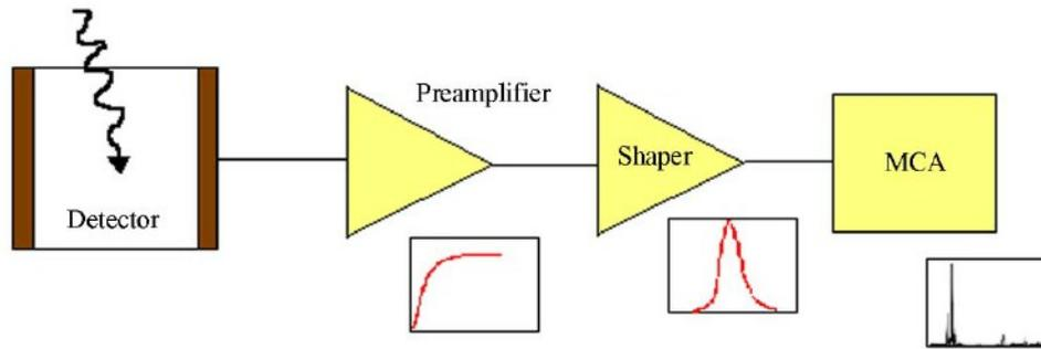
Figure 1. Block diagram of a spectroscopy system.
