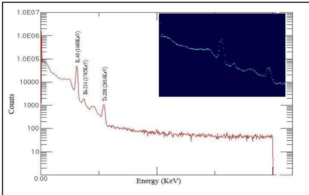
Figure 5. The spectrum of sample B6 (Soft Roll Brad, made in Syria) in Maestro-32.
