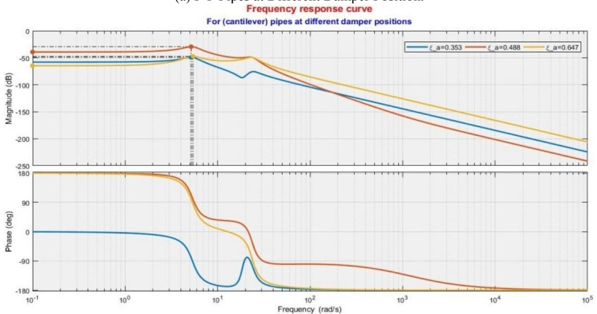
Figure 3. Frequency response curve at different damper positions.
