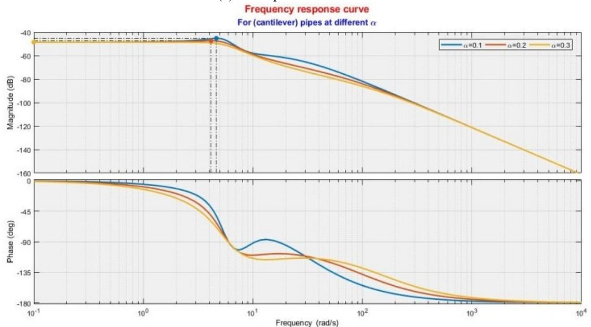
(b) cantilever Pipes at Different  $\alpha$ .Figure 5. Frequency response curve at different  $\alpha$ .
