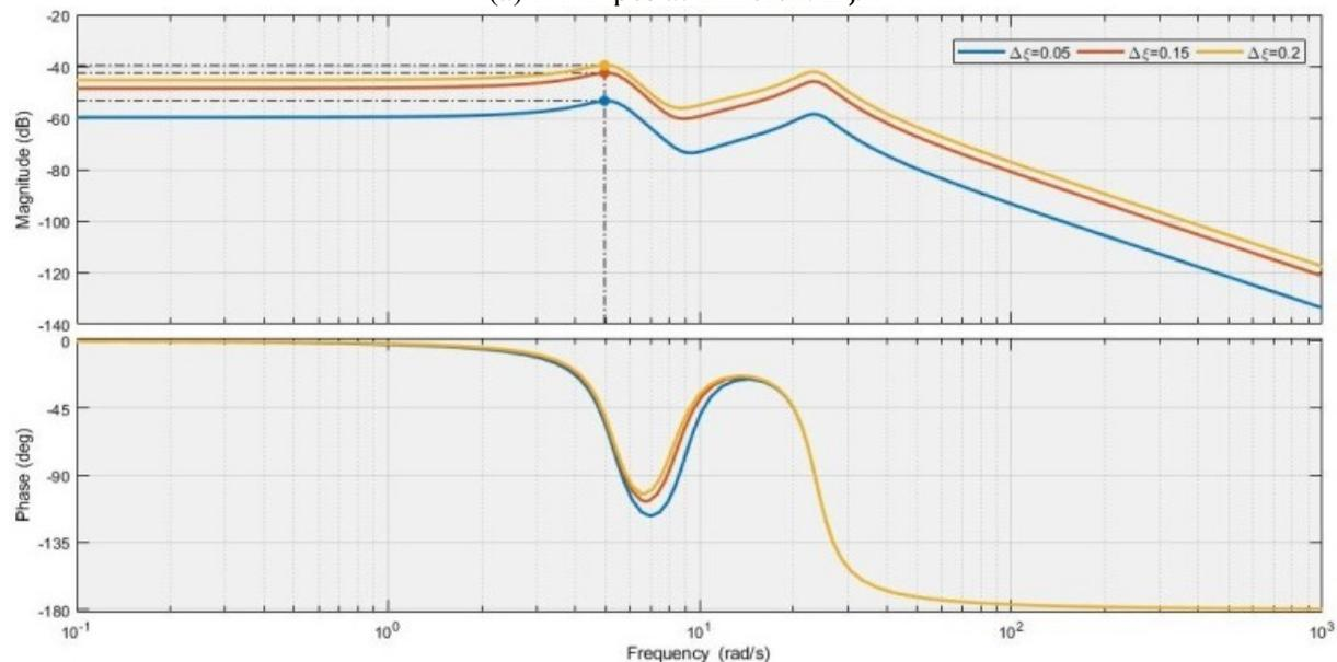
(b) Cantilever Pipes at Different  $\Delta\xi$ .
