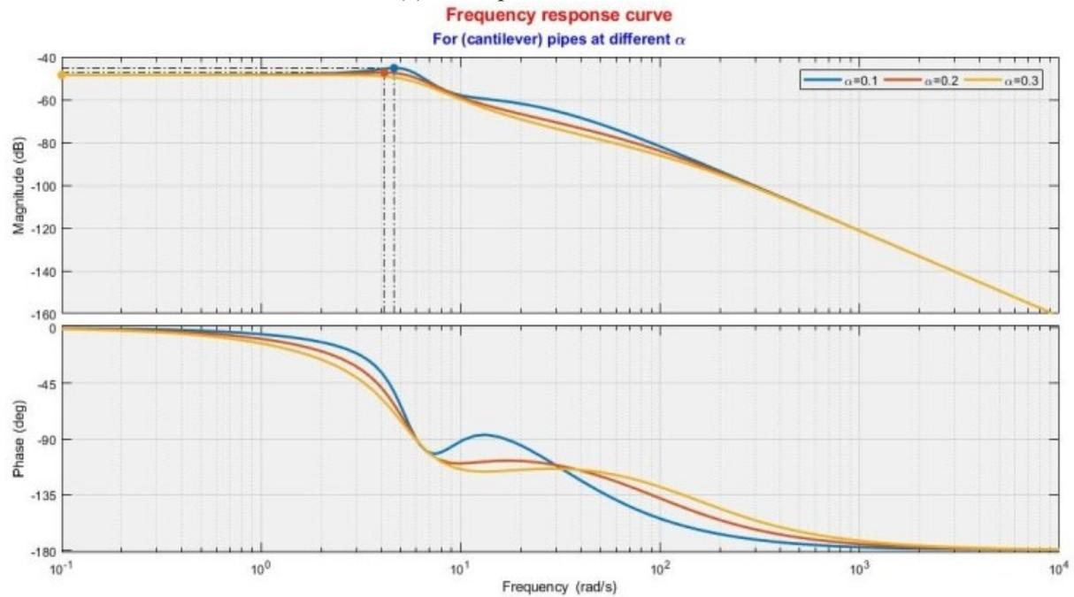
(b) cantilever Pipes at Different  $\alpha$ .
