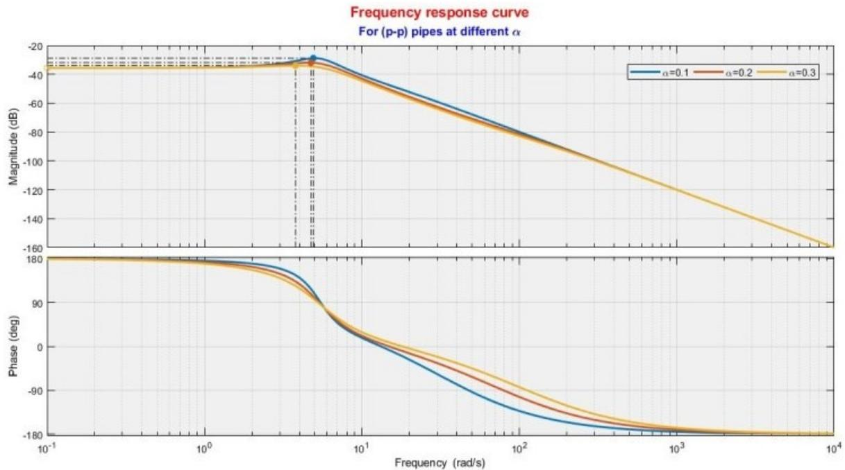
(a) P-P Pipes at Different  $\alpha$ .
