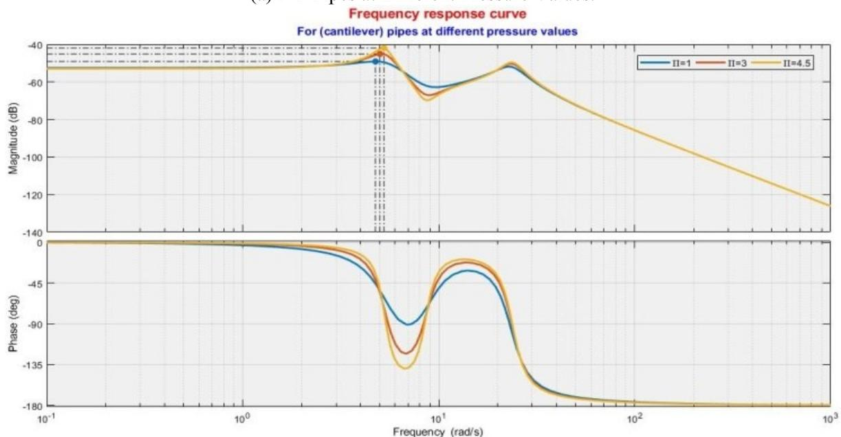
Figure 6. Frequency response curve at different  $\Pi$ .
