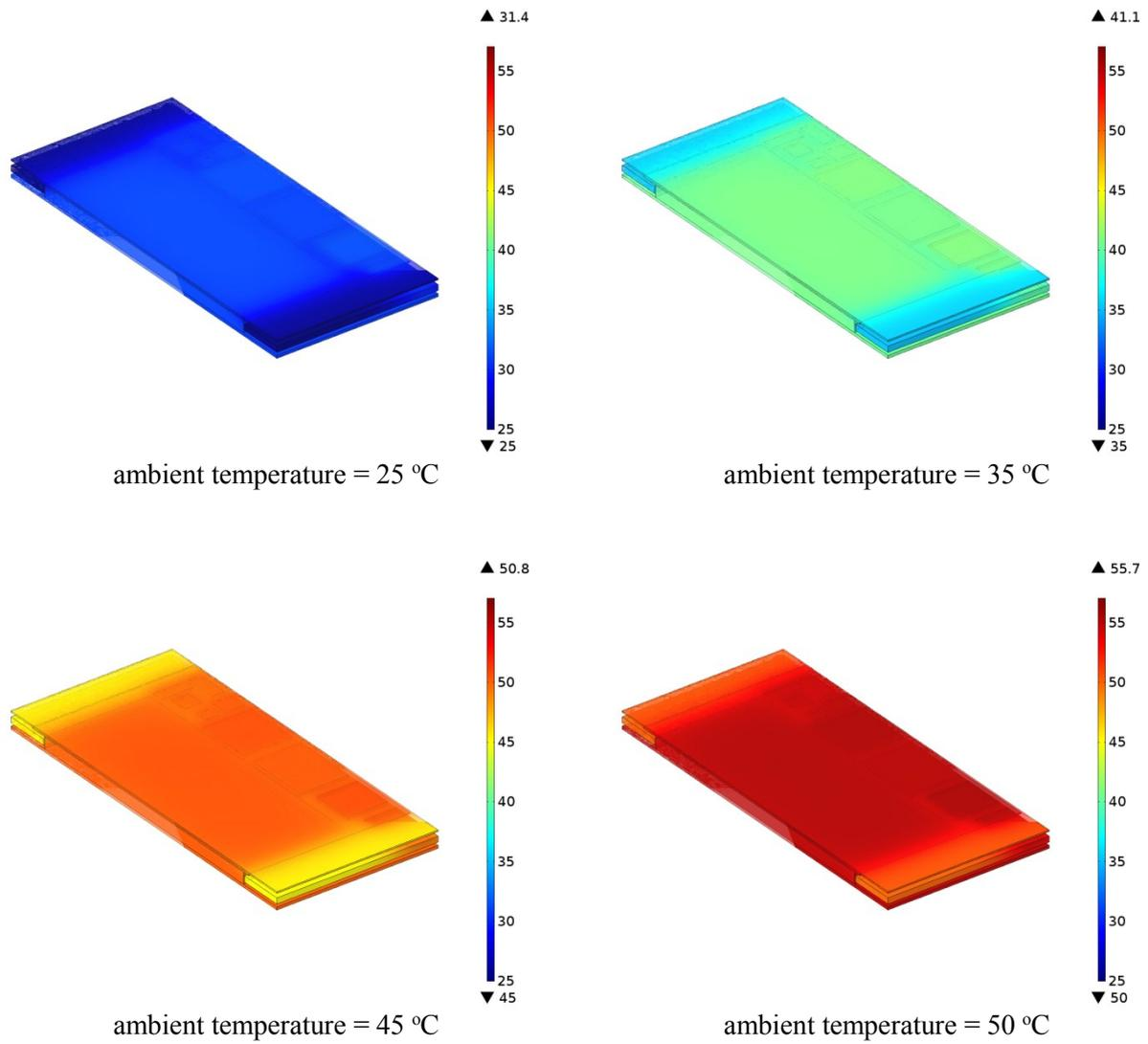
Figure 7. Temperature distribution in iPhone5 [°C] during operating for 15 minutes at ambient temperatures of 25, 35, 45 and 50 °C.
