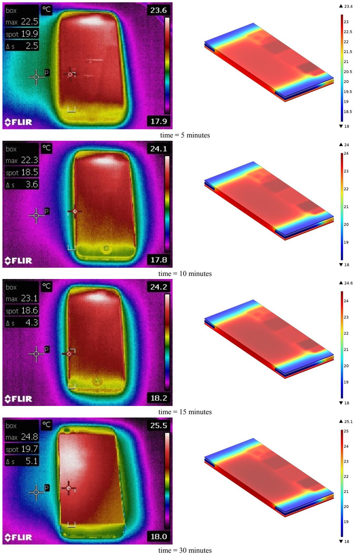
Figure 5. Temperature distribution in iPhone5 [°C] during operating: (left) thermal camera image and (right) CFD simulation.
