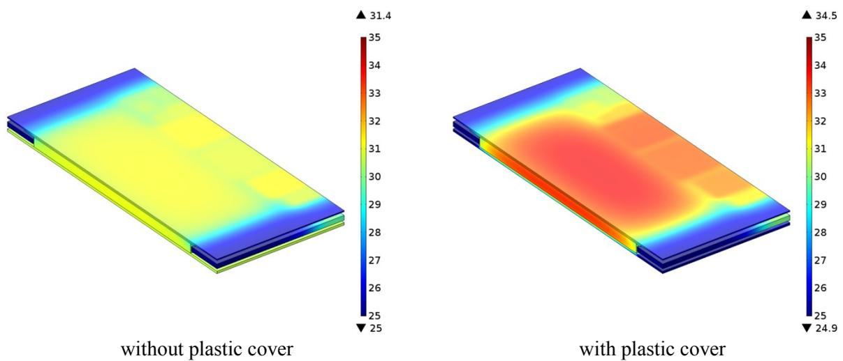
Figure 8. Temperature distribution in iPhone5 [°C] during operating for 15 minutes with and without plastic external cover (attached to the back of iPhone).
