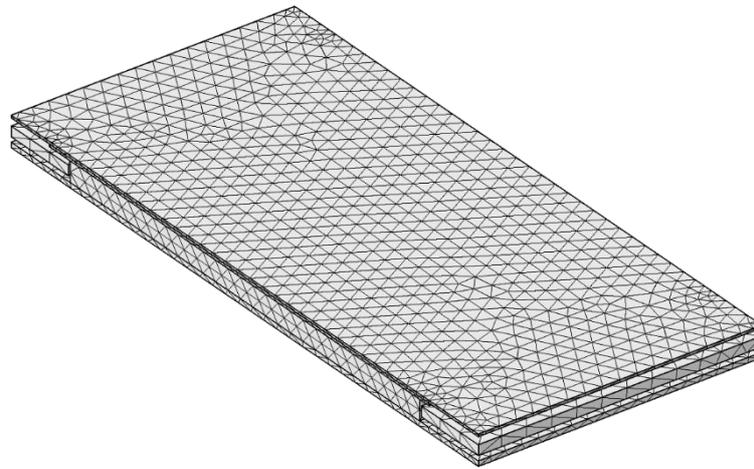
Figure 4. Computational mesh of the computational domain (quadratic).
