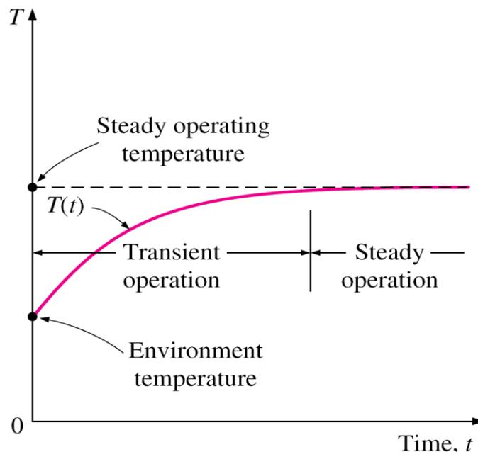
Figure 1. The temperature change of a smartphone component with time as it reaches steady operating temperature after it is turned on.
