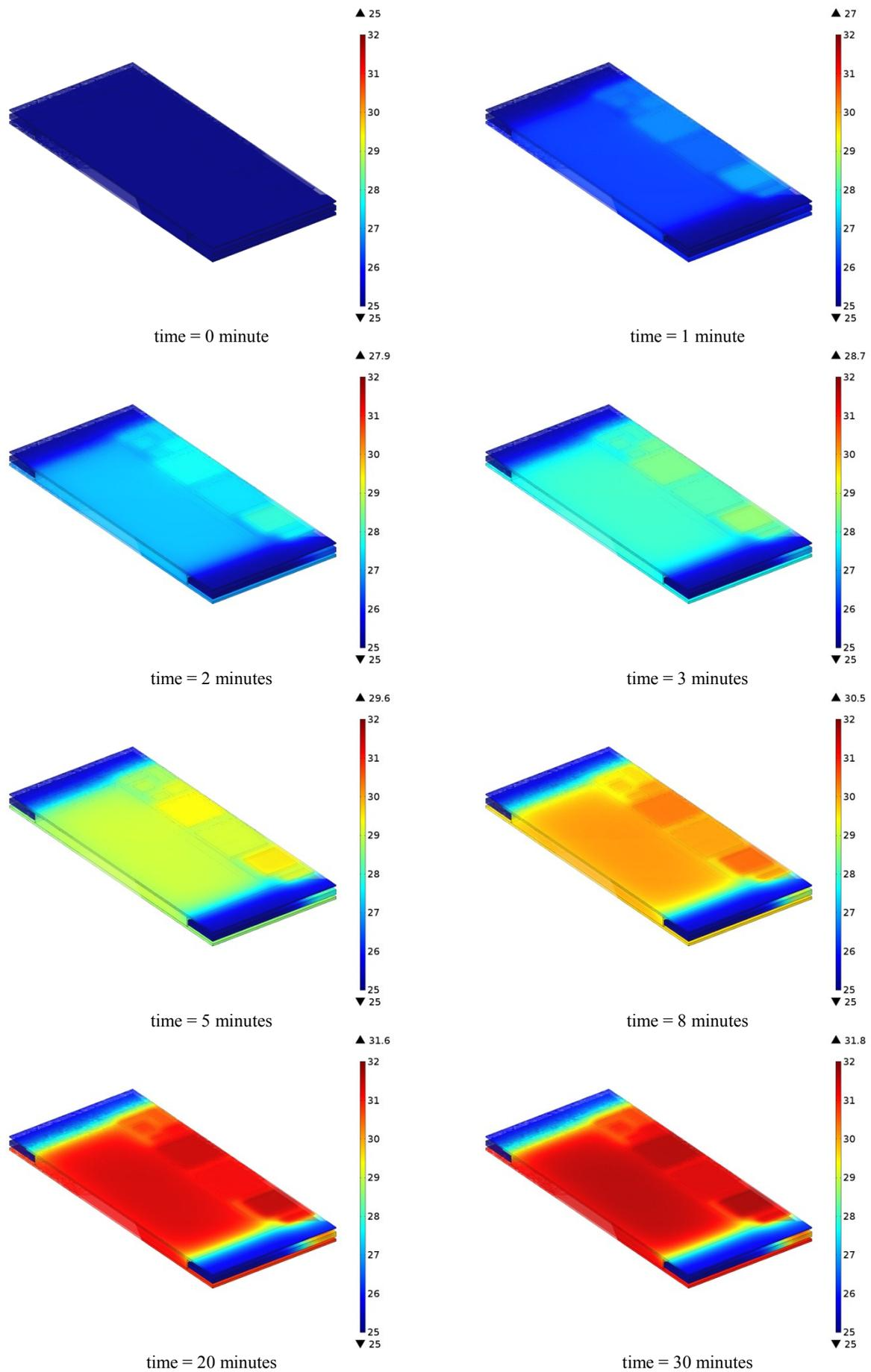
Figure 6. Temperature distribution in iPhone5 [°C] during operating from 0 ~ 30 minutes.
