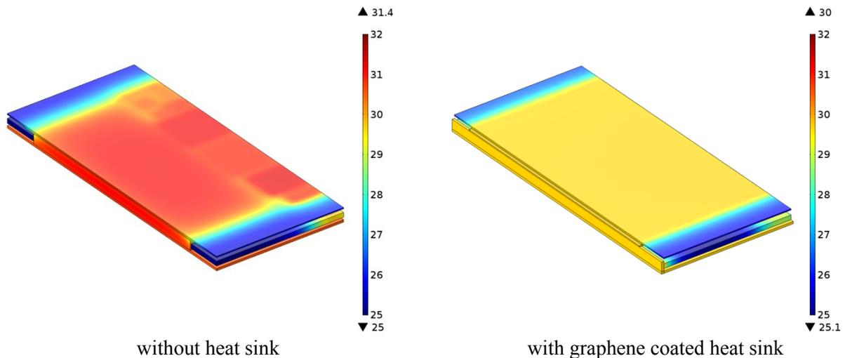
Figure 9. Temperature distribution in iPhone5 [°C] during operating for 15 minutes without and with graphene coated copper flat plate heat sink.
