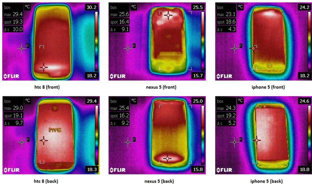
Figure 2. Thermal camera images from video test for 15 minutes of three different types of smartphones.
