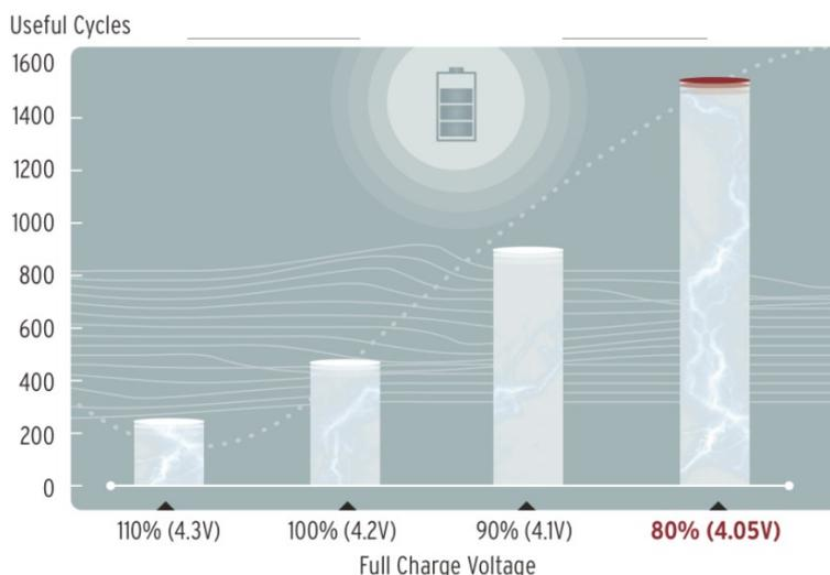
Figure 5. Useful cycles and charge voltage interaction as represented by [26].
