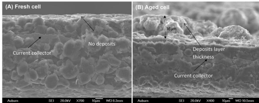
Figure 4. Deposit layer concentration taken by an aged anode electrode after 600 battery cycles as shown at [22].
