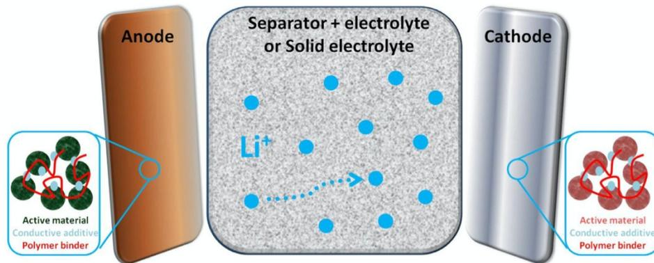
Figure 2. Lithium Polymer battery structure, by Costa et al. [10]
