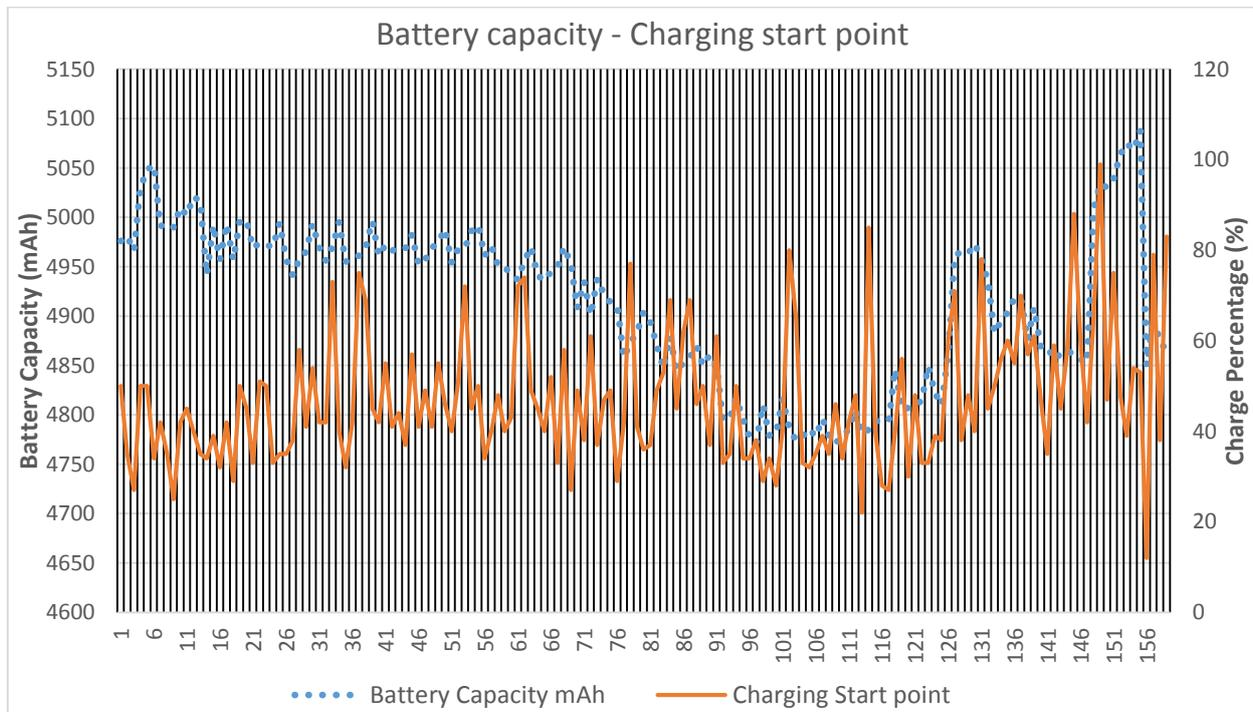
Figure 11. The effect partial discharges have on battery capacity.
