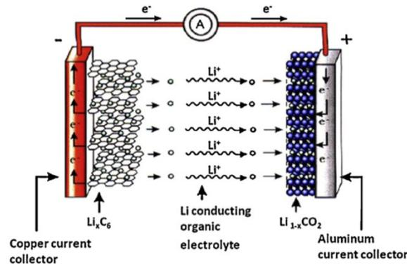
Figure 1. A typical ion battery as reproduced by Scrosati, B. and Garche, J. (2010) [3].
