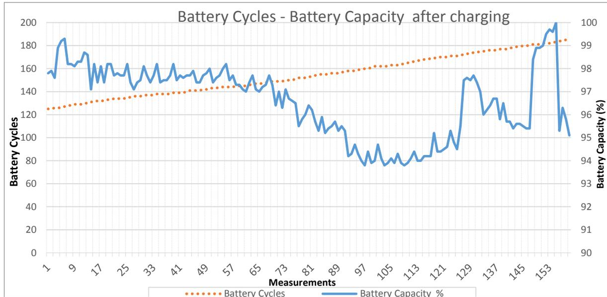
Figure 7. Battery capacity after charging to battery cycles comparison. Cycles follow a linear increase as expected whereas capacity ranges substantially.
