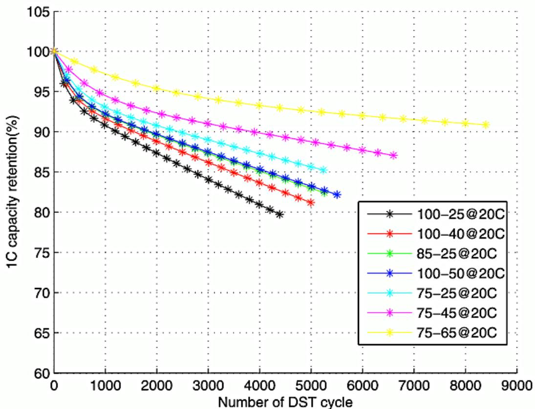
Figure 12. Reproduced Dynamic Stress test data comparison by Xu et al. [29]. This graph confirms the DoD technique declared at precious chapters.
