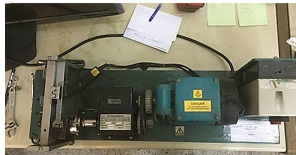
(b) Alternating-bending fatigue testing machine
