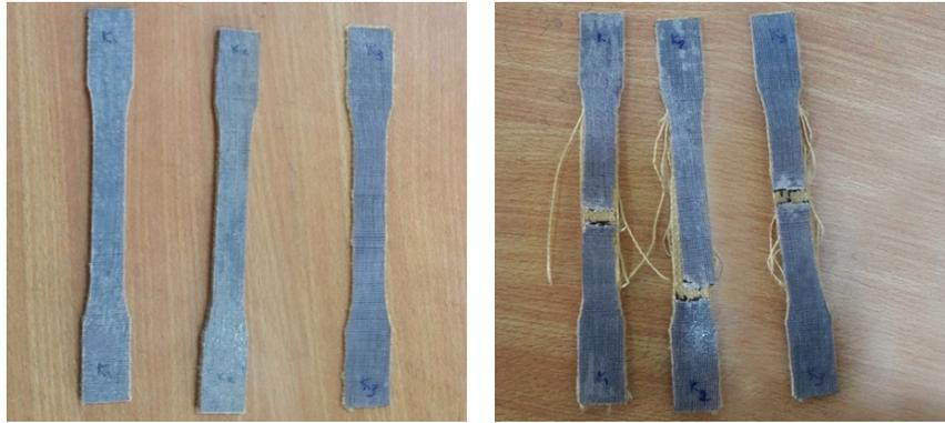
Figure 4. Tensile samples before and after test respectively.
