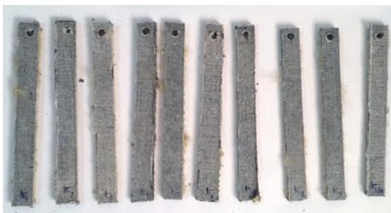
(c) Fatigue sample before test
