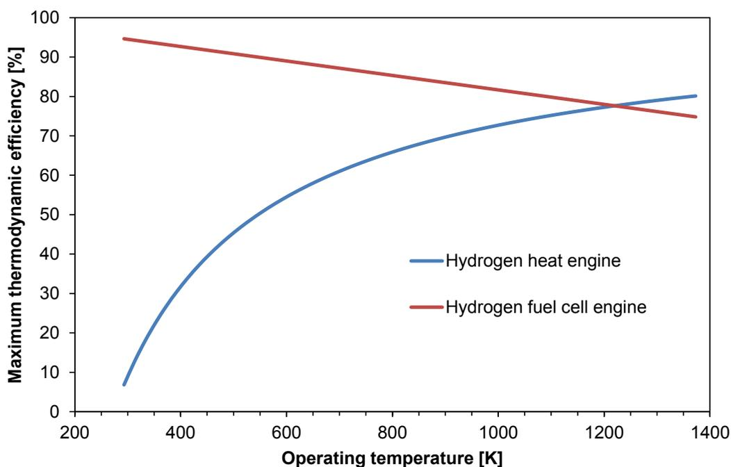
Figure 10. Comparison of maximum thermodynamic efficiency for hydrogen heat engine (Carnot cycle, exhaust to 273 K) and hydrogen fuel cell engine (vapour-phase water, LHV).
