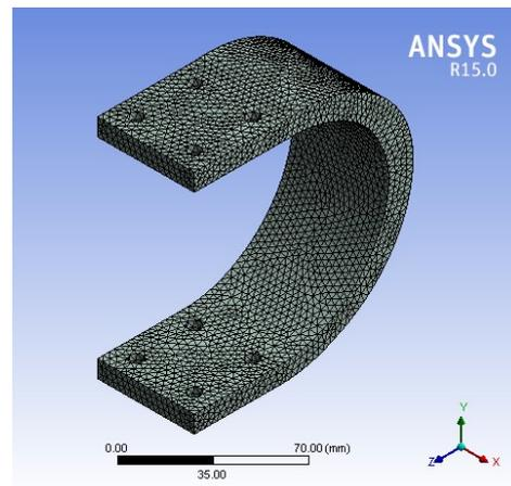
Figure 5. Meshing of model.
