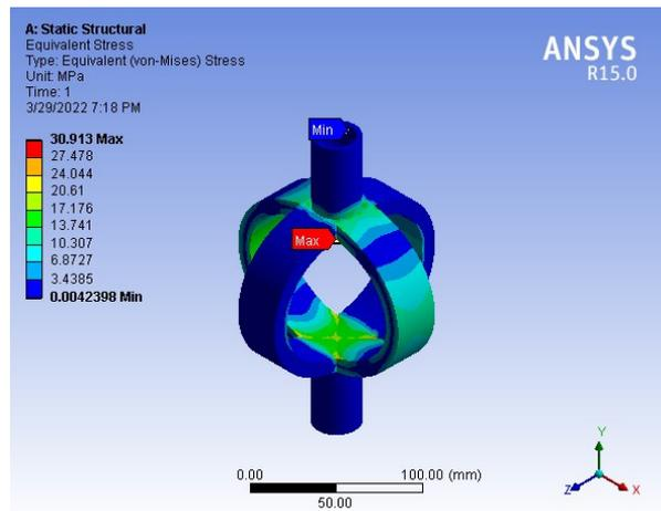
Figure 15. Equivalent Von-Mises stress for double circle model.
