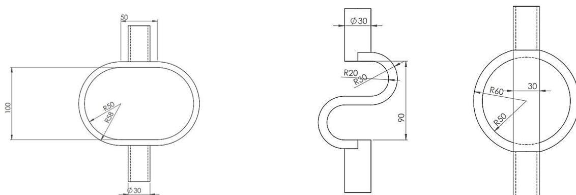
Figure 2. Detailed drawing of the suggested models.
