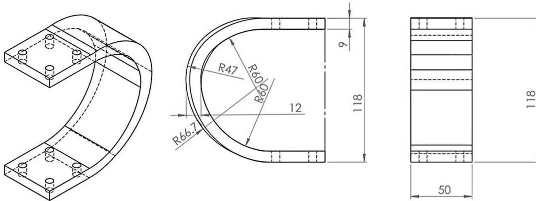
Figure 3. Isometric drawing of C shape used in SOLIDWORKS.
