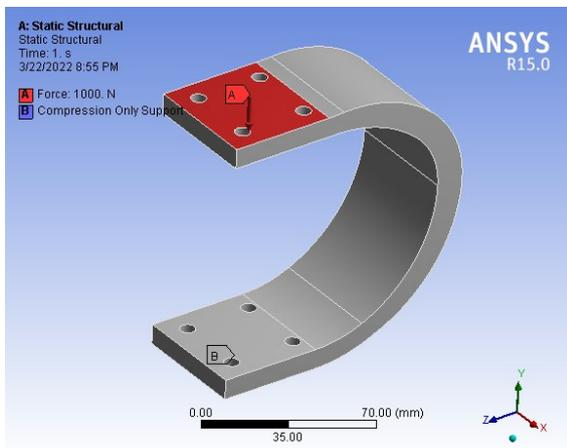
Figure 4. Load location and support.
