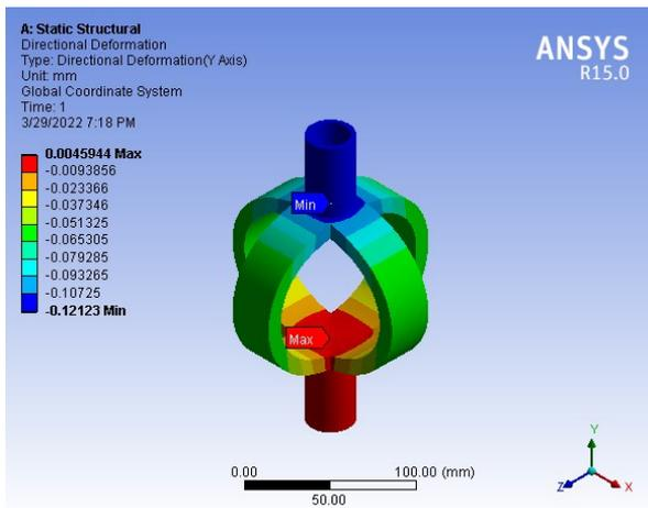
Figure 14. Deformation in Y-axis for double circle model.
