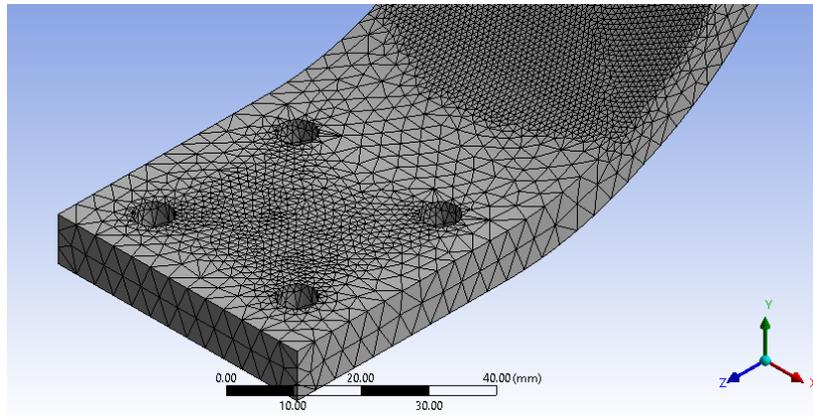
Figure 7. Mesh type, mesh sizing.
