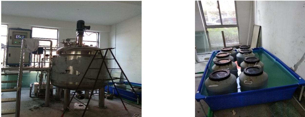
Figure 1. The pilot-scale digester setup with manure cold storage basin at the right hand side.
