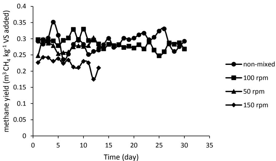
Figure 4. Methane yield for the different mixing intensities.
