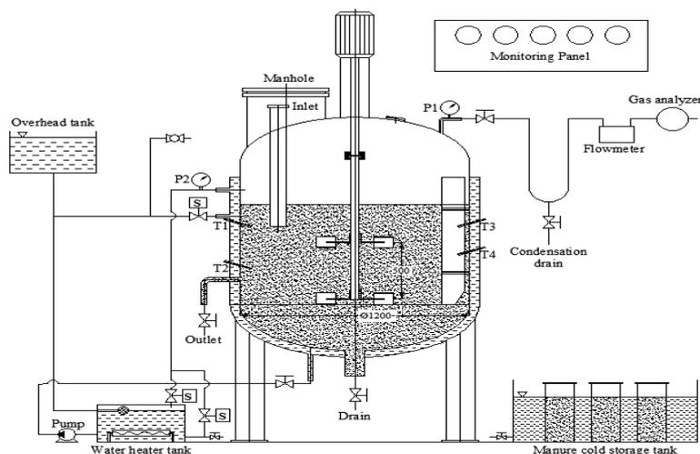
Figure 2. The 2D sketch of the pilot-scale stirred tank digester setup.
