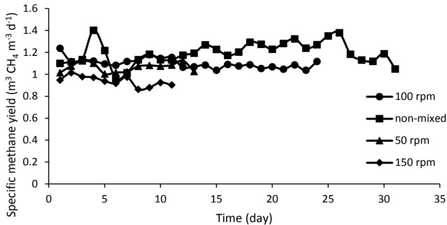
Figure 3. Specific methane production rate at different mixing intensities.
