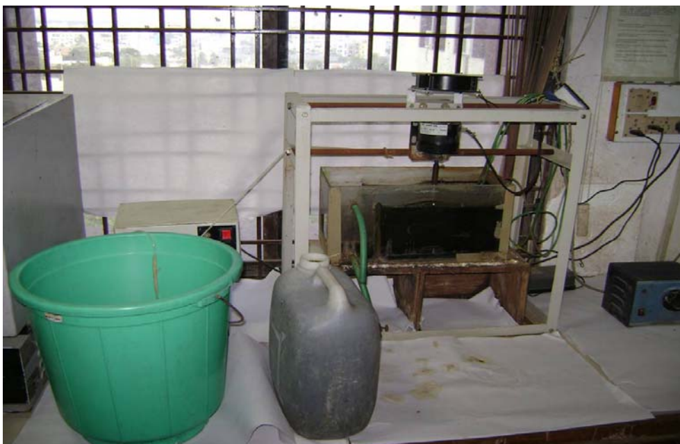
Figure 1. Activated sludge reactor used for the degradation phenolic compounds
