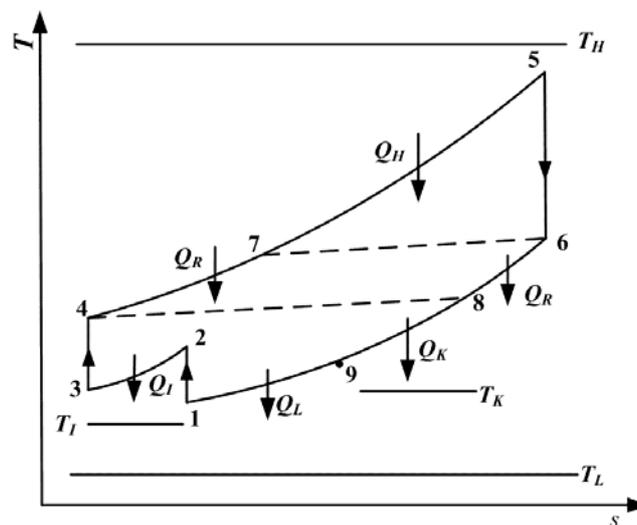
Figure 1.  $T$ - $s$  diagram for the cycle model
