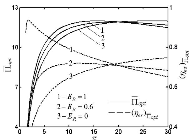
Figure 6. Effects of  $E_R$  on the characteristics of  $\bar{\Pi}_{opt}$  and  $(\eta_{ex})_{\bar{\Pi}_{opt}}$  versus  $\pi$
