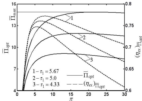
Figure 4. Effects of  $\tau_1$  on the characteristics of  $\bar{\Pi}_{opt}$  and  $(\eta_{ex})_{\bar{\Pi}_{opt}}$  versus  $\pi$
