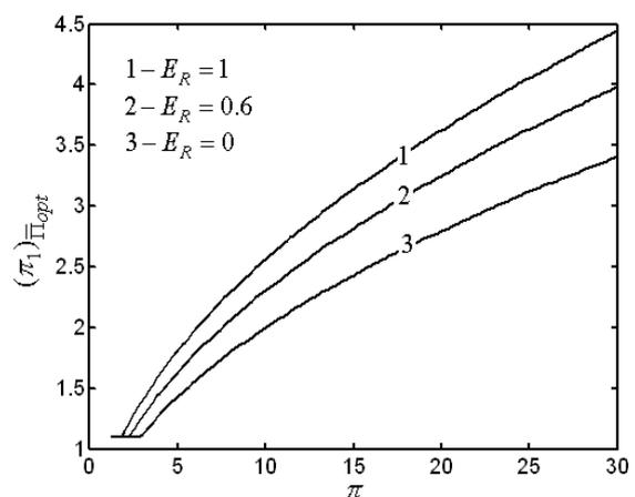
Figure 7. Effect of  $E_R$  on the characteristic of  $(\pi_1)_{\bar{\Pi}_{opt}}$  versus  $\pi$
