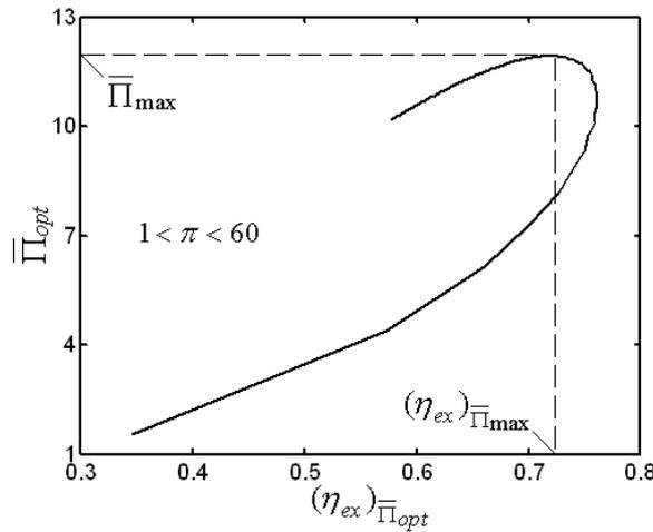
Figure 8. Characteristic of  $\bar{\Pi}_{opt}$  versus  $(\eta_{ex})_{\bar{\Pi}_{opt}}$
