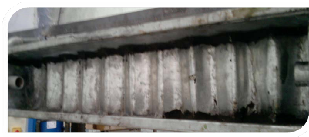
Figure 2. Corrugated channel in test section
