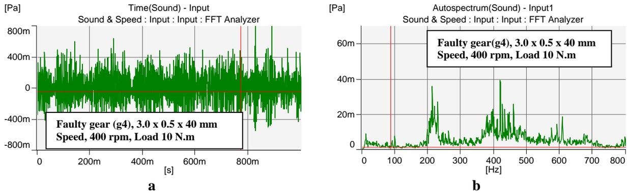
Figure 7. Sound pressure level spectra: (a) time history of sound pressure level; and (b) frequency domain of sound pressure level
