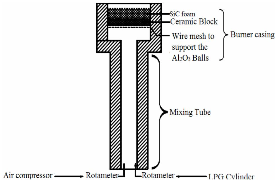
Figure 3. Schematic illustration of the PRB [12]
