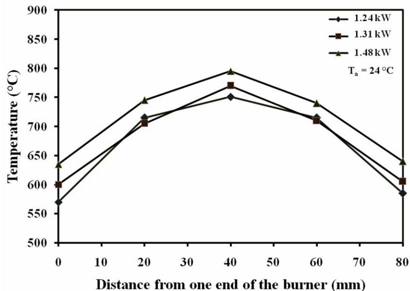
Figure 8. Temperature distribution on the burner surface of the porous matrix
