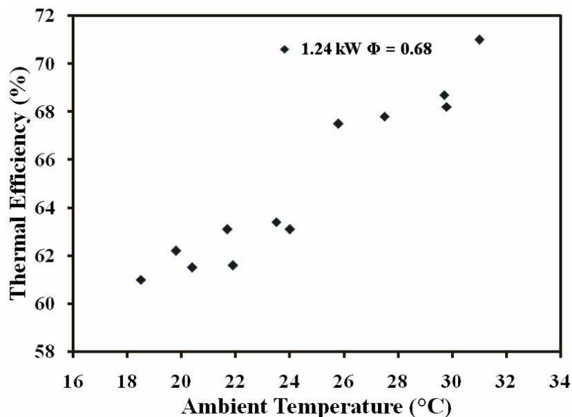
Figure 6. Effect of ambient temperature on the thermal efficiency of PRB
