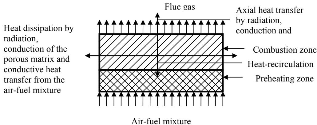
Figure 1. Illustration of combustion occurring in porous radiant burner
