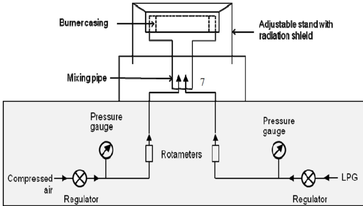
Figure 2. Layout of the experimental setup [12]
