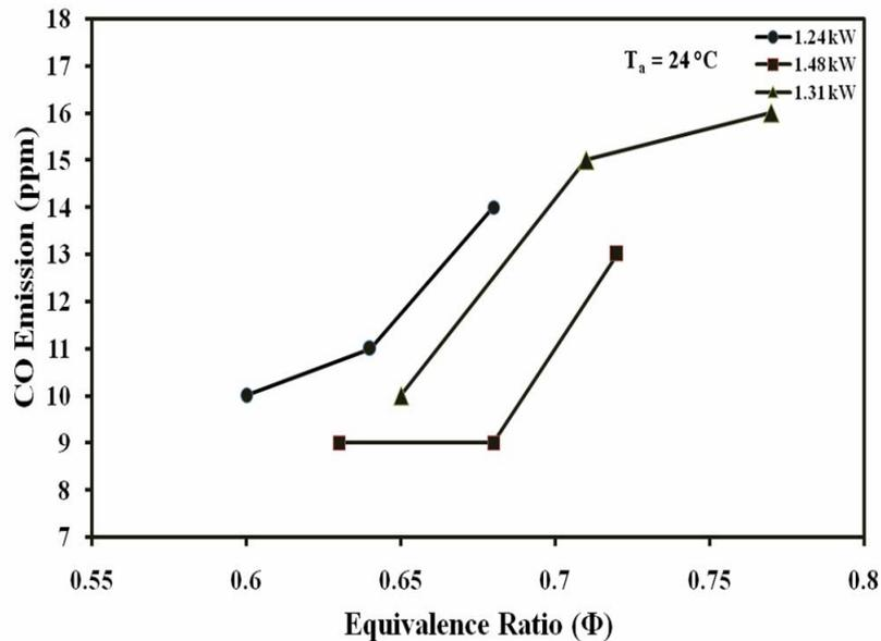
Figure 7. CO Emissions at different equivalence ratio and power intensities
