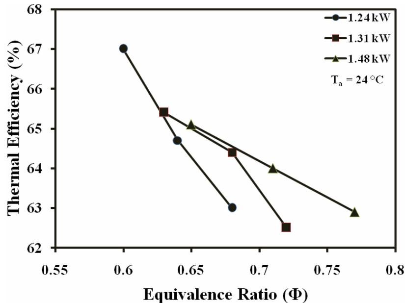
Figure 5. Effects of equivalence ratio and power intensity on thermal efficiency
