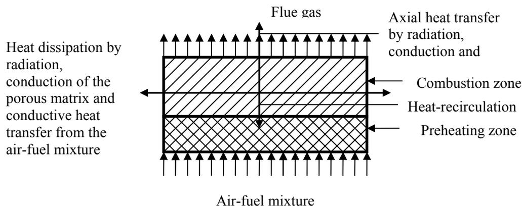
Figure 1. Illustration of combustion occurring in porous radiant burner
