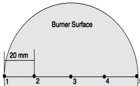
Figure 4. Position of thermocouples on the surface of the PRB
