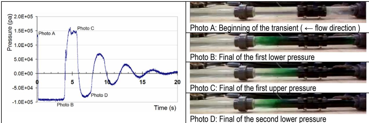
Figure 2. Experimental results of the tested transient scenario and images of the occurrence of intrusion
