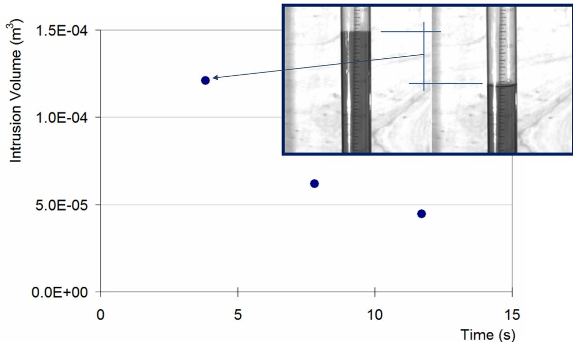
Figure 4. Experimental intrusion volume estimation by using the video of the transient
