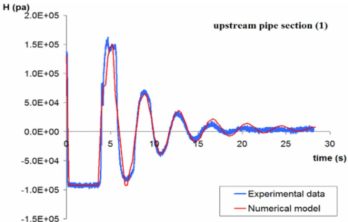
Figure 3. Comparison between MOC dissipative model results and experimental data
