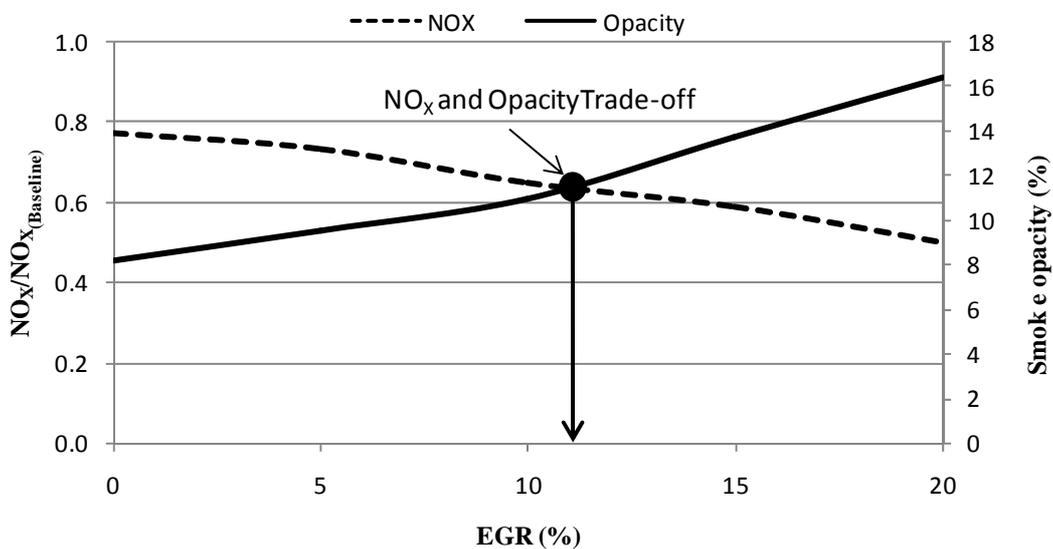
Figure 12. The optimum trade-off between NO<sub>x</sub> and smoke opacity for different EGR rates with JB5
