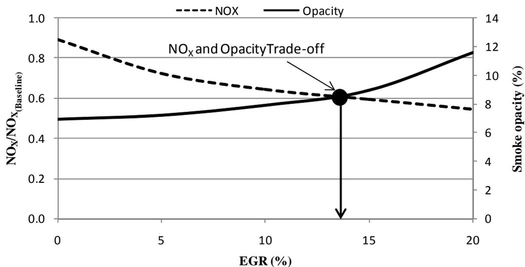
Figure 13. The optimum trade-off between NO<sub>x</sub> and smoke opacity for different EGR rates with JB20
