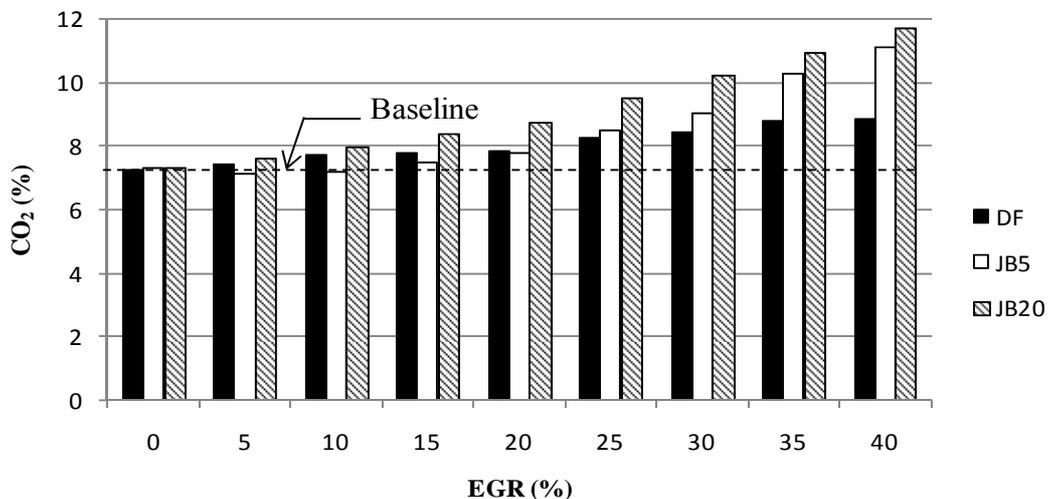
Figure 9. Variation of CO<sub>2</sub> emission with various EGR rates
