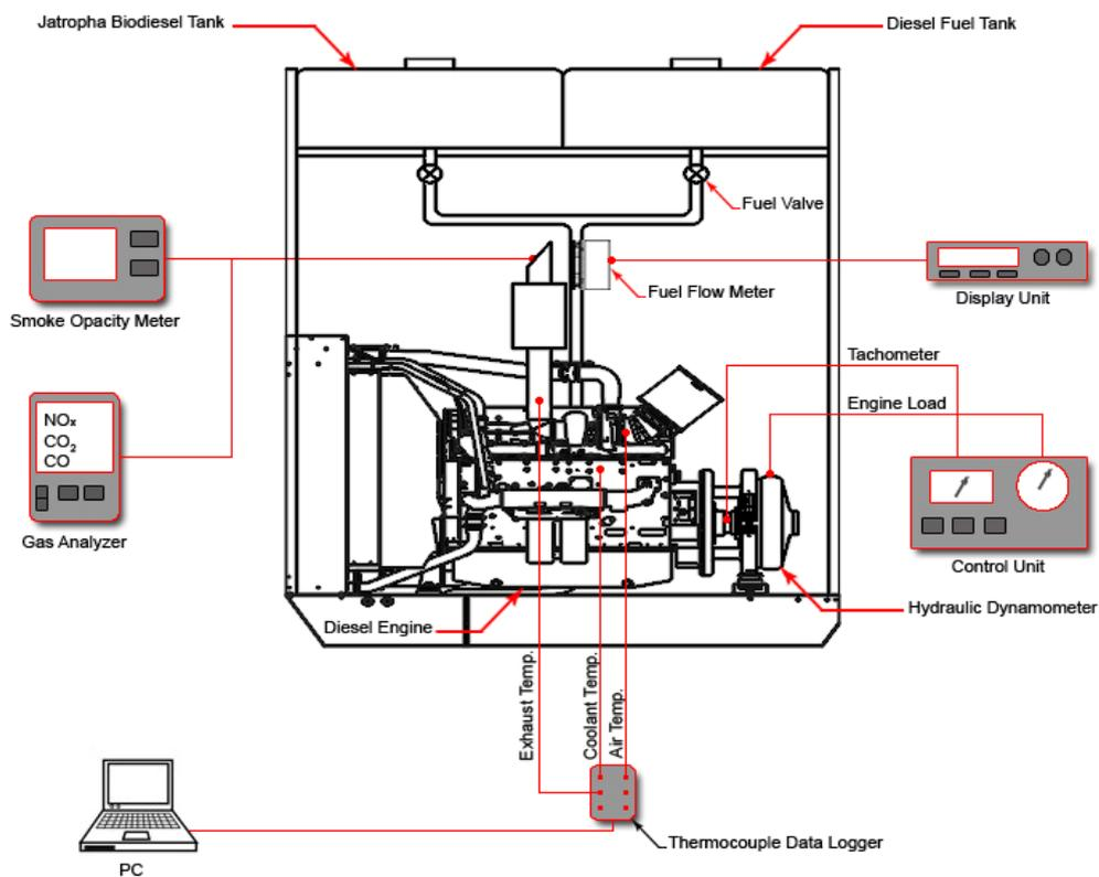
Figure 2. A schematic diagram of experimental setup
