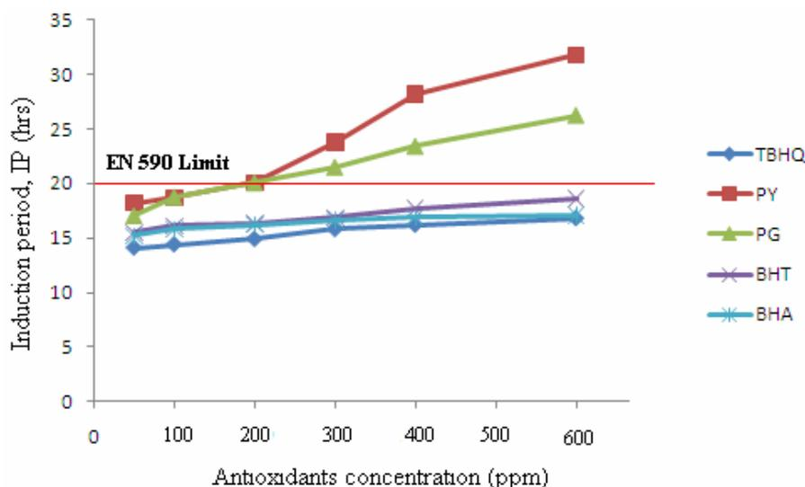
Figure 9. Effect of antioxidants on the stability of B40 blend
