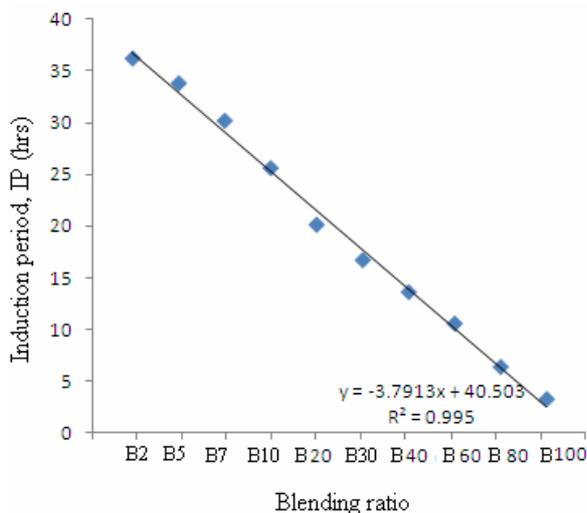
Figure 4. Variation of induction period with blending ratio
