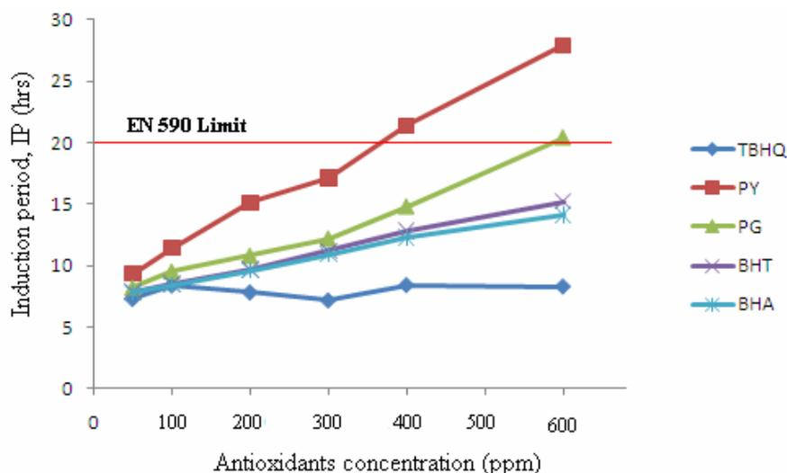
Figure 7. Effect of antioxidants on the stability of B80 blend
