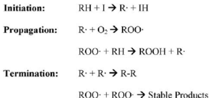
Figure 1. Primary oxidation reaction
