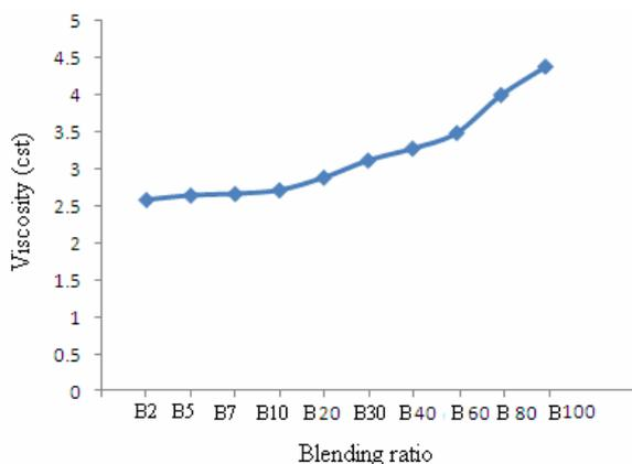
Figure 6. Variation of viscosity with in increasing proportion of blend
