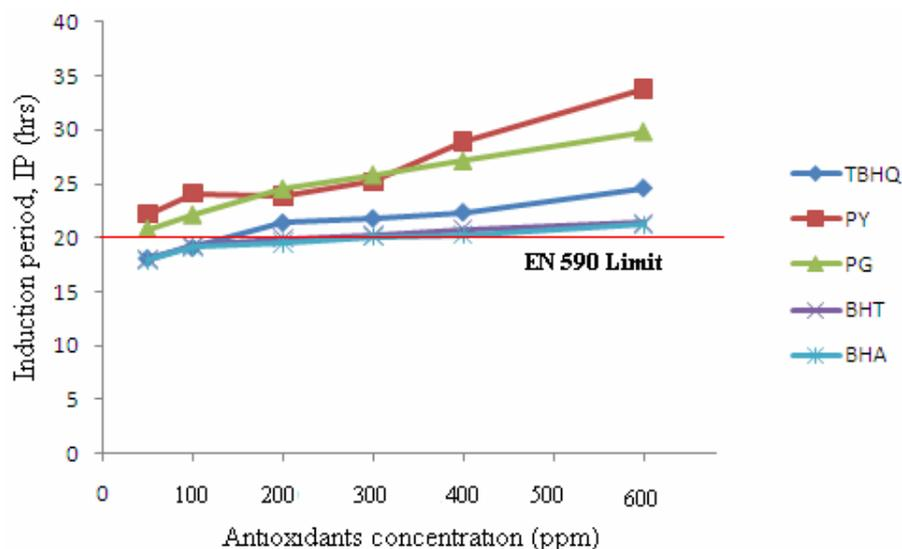
Figure 10. Effect of antioxidants on the stability of B30 blend
