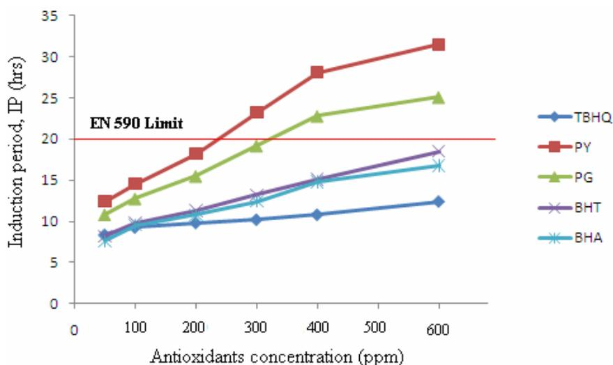
Figure 8. Effect of antioxidants on the stability of B50 blend
