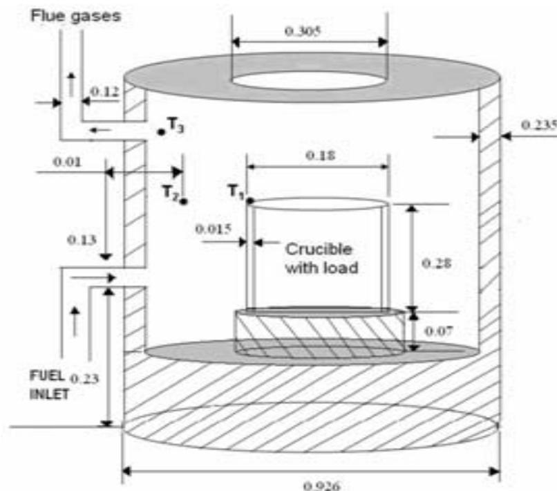
Figure 1. Schematic diagram of the crucible furnace for model geometry (in metre)
