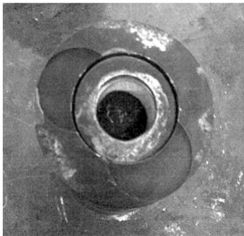
Figure 1. Photographic view of piston with porous medium implementation
