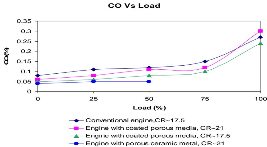
Figure 6. Comparison of carbon monoxide emission
