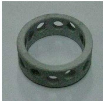
Figure 2. Zirconium dioxide ceramic coated porous medium
