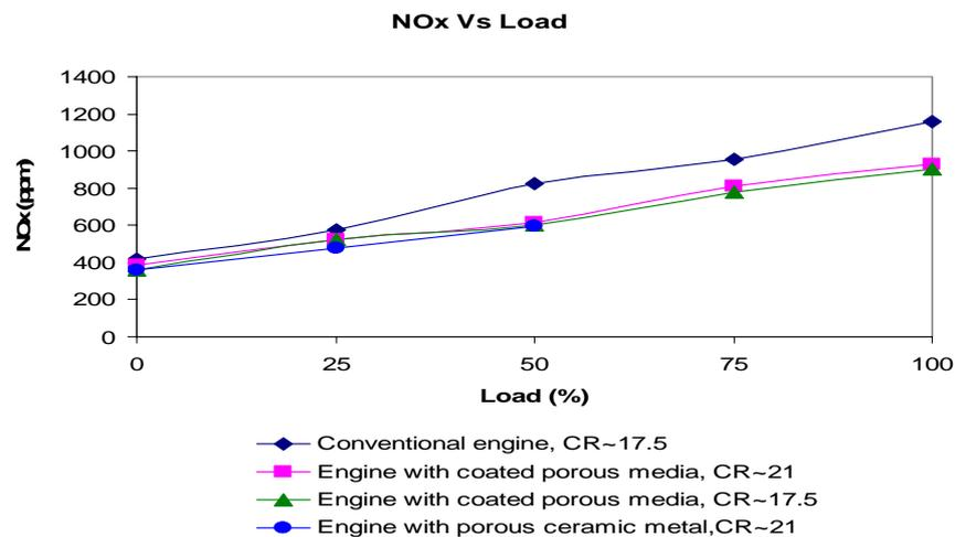
Figure 7. Comparison of nitrogen oxide emission
