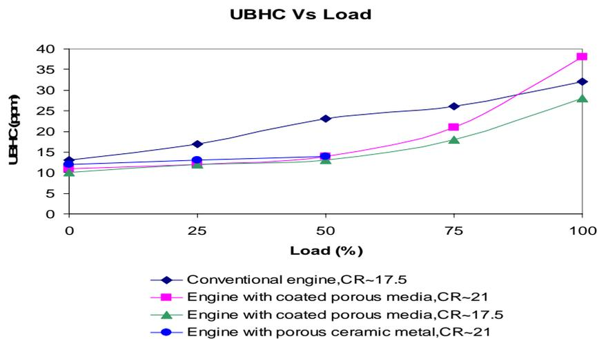
Figure 5. Comparison of hydrocarbon emission
