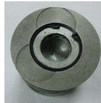
Figure 3. Assembled view of piston with zirconium dioxide coated porous medium
