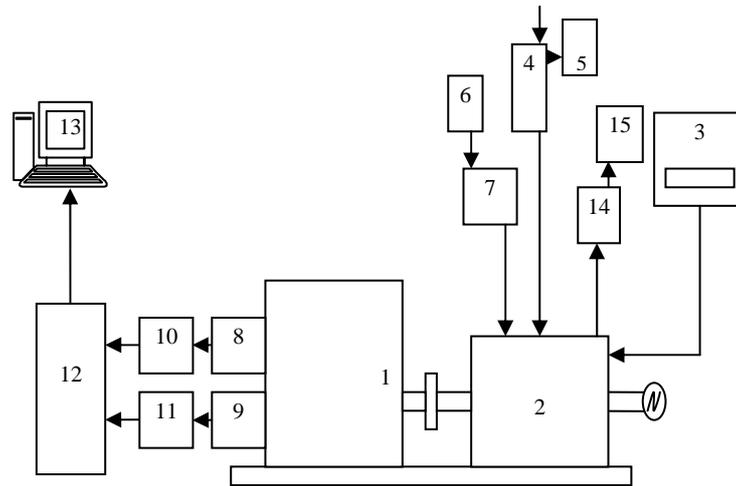
1- Diesel Engine, 2 - Electrical dynamometer, 3 - Dynamometer controls, 4 - Air box, 5 - U tube manometer, 6 - Fuel tank, 7 - Fuel measurement, 8 - Pressure transducer, 9 - TDC position sensor, 10 - Charge amplifier, 11- TDC amplifier circuit, 12 - Analog to digital card, 13 – Computer, 14 - Exhaust gas analyzer, 15 - AVL smoke meter
