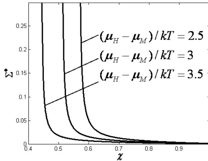
Figure 5. Influence of  $(\mu_H - \mu_M)/(kT)$  on  $\Sigma^*$  versus  $\chi$  characteristic with  $(\mu_O - \mu_L)/(kT) = 3$
