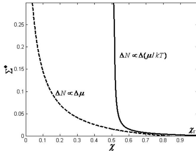
Figure 2. Relation between the optimal dimensionless rate of energy pumping and COP
