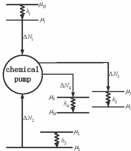
Figure 1. Model of an isothermal endoreversible four-mass-reservoir chemical pump
