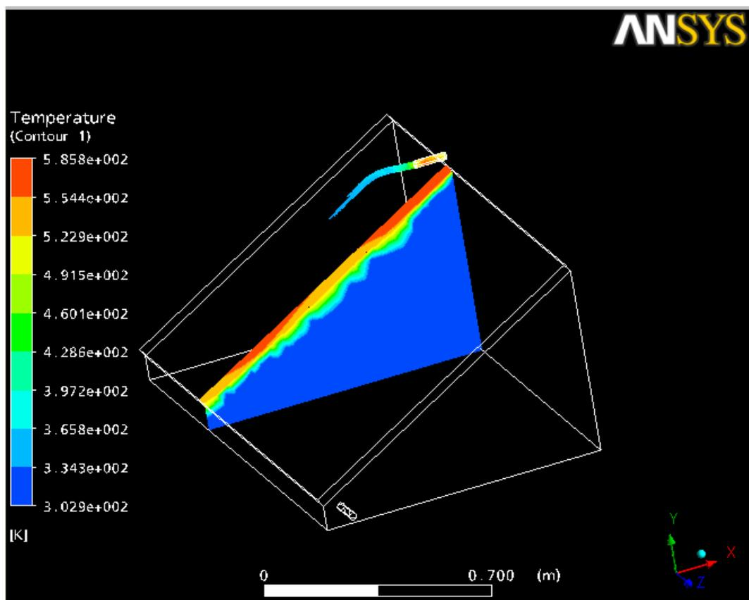
Figure 12. Side view of Temperature contour of solar still
