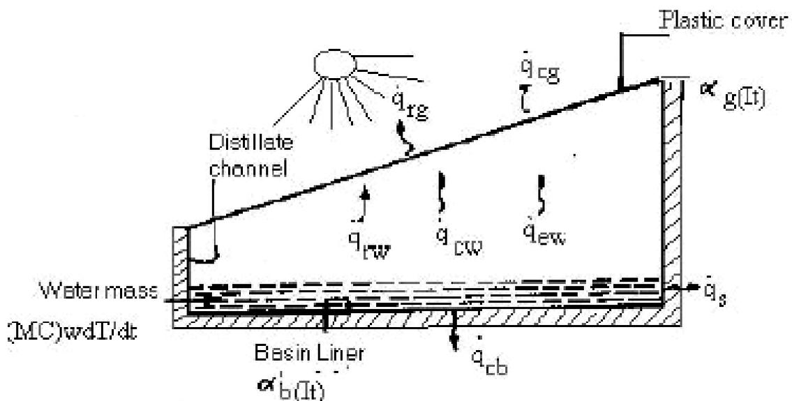
Figure 1. Energy flow in Single basin single slope solar still
