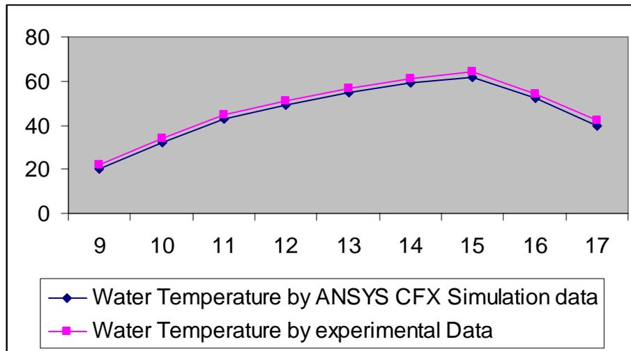
Figure 9. Water temperature predicted by ANSYS CFD Simulation and experimental data
