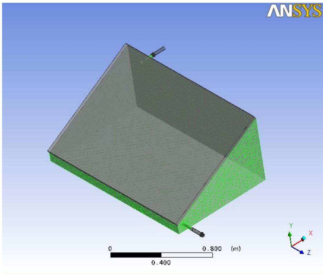
Figure 5. No slip wall boundary condition of solar still
