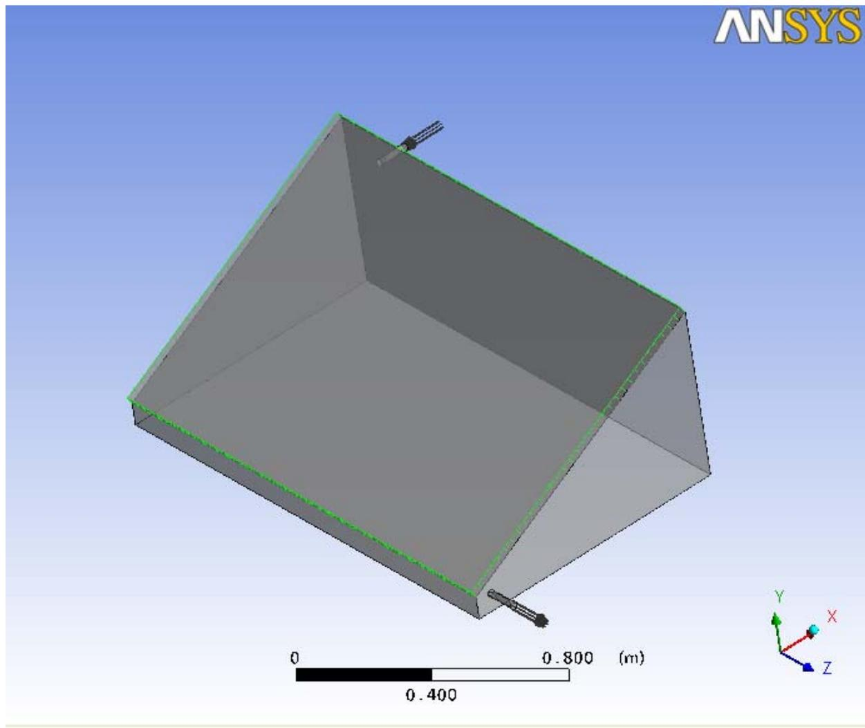
Figure 6. Adiabatic condition between glass and wall
