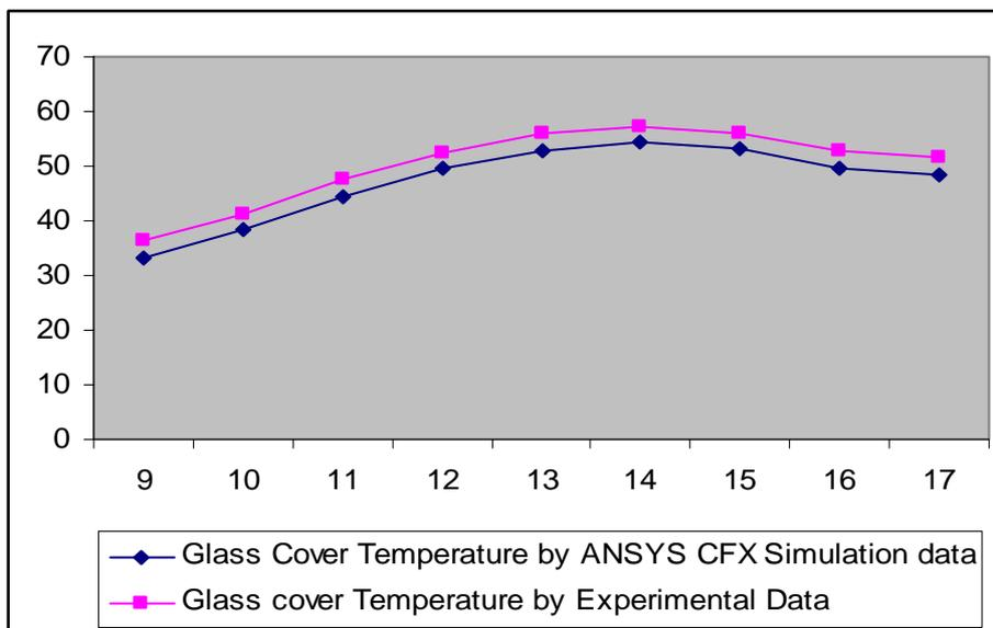
Figure 10. Glass cover Temperature predicted by ANSYS CFX Simulation result and experimental data
