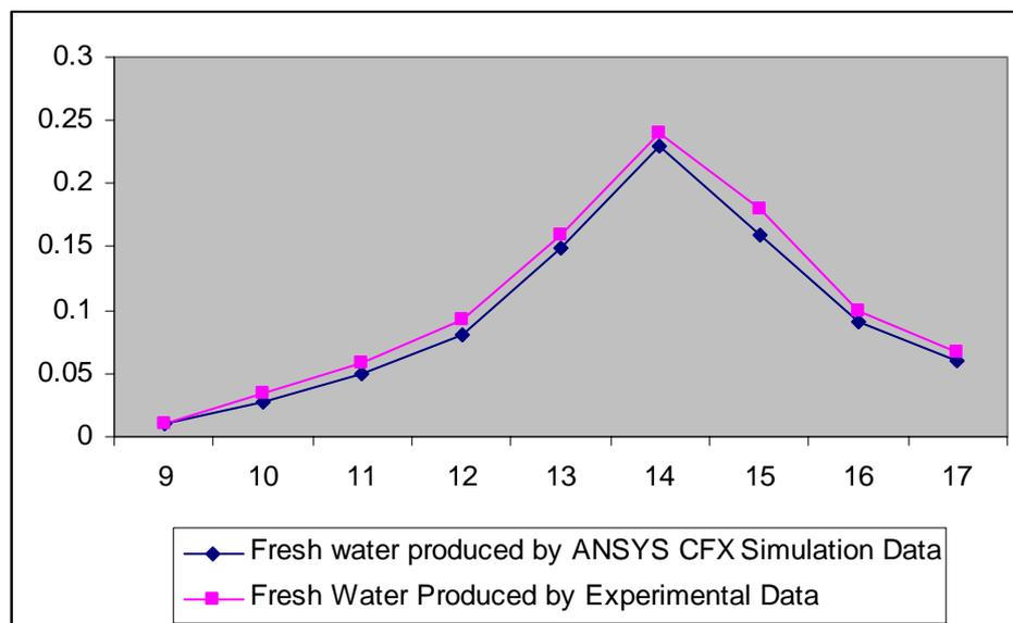
Figure 8. Rate of water production from experimental data and simulation results
