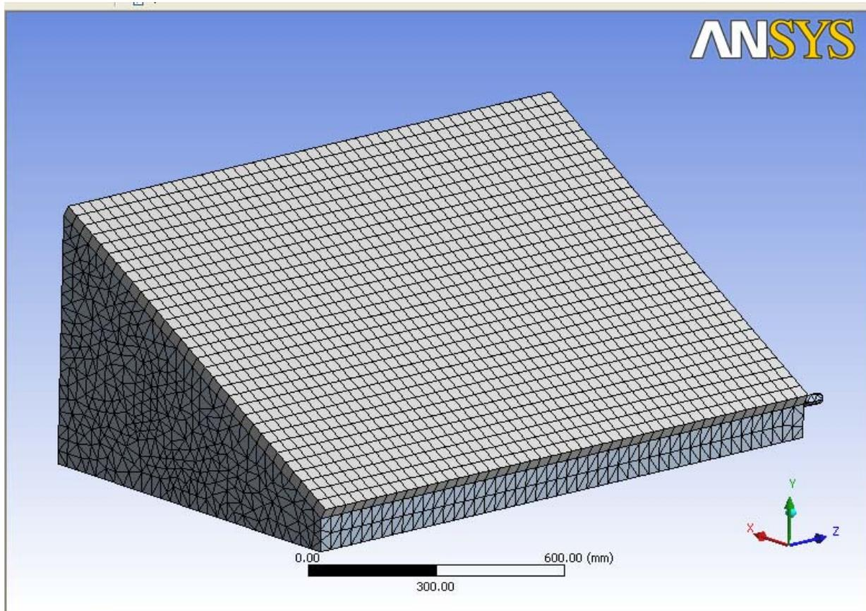
Figure 4. Meshing of model of Solar still in ANSYS
