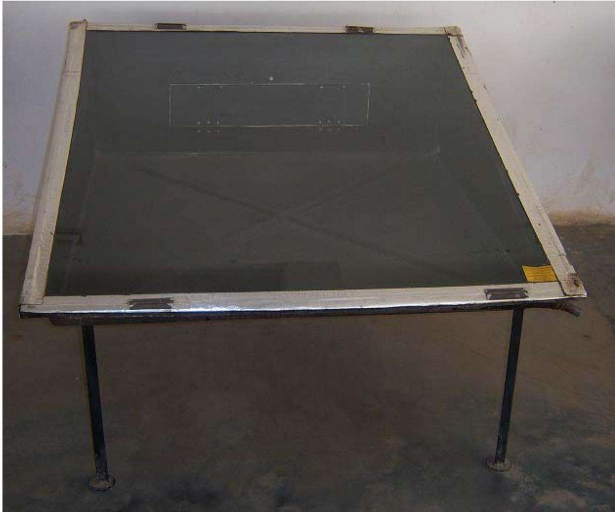
Figure 2. Experimental set up of solar still
