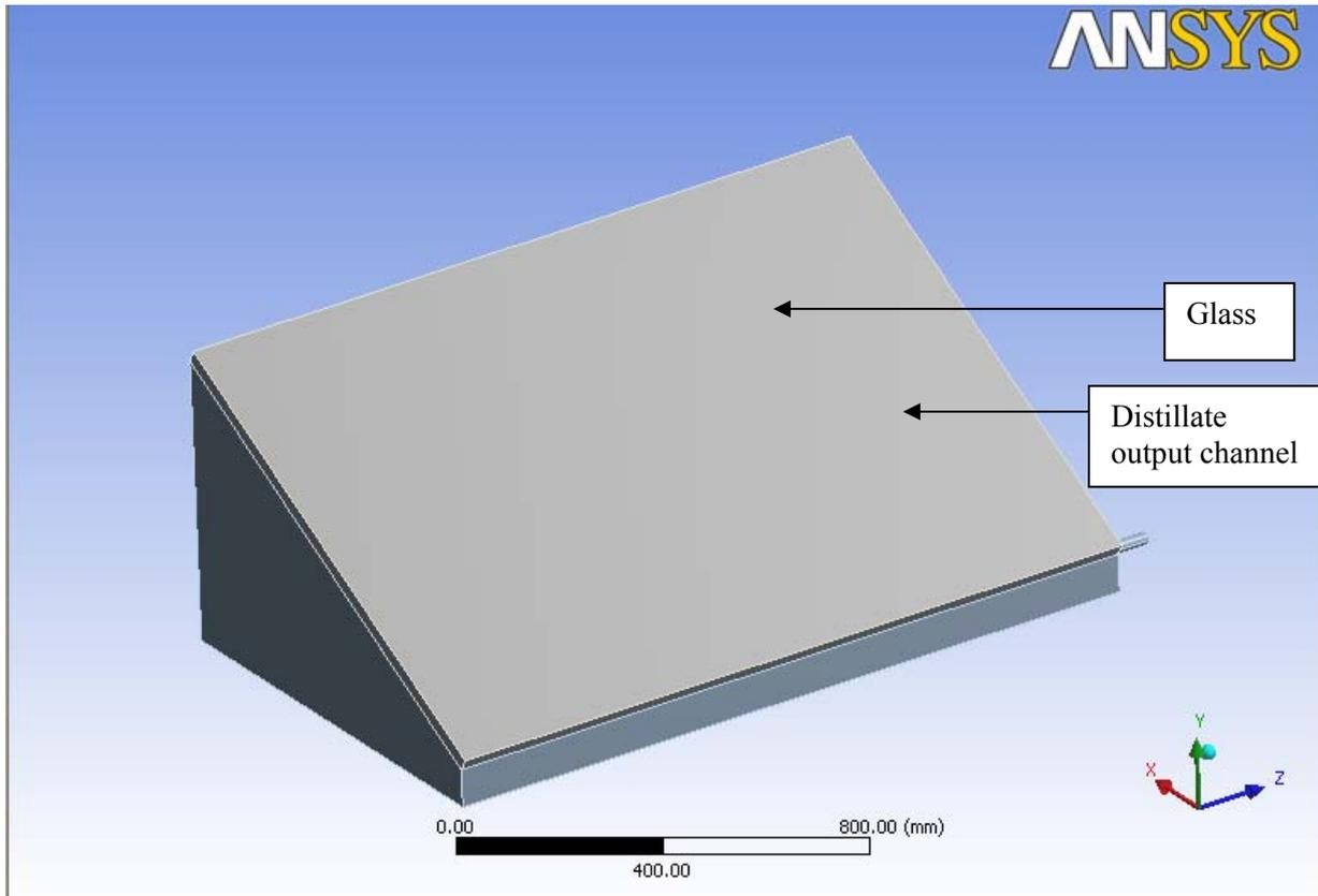
Figure 3. Model geometry of solar still made in ANSYS Workbench
