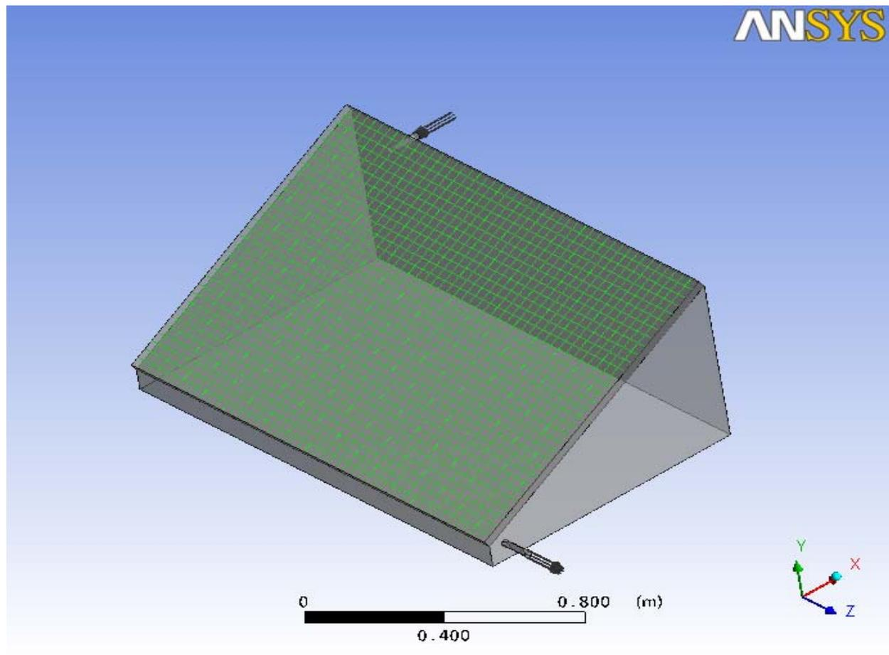
Figure 7. Application of Incident solar insolation applied to glass cover
