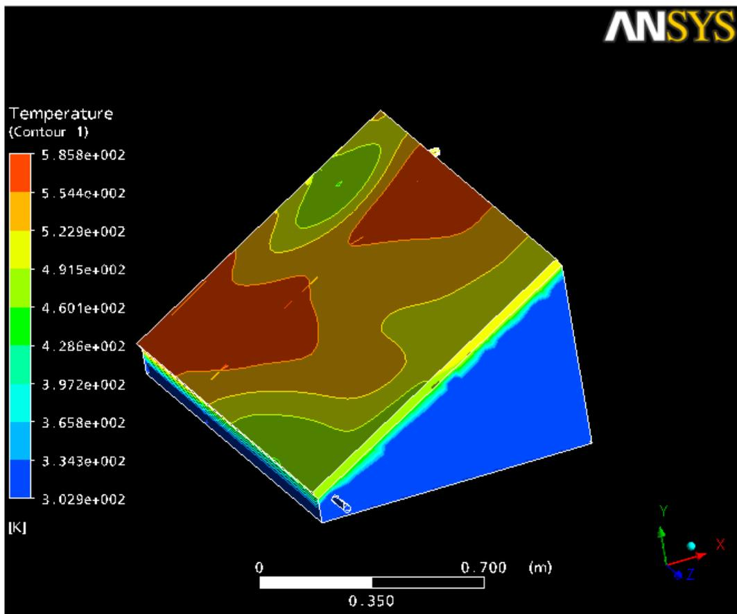
Figure 11. Temperature contour various points in solar still
