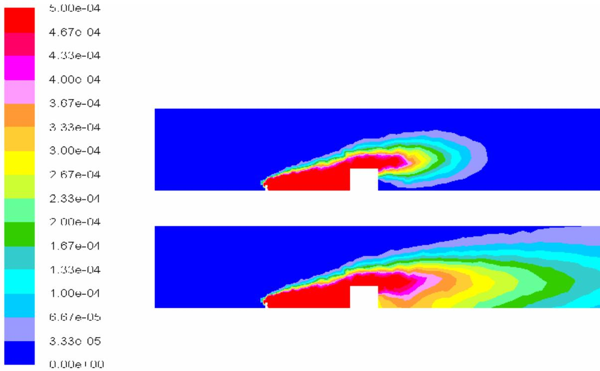
Figure 4. Mass fraction contour of Chlorine on the centre vertical plane at 30s and 90s
