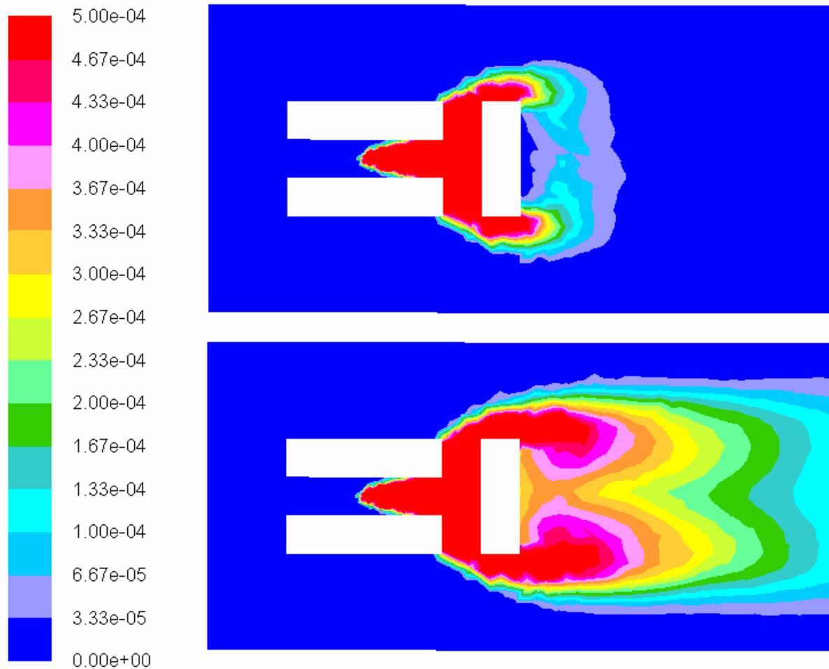
Figure 5. Mass fraction contour of Chlorine on the plane 1.5 m from the ground at 30s and 90s
