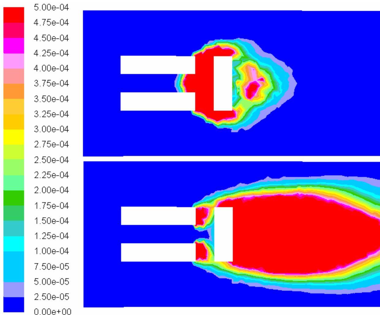
Figure 8. Mass fraction contour of Chlorine on the plane 1.5 m from the ground at 20s and 60s
