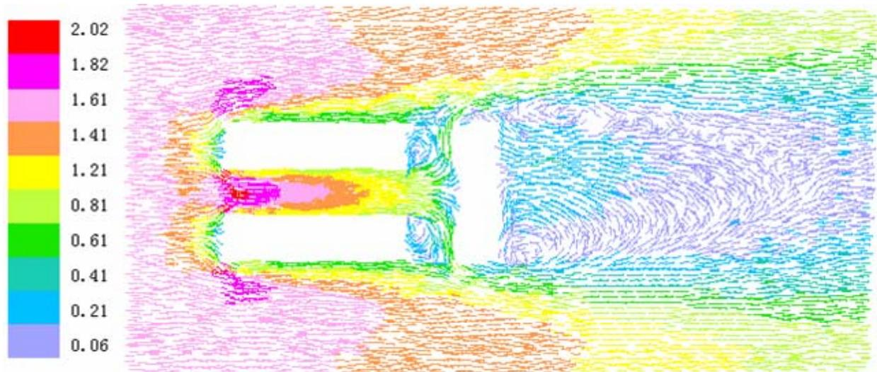
Figure 3. Velocity vector contour 1m from the ground (m/s)
