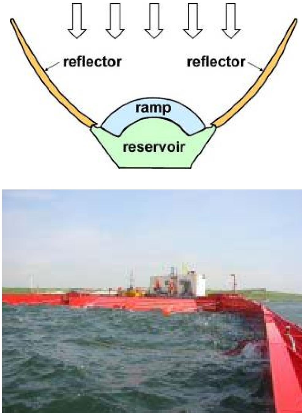
Figure 8. Photo and schematic representation of Wave Dragon [20]
