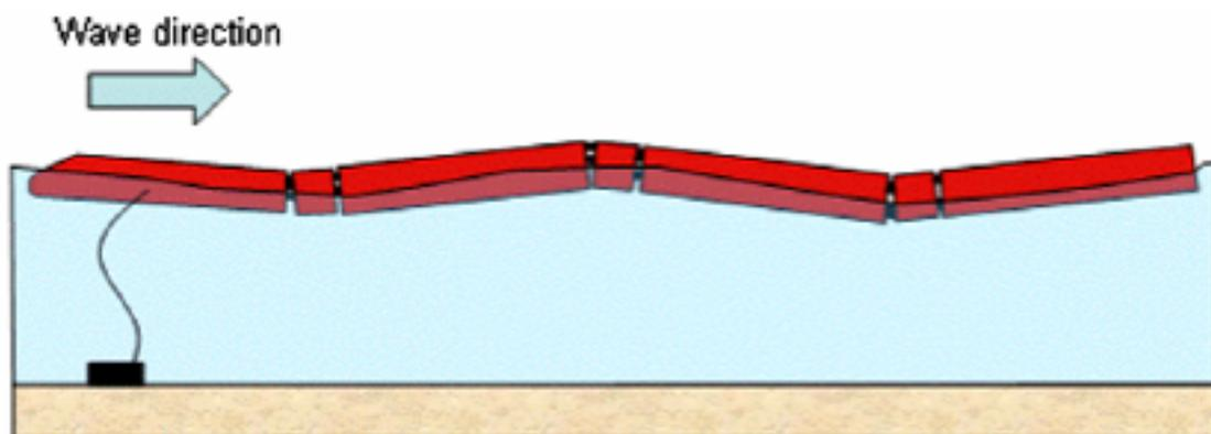
Figure 5. The four-unit of Pelamis wave farm [15]
