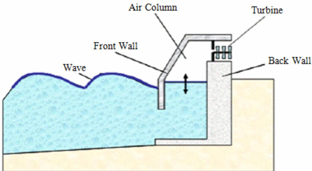
Figure 2. The oscillating water column [15]
