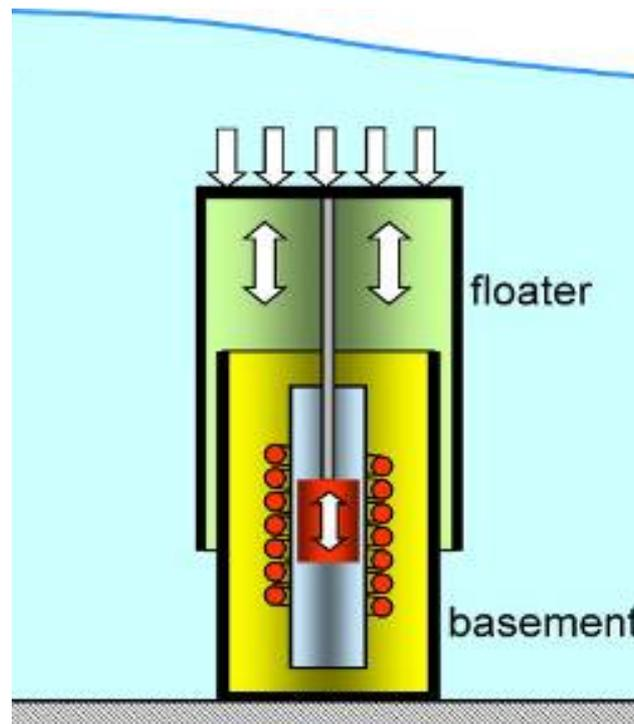
Figure 3. The Archimedes Wave Swing [16]
