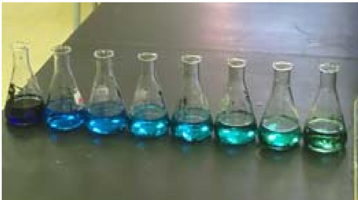
Figure 1. 50 ml aliquot of methylene blue after addition of different masses of adsorbent. The first flask on the left contains the original solution without addition of adsorbent
