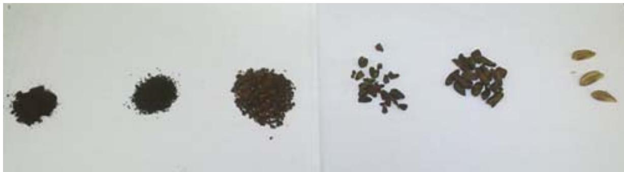
Figure 2. Different particle sizes of the dried dates stones. The three particles on the right are whole stones while on the left are powdered particles
