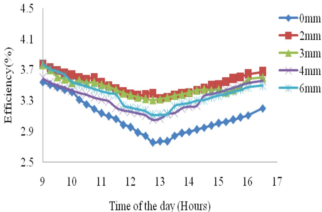
Figure 6. Variation of module efficiency throughout the day
