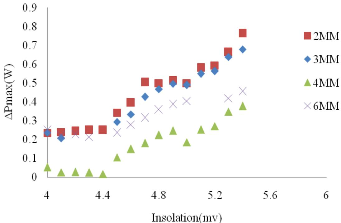
Figure 3. Variation of  $\Delta P_{\max}$  with solar radiation
