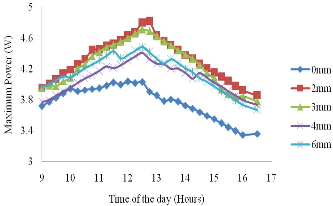
Figure 7. Variation of maximum power delivered by module throughout the day
