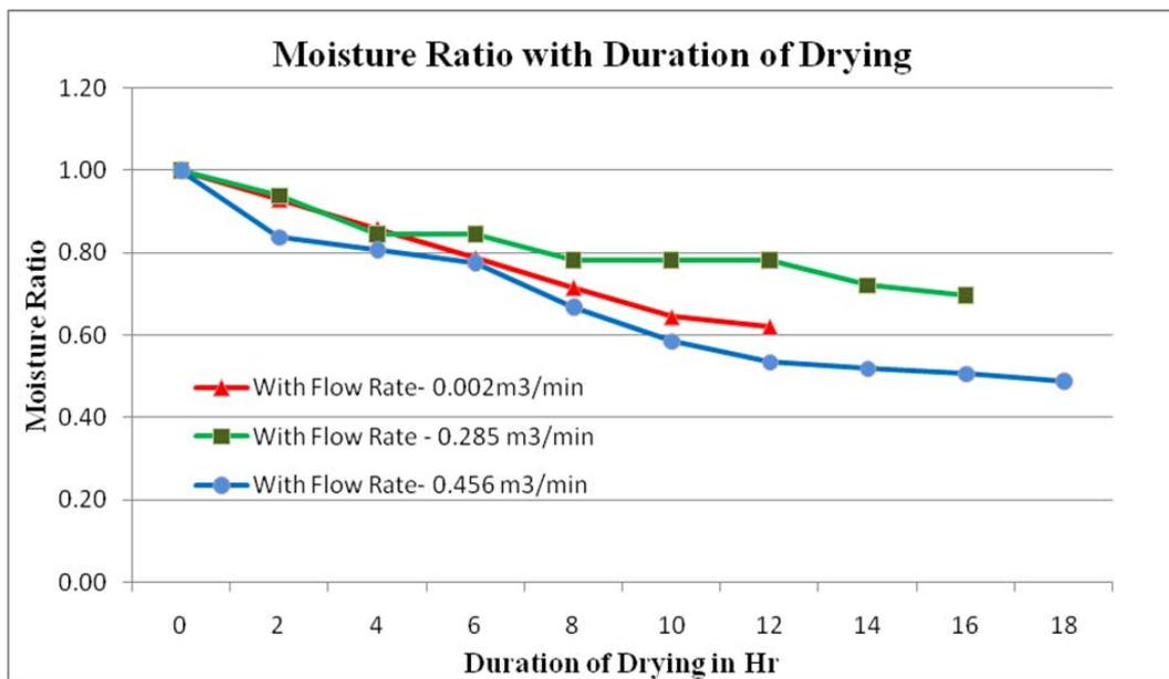
Figure 4. Variation of Moisture Ratio with Duration of drying for Tendu Leaf for different mass flow rates
