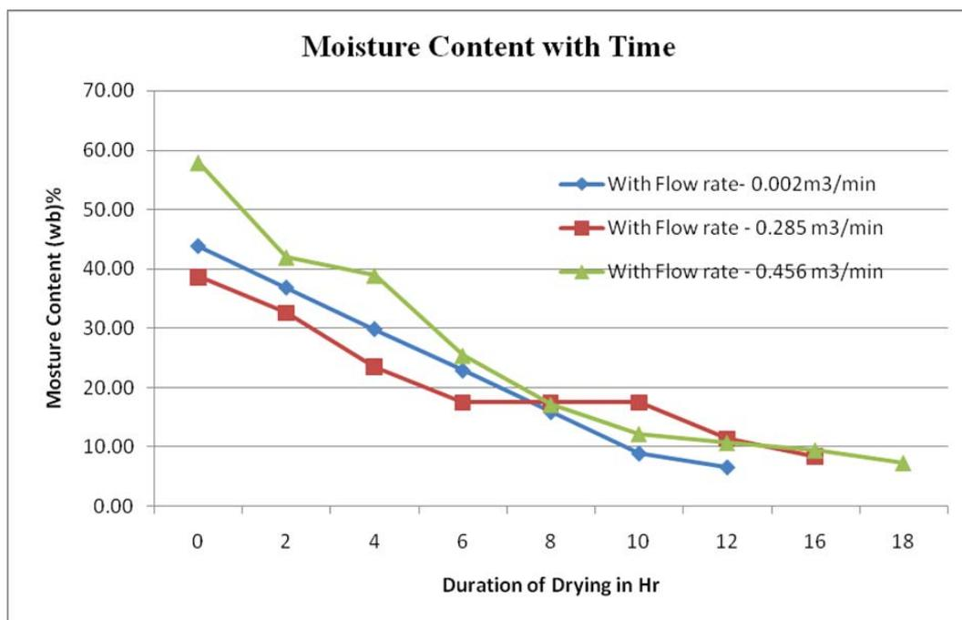
Figure 3. Variation of Moisture Content with Duration of drying for Tendu Leaf for different mass flow rates
