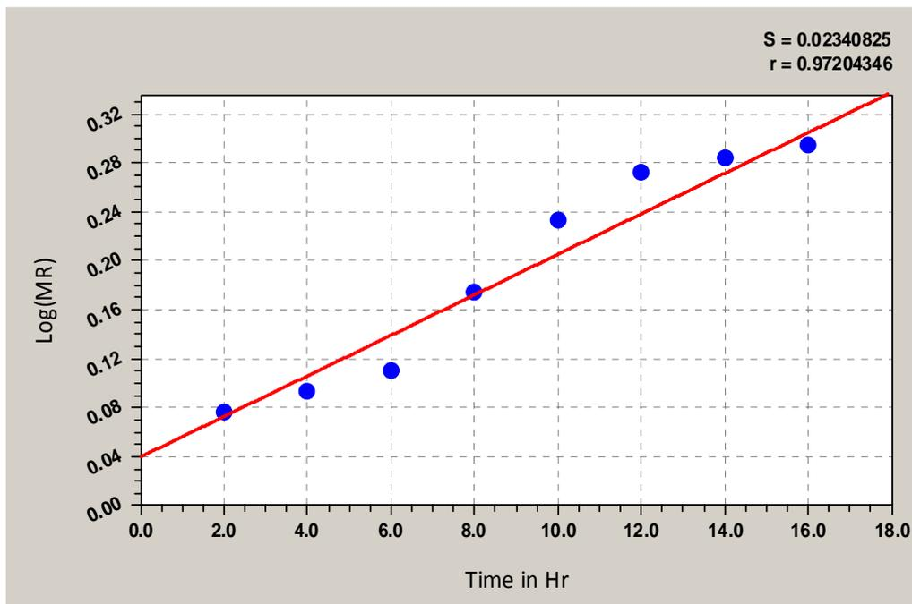
Figure 7. Log (MR) as a function of time for experiments of tendu leaves with mass flow rate of  $0.456 \text{ m}^3/\text{min}$  using solar dryer
