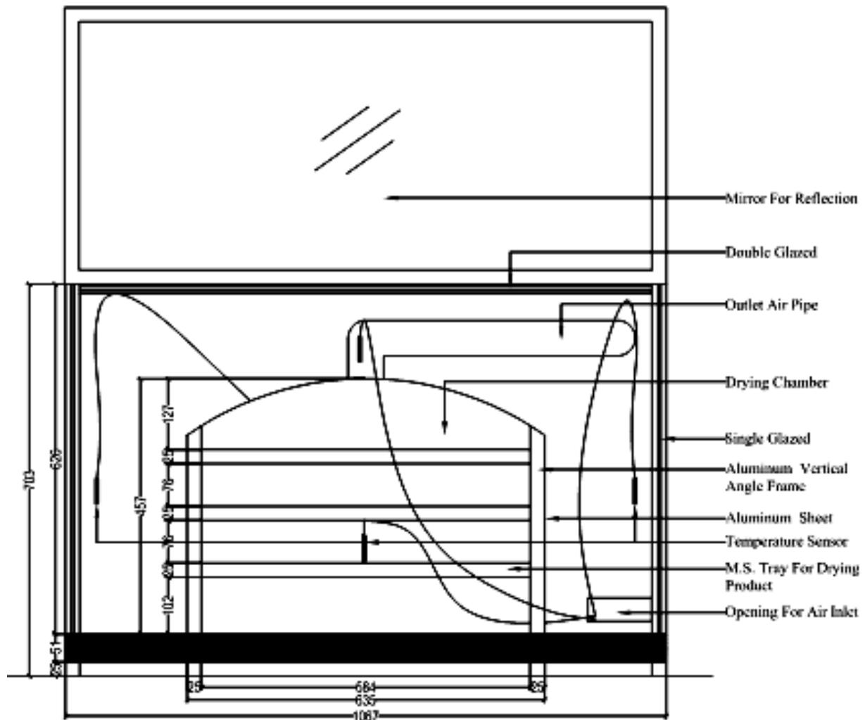
Figure 1. Front view of solar dryer with mirror booster
