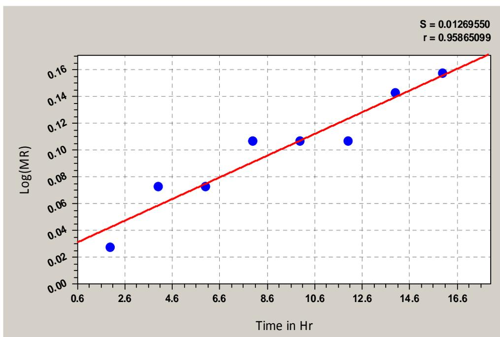
Figure 6. Log (MR) as a function of time for experiments of tendu leaves with mass flow rate of 0.285 m<sup>3</sup>/min using solar dryer
