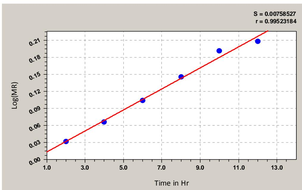
Figure 5. Log (MR) as a function of time for experiments of tendu leaves with mass flow rate of 0.002 m<sup>3</sup>/min (Natural Convection) using solar dryer
