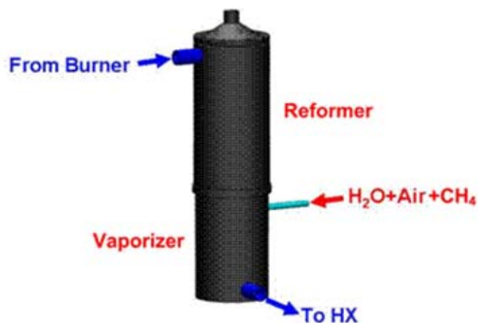
Figure 8. Non-electrically heated reformer
