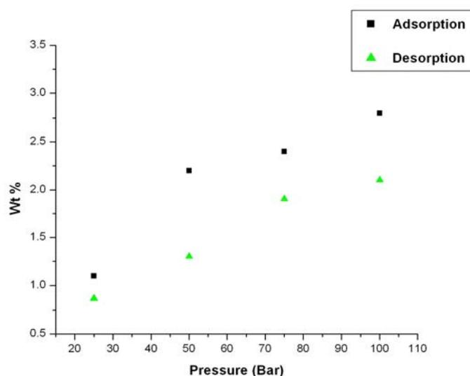
Figure 5. Adsorption and Desorption Isotherm of MOF-177
