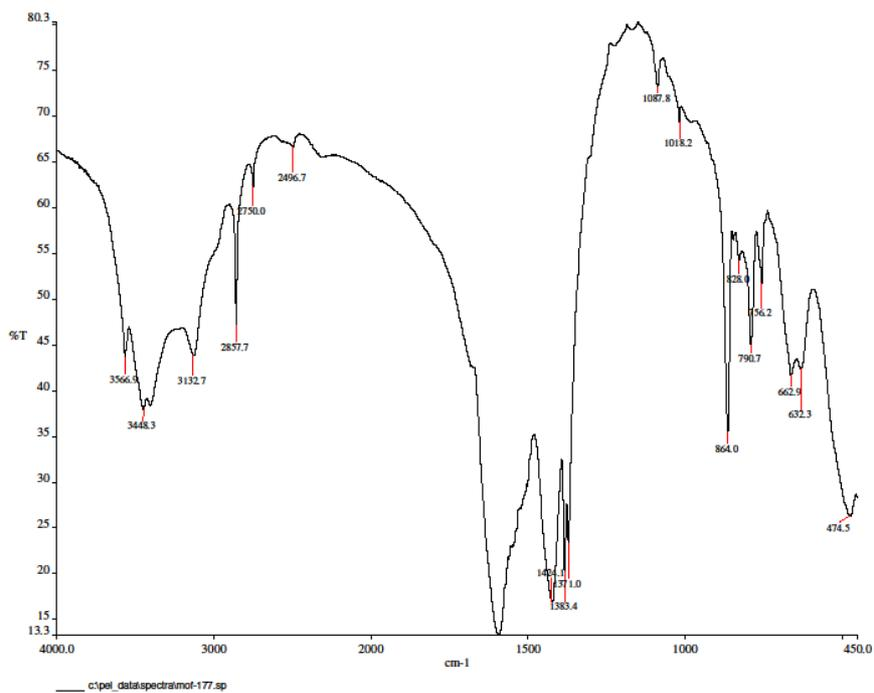
Figure 4. FT-IR spectra of MOF-177
