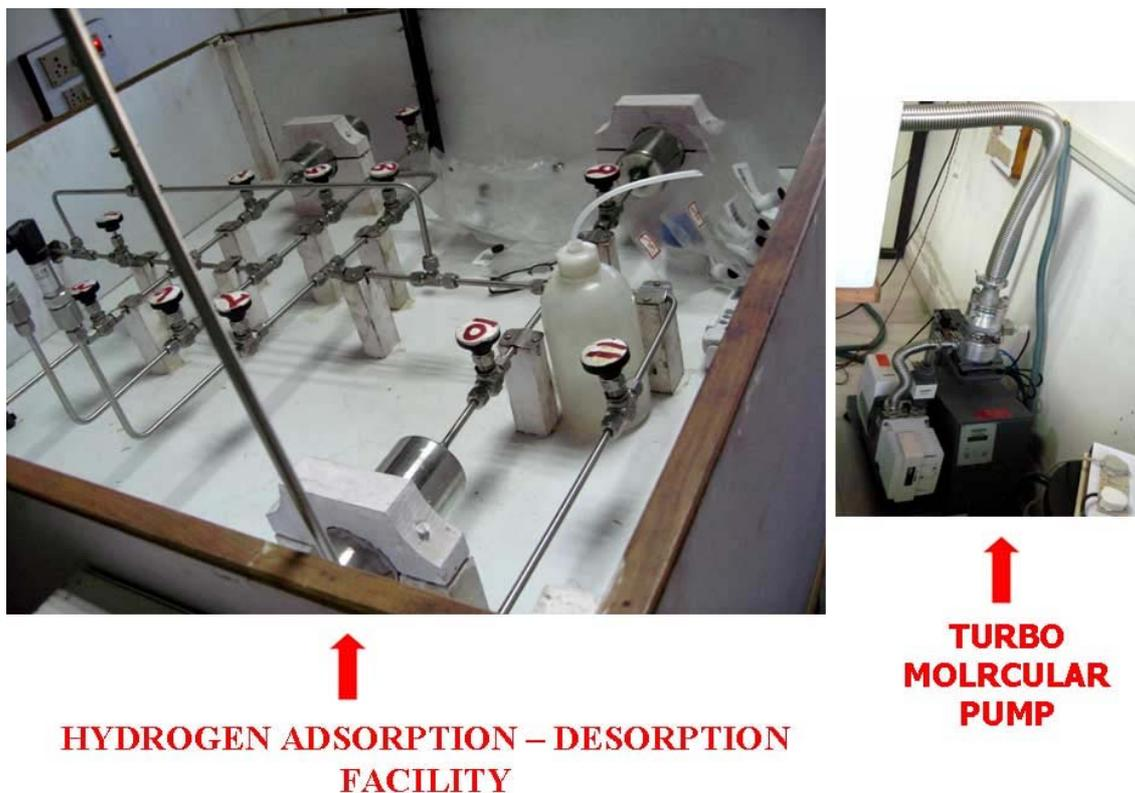
Figure 1. Hydrogen adsorption unit
