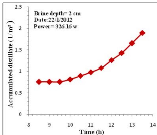
Figure 6. Time variation of accumulated distillate for still with brine depth of 2 cm
