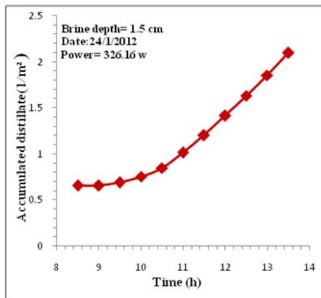
Figure 5. Time variation of accumulated distillate for still with brine depth of 1.5 cm
