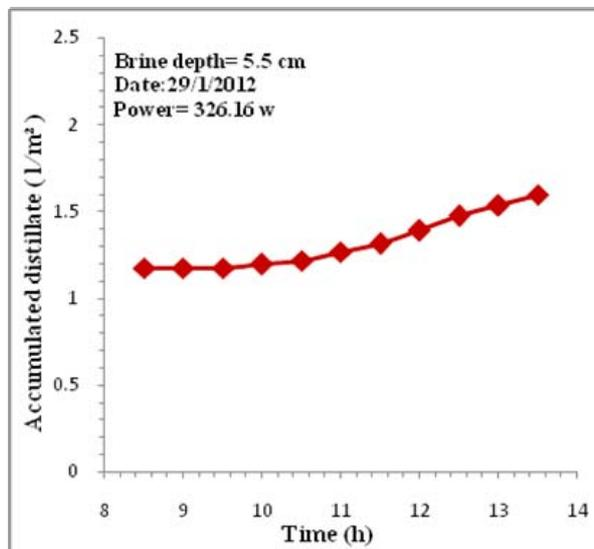
Figure 8. Time variation of accumulated distillate for still with brine depth of 5.5 cm
