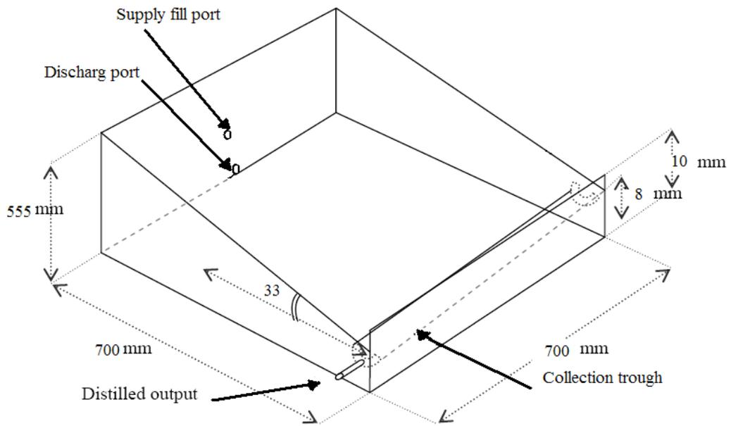
Figure 2. The schematic diagram of the experimental prototype
