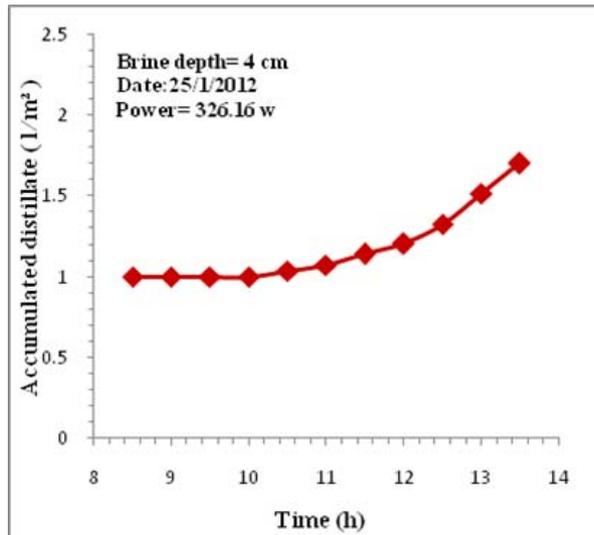
Figure 7. Time variation of accumulated distillate for still with brine depth of 4 cm.
