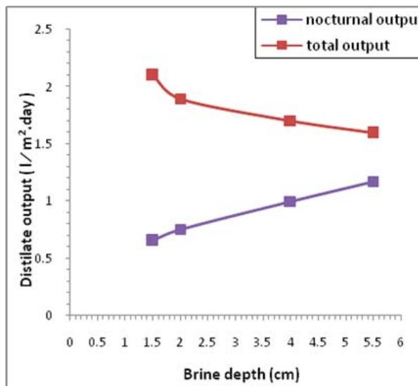
Figure 9. The total and nocturnal output for different brine depths
