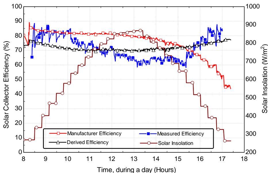
Figure 13. Efficiency of solar collector and solar insolation variations for entire day light in the Middle East
