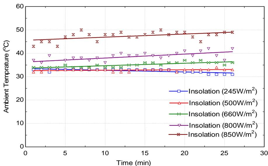
Figure 10. Ambient temperature under the solar simulator
