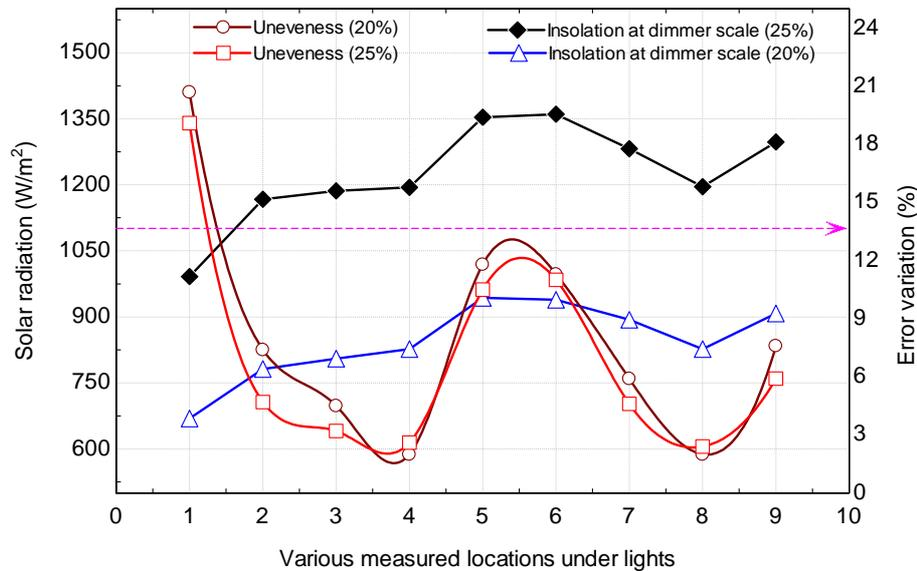
Figure 9. The unevenness and insulations under solar simulator at various spaced points
