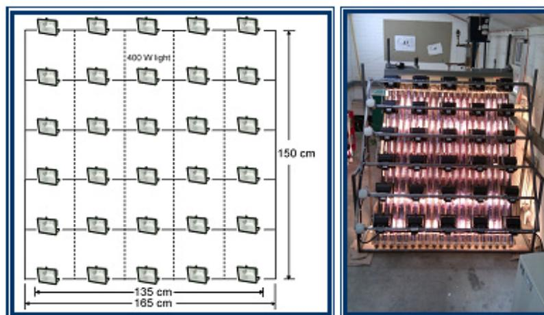
Figure 2. Test rig components
