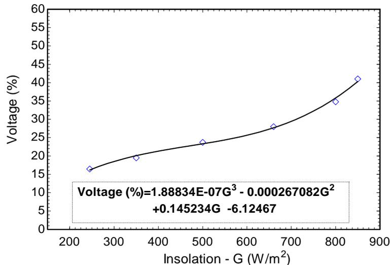
Figure 6. Solar insolation level versus transformer voltage calibration results
