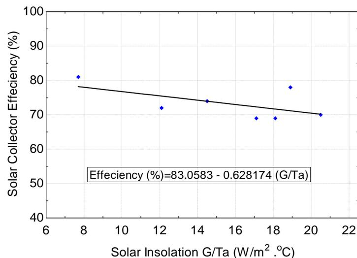
Figure 12. Experimental efficiency formula of solar collector
