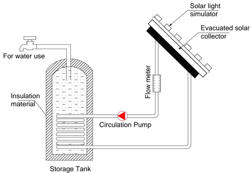
Figure 1. Schematic of experimental set-up of solar simulator with solar collector
