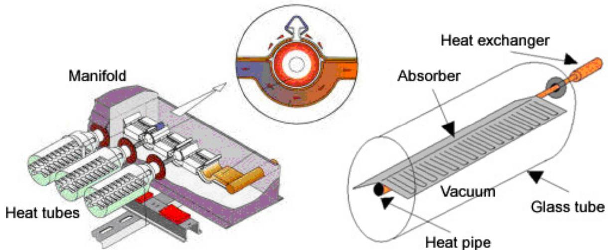
Figure 4. Evacuated solar collector manifolds and heat tubes assembly
