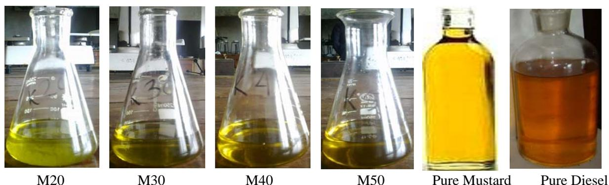
Figure 1. Sample color of different bio-diesel blends with kerosene, pure mustard and diesel
