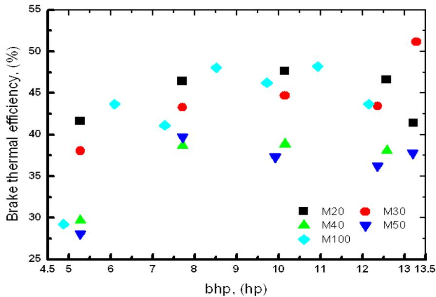
Figure 8. Variation of brake thermal efficiency with brake house power (bhp)
