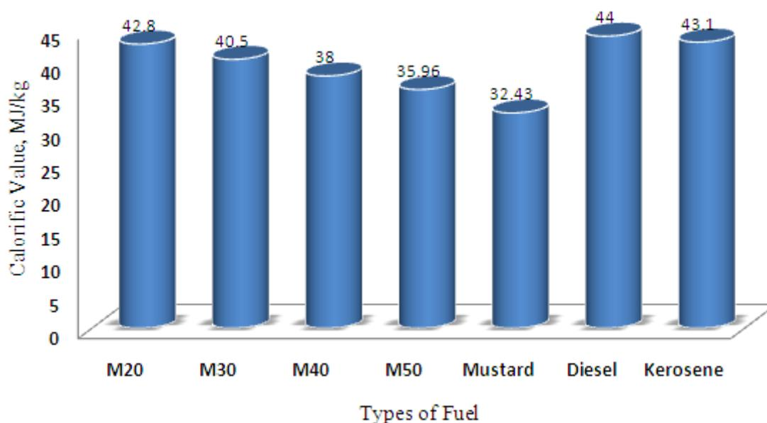
Figure 2. Lower calorific value in MJ/kg for different blends
