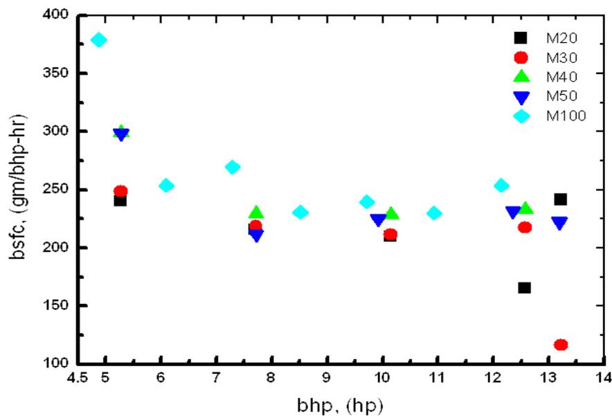
Figure 7. Variation of break specific fuel consumption (bsfc) with break house power (bhp)
