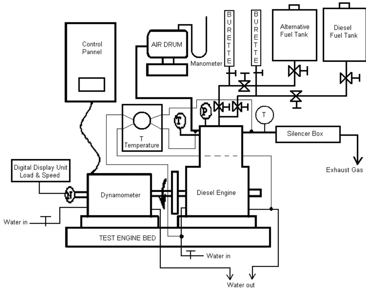
Figure 5. Schematic diagram of the experimental setup with hydraulic dynamometer
