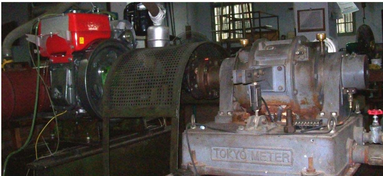
Figure 6. Test engine mounted on dynamometer bed
