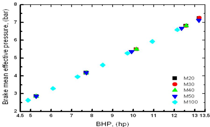
Figure 9. Variation of brake mean effective pressure with engine load
