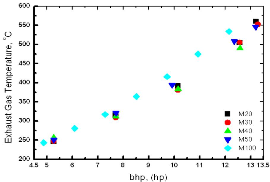
Figure 10. Variation of exhaust gas temperature with engine load
