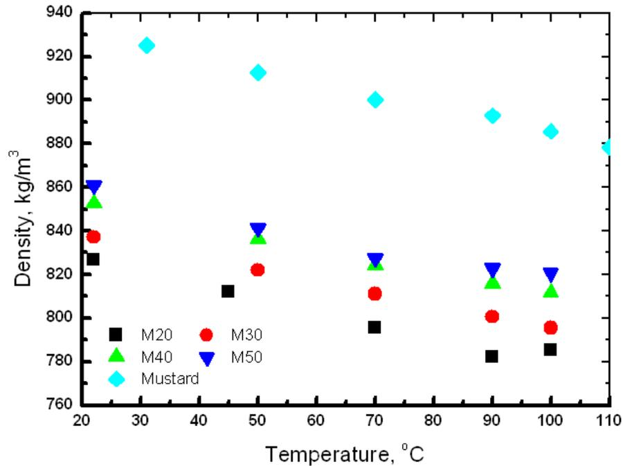
Figure 3. Variation of density with temperature for the different bio-fuel blends with kerosene.
