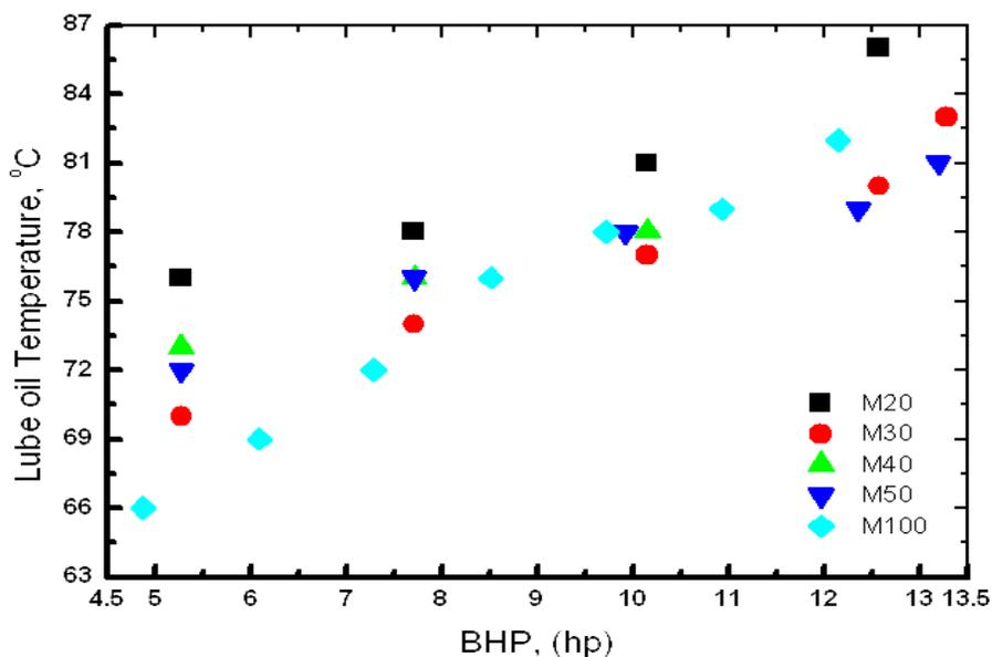
Figure 11. Variation of engine lube oil temperature with load
