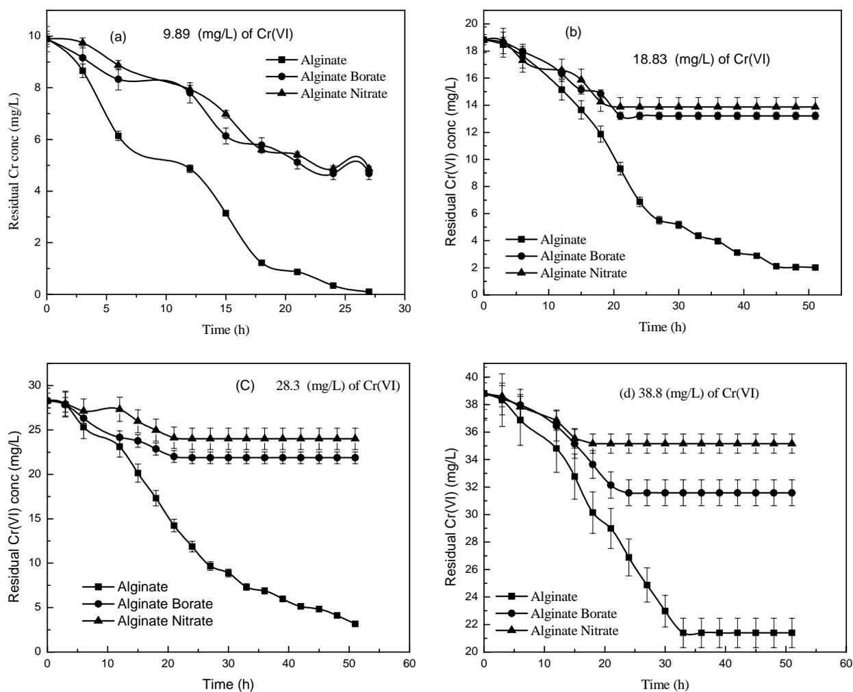
Figure 3. Cr(VI) reduction by *Halomonas* immobilized in Alginate beads : (a) Initial Cr(VI) concentration 9.89 (mg/L); (b) Initial Cr(VI) concentration 18.83 (mg/L); (C) Initial Cr(VI) concentration 28.3 (mg/L); Initial Cr(VI) concentration 38.8 (mg/L)
