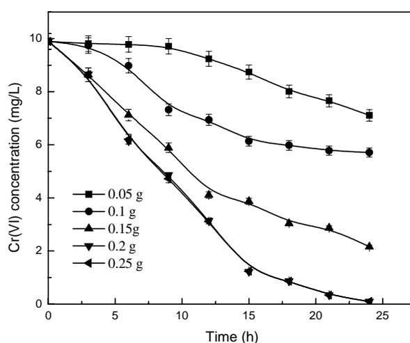
Figure 4. Effect of cell concentration on bioreduction of Cr(VI)
