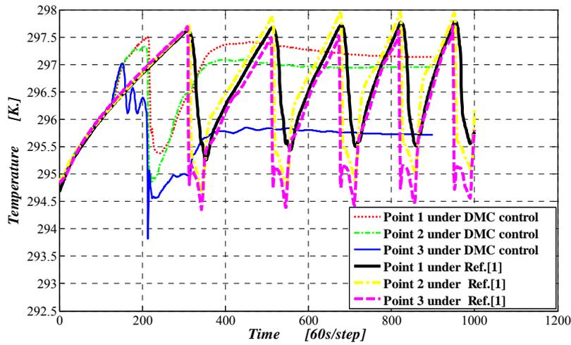
Figure 9. The comparison of temperature control results from Ref. [1] and the present fuzzy controller
