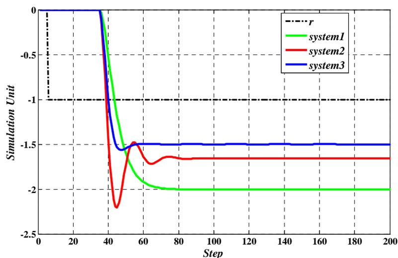
Figure 4. The three systems' open-loop step responses in group 1
