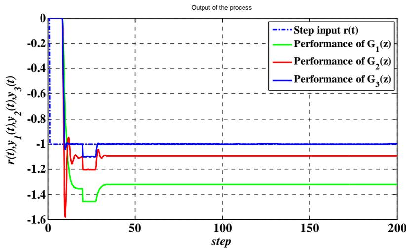
Figure 6. The three systems' closed-loop step responses only considering  $G_3(z)$ 's performance in group 1
