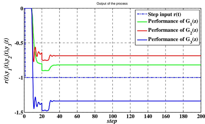
Figure 8. The three systems' closed-loop step responses considering three points' performance in group 2
