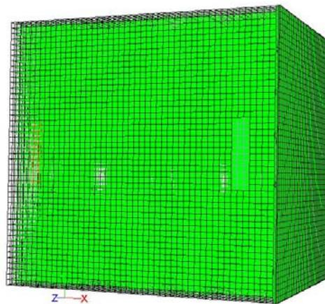
Figure 2. The 3-D Cartesian mesh inside the room
