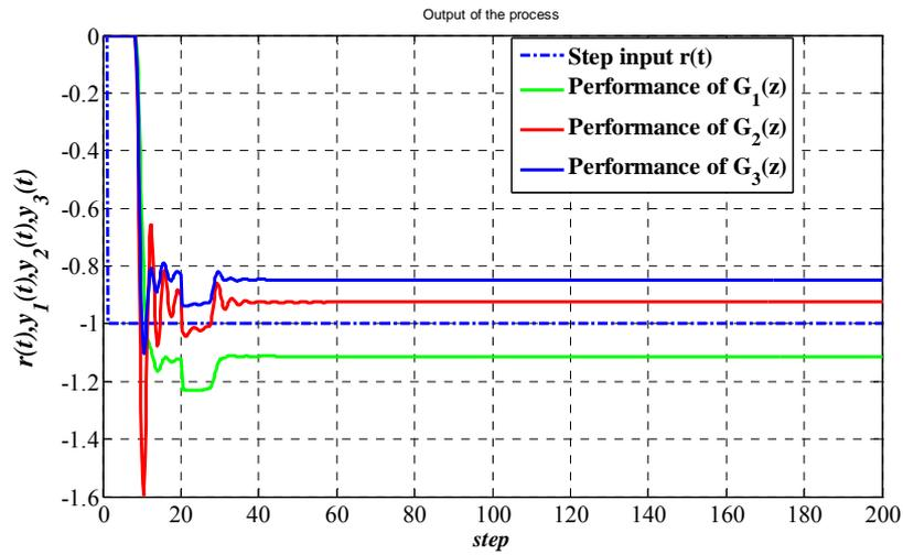
Figure 5. The three systems' closed-loop step responses considering three points' performance in group 1
