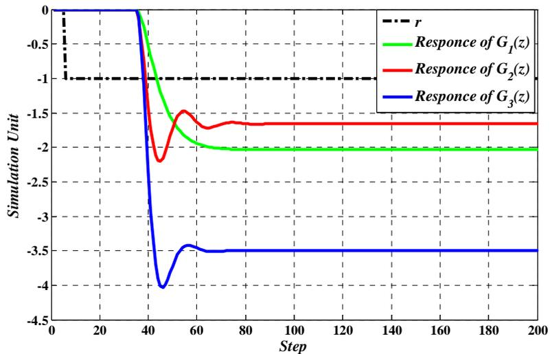
Figure 7. The three systems' open-loop step responses in group 2
