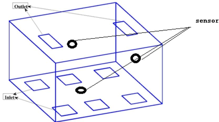
Figure 1. 3D view of the room with three sensors, two outlet vents and six inlet vents employed in displacement ventilation
