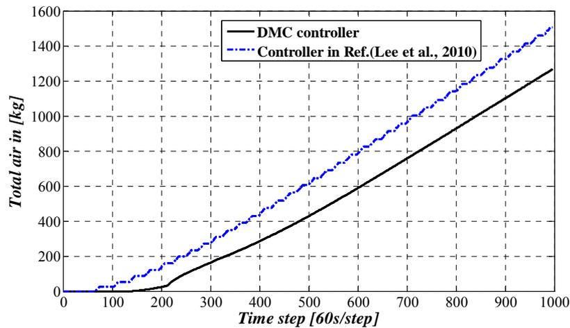
Figure 10. The cost of the cold air or energy saving using two different controllers
