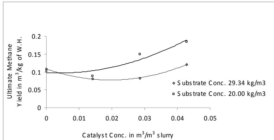
Figure 5. Plot of ultimate methane yield ( $B_o$ ) in m<sup>3</sup>/kg of W.H. against volume of catalyst used in ml at different water hyacinth concentrations
