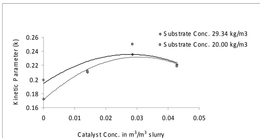
Figure 7. Plot of kinetic parameter (k) against volume of catalyst used in ml at different water hyacinth concentrations
