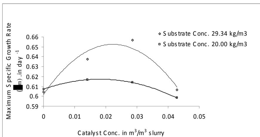
Figure 6. Plot of maximum specific growth rate ( $\mu_m$ ) in day $^{-1}$  against volume of catalyst used in ml at different water hyacinth concentration
