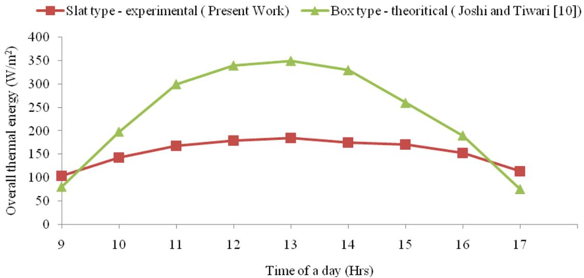
Figure 12. Hourly variation of experimental and theoretically predicted overall thermal energies
