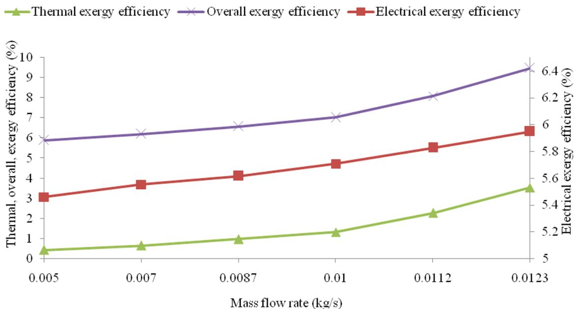
Figure 9. Thermal, electrical and overall thermal exergy efficiencies variation with air mass flow rate
