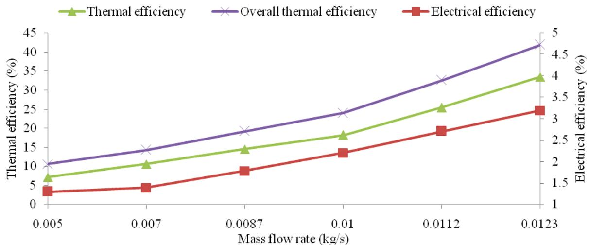
Figure7. Thermal, electrical and overall thermal efficiencies variation with air mass flow rate
