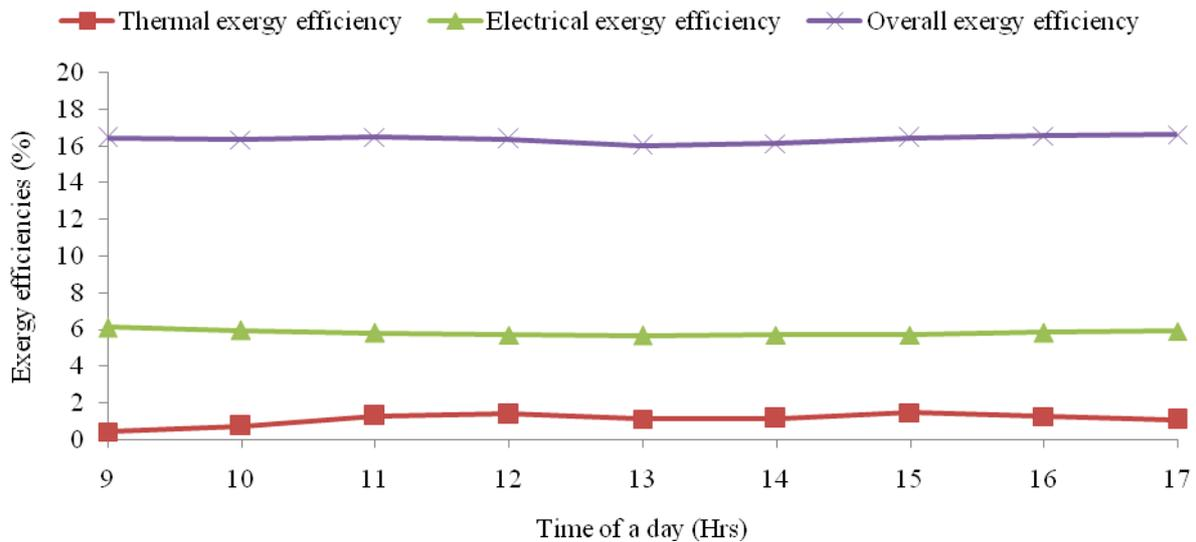
Figure 8. Hourly variation of thermal, electrical & overall exergy efficiencies
