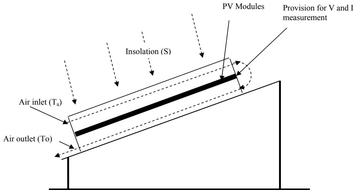
Figure 2. Schematic representation indicating locations of parameters measured
