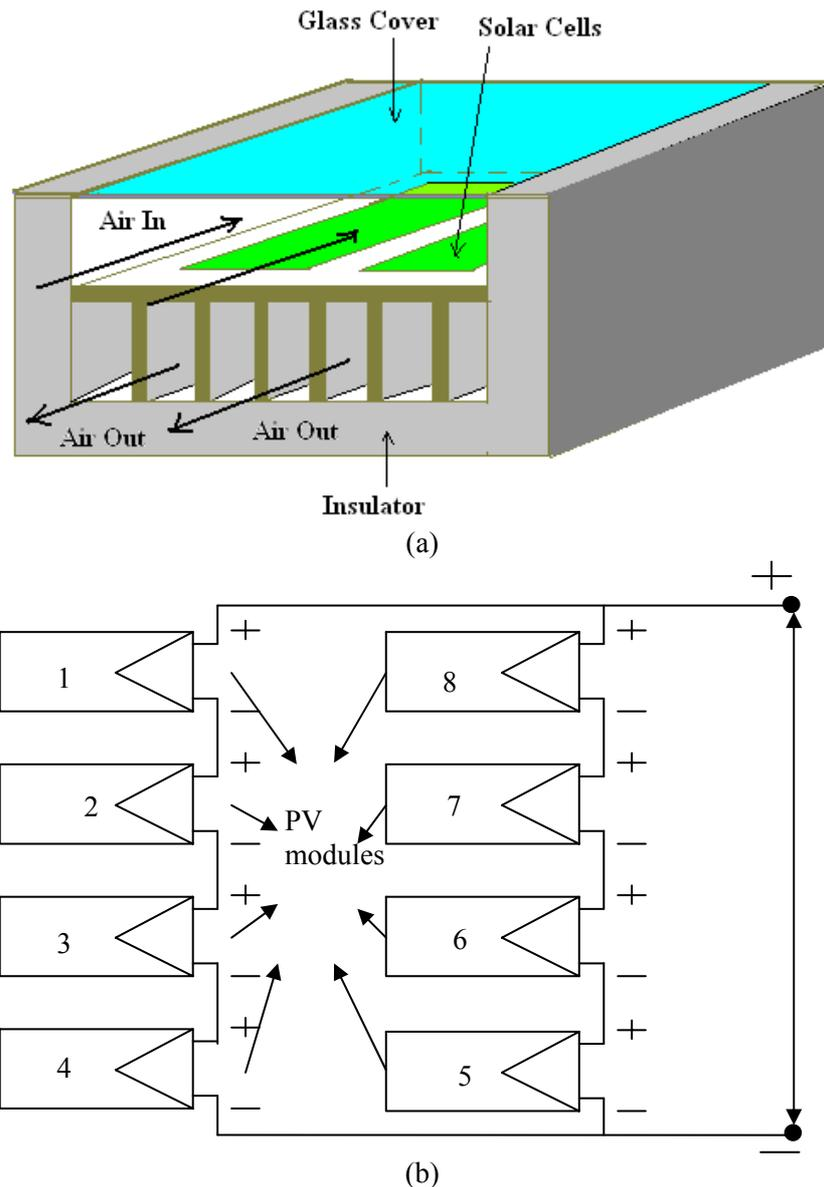
Figure 1. (a) Schematic diagram of DPHSAH with slats; (b) Schematic representation of PV module connections
