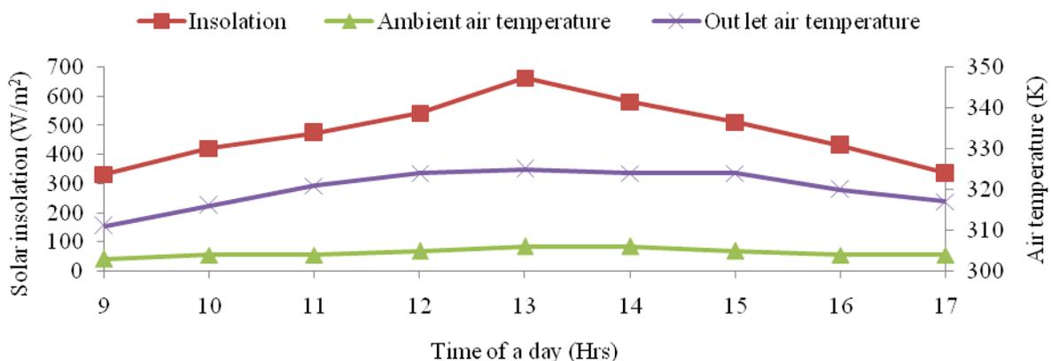
Figure 5. Hourly variation of solar insolation and fluid temperatures
