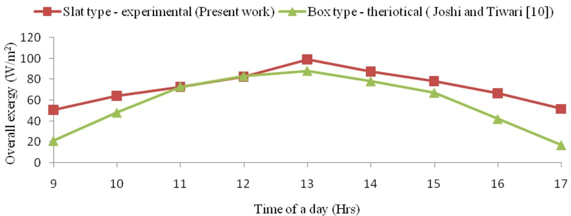
Figure 13. Hourly variation of experimental and theoretically predicted overall thermal exergy values
