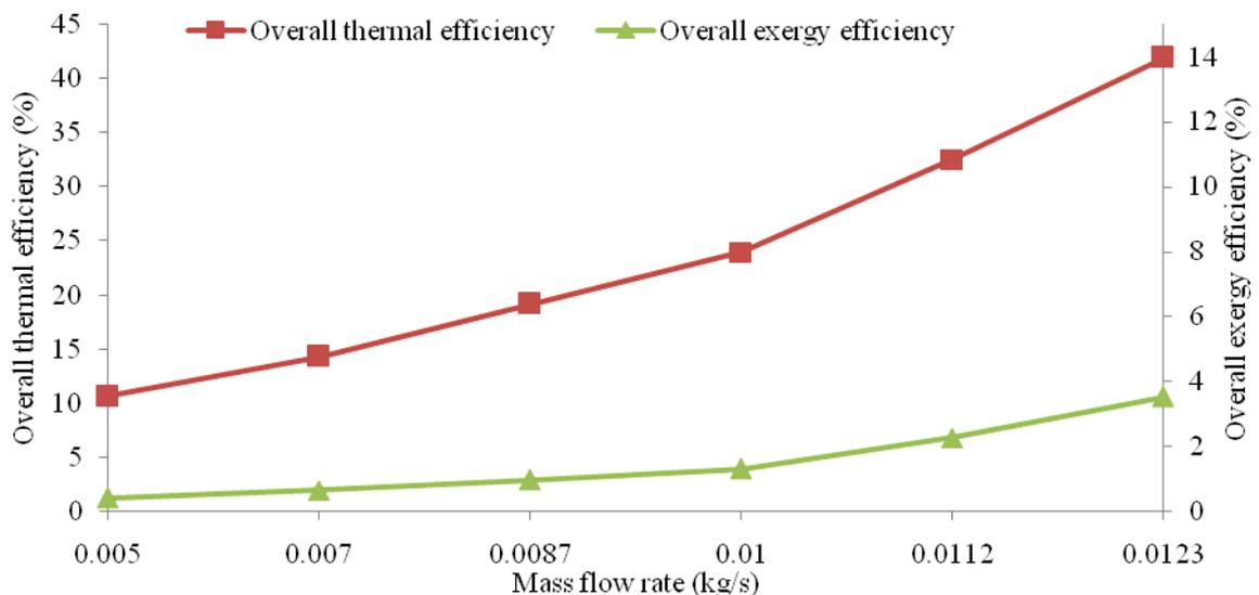
Figure 11. Overall thermal and overall exergy variation with mass flow rate
