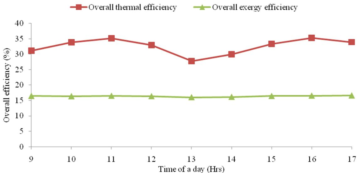
Figure 10. Hourly variation of overall energy and overall exergy efficiencies
