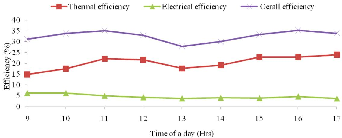
Figure 6. Hourly variation of thermal, electrical and overall thermal efficiencies
