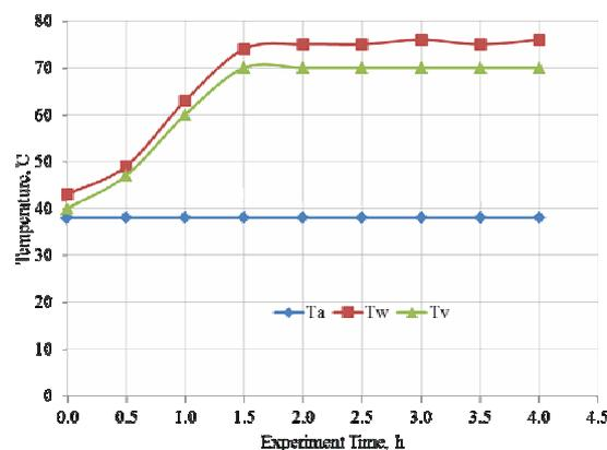
Figure 7. Time variation of the system temperatures using electrical heater only at 75 °C set point
