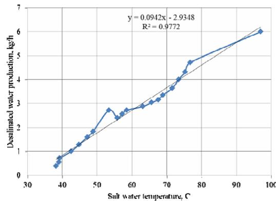
Figure 11. Effect of the salt-water temperature on the desalinated water production
