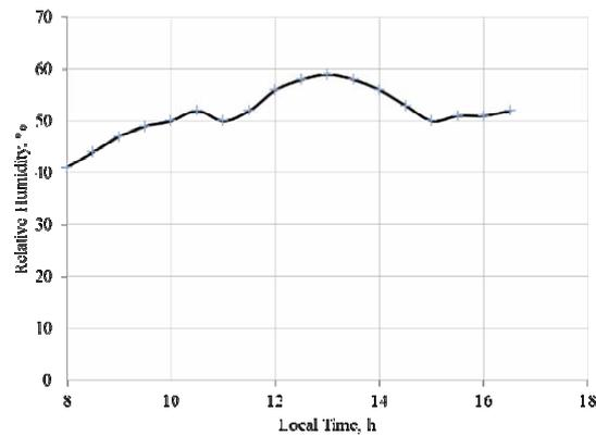
Figure 5. Time variation of relative humidity inside the condenser humidity using solar energy only at May 7, 2010
