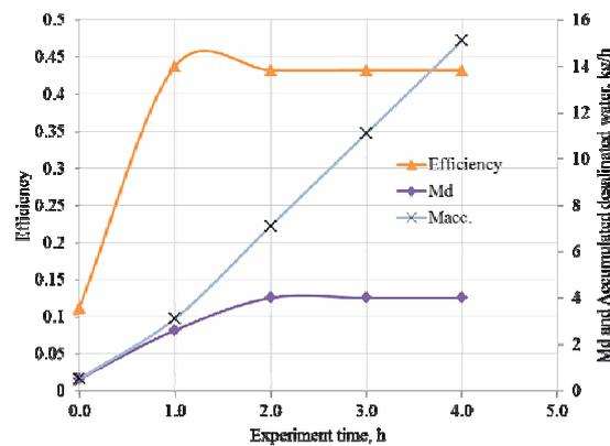
Figure 6. Time variation of the system production and efficiency using electrical heater only at 75 °C set point
