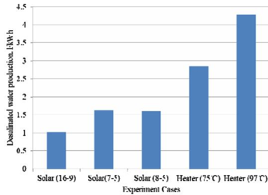
Figure 10. Desalinated water production per kWh of input energy
