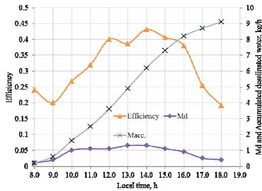
Figure 2. Time variation of the system production and efficiency using solar energy only at Sept. 16, 2010
