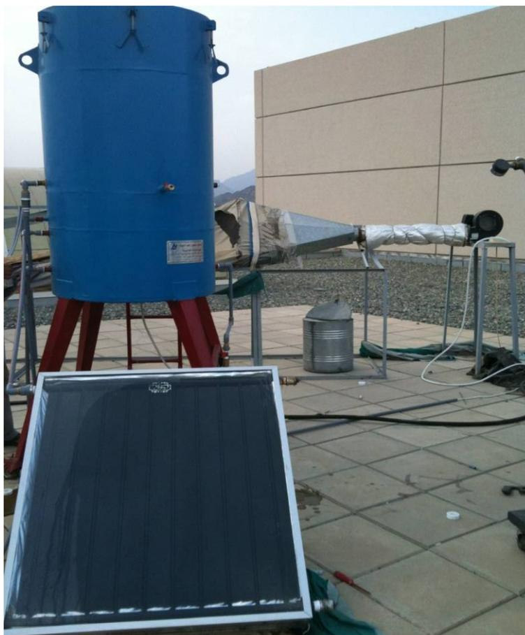
Figure 1. (a) Schematic diagram of the solar desalination system; (b) Photograph of the solar water desalination system
