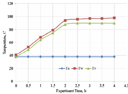
Figure 9. Time variation of the system temperatures using electrical heater only at 97 °C set point
