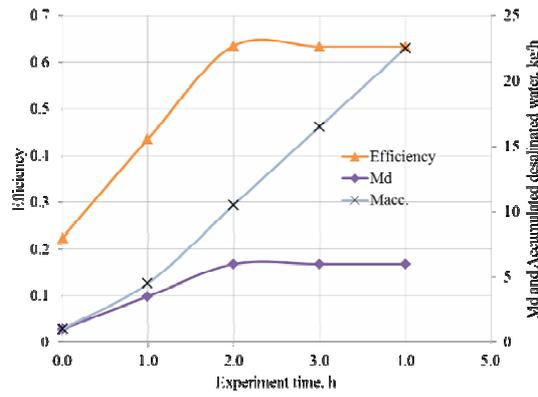
Figure 8. Time variation of the system production and efficiency using electrical heater only at 97 °C set point
