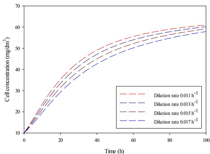
Figure 5. Cell concentration as function of time and dilution rate (Chemostat without recycle, *Bacillus* sp.)
