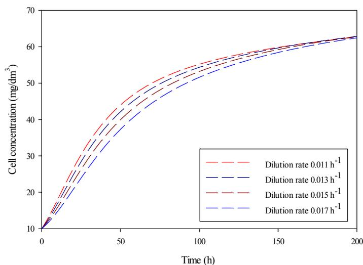
Figure 7. Cell concentration as function of time and dilution rate (Chemostat with recycle, *Pseudomonas* sp.)
