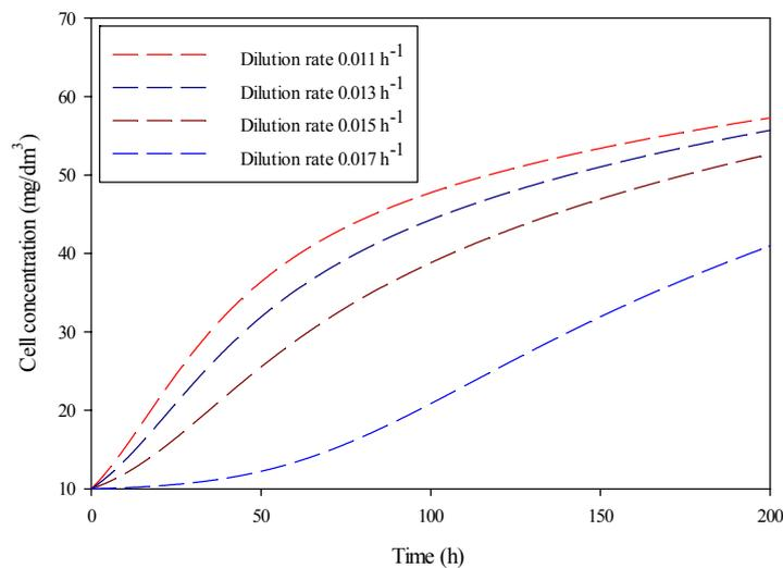
Figure 3. Cell concentration as function of time and dilution rate (Chemostat without recycle, *Pseudomonas* sp.)
