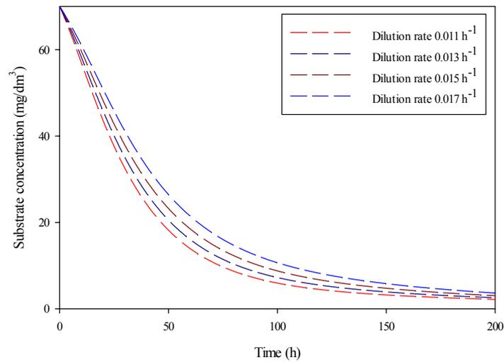
Figure 8. Substrate concentration as function of time and dilution rate (Chemostat with Recycle, *Pseudomonas* sp.)
