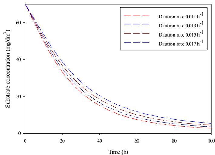
Figure 6. Substrate concentration as function of time and dilution rate (Chemostat without recycle, *Bacillus* sp.)
