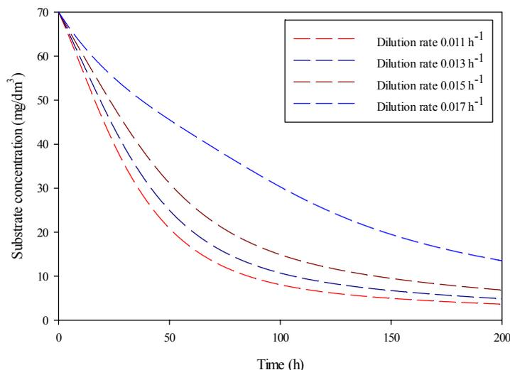
Figure 4. Substrate concentration as function of time and dilution rate (Chemostat without recycle, *Pseudomonas* sp.)
