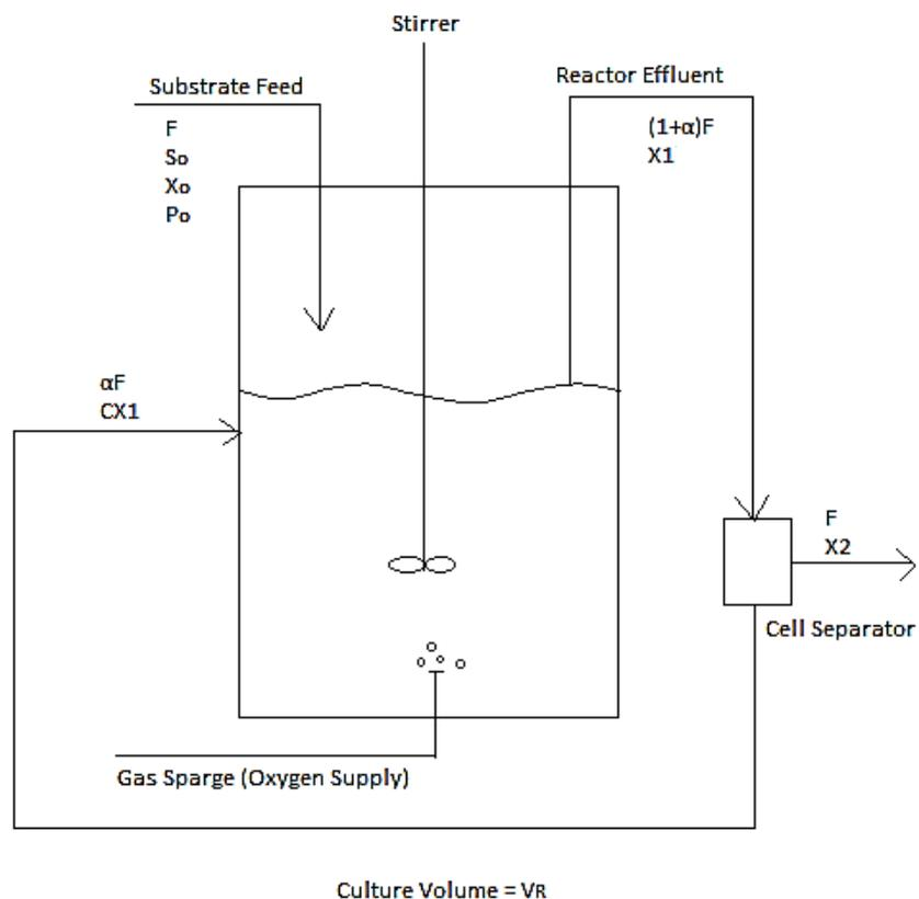
Figure 2. Chemostat with recycle
