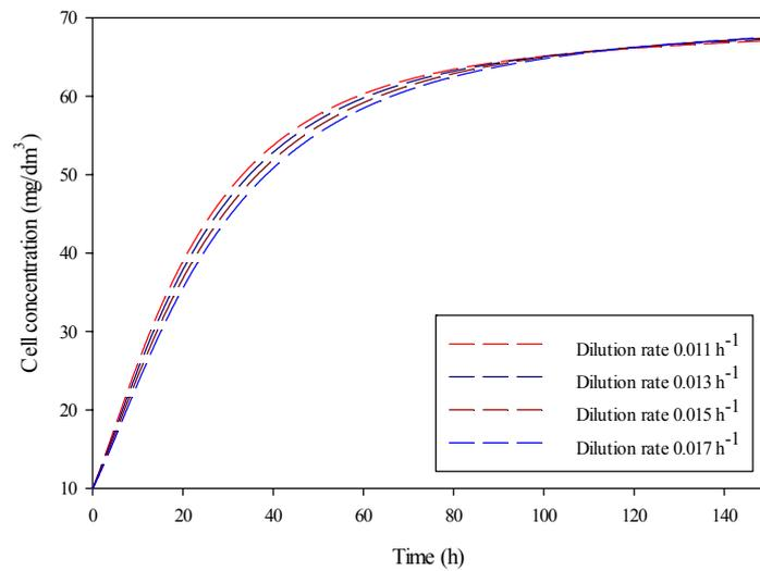
Figure 9. Cell concentration as function of time and dilution rate (Chemostat with Recycle, *Bacillus* sp.)
