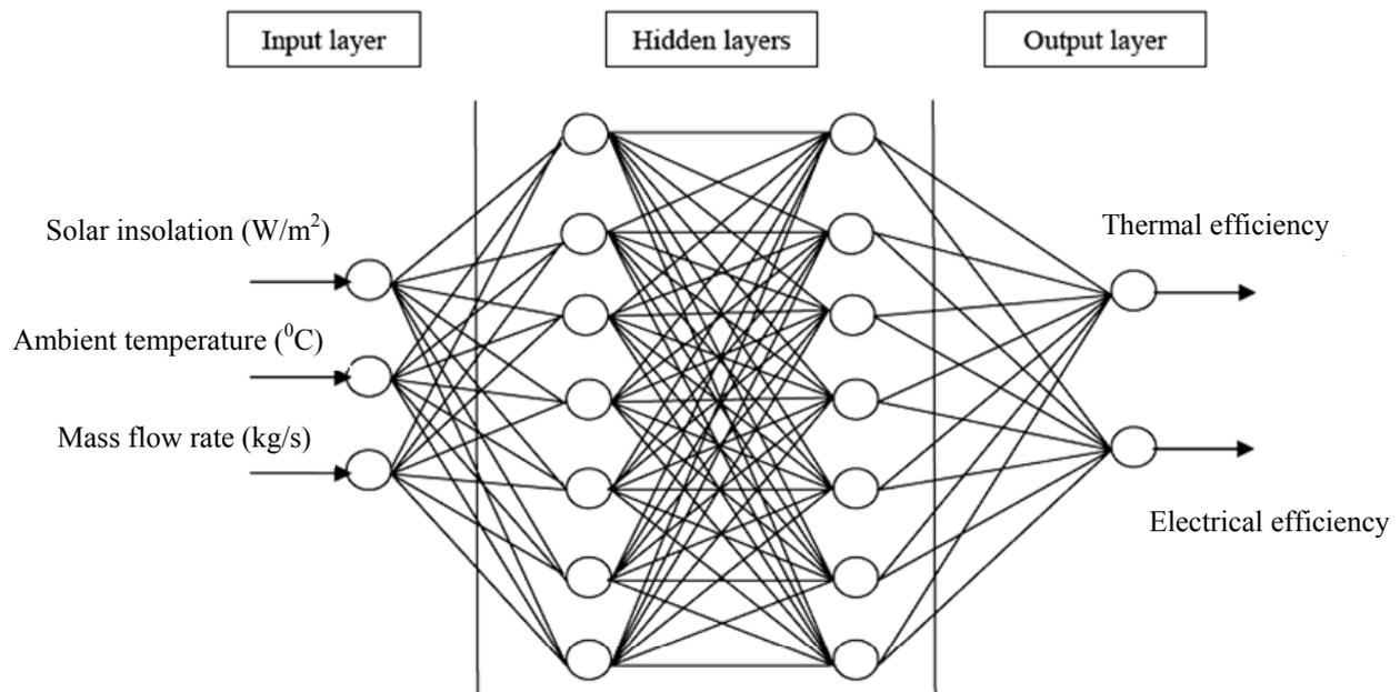
Figure 5. Architecture of ANN used for the performance prediction
