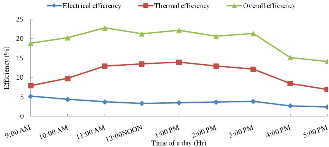
Figure 11. Variation of electrical, thermal and overall efficiencies (22 February 2011)
