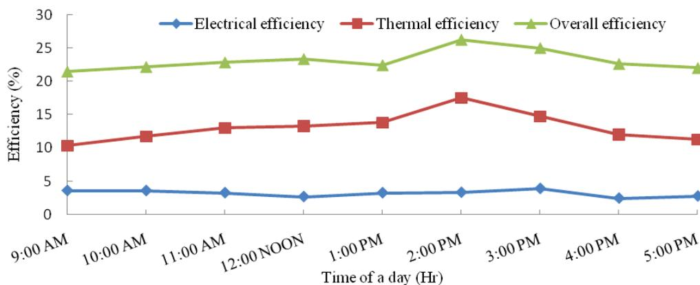
Figure 10. Variation of electrical, thermal and overall efficiencies (21 January 2011)
