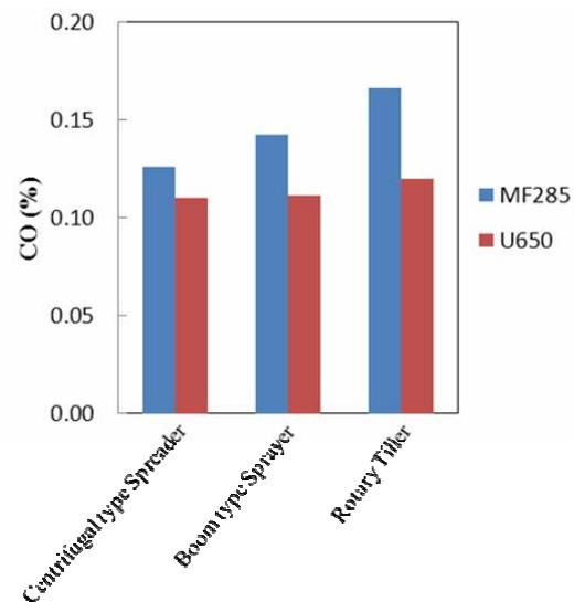
Figure 3. CO emission from tractors at operation conditions
