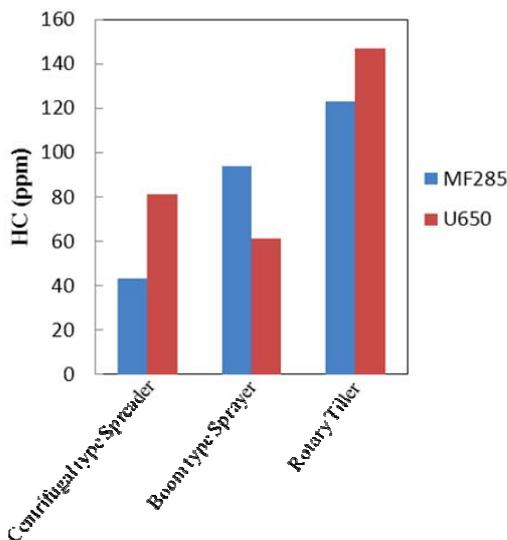
Figure 2. HC emission from tractors at operation conditions
