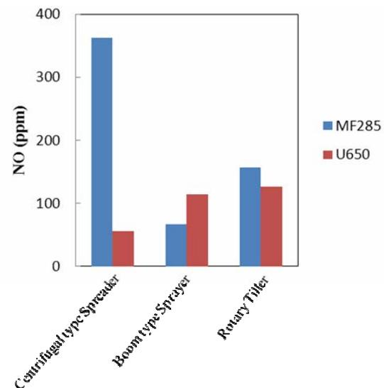
Figure 5. NO emission from tractors at operation conditions
