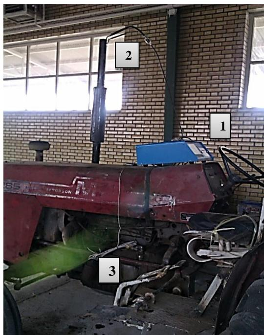
Figure 1. Details of specific device (1. Gas analyzer, 2. Gas inlet, 3. Oil temperature sensor)
