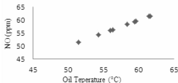
Figure 6. Relationship between NO emission and engine oil temperature
