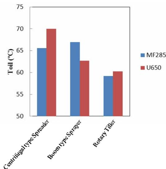
Figure 8. Engine oil temperature from tractors at operation conditions
