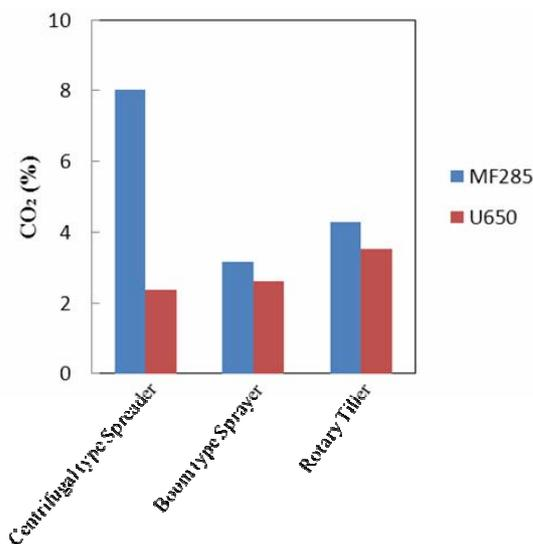
Figure 4. CO<sub>2</sub> emission from tractors at operation conditions
