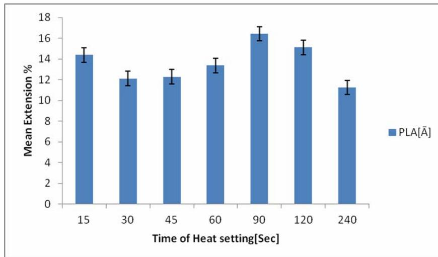
Figure 5. Mean [Å] of effect of time of heatsetting on the tensile extension EM [%] of Ingeo™ Poly (lactic acid)
