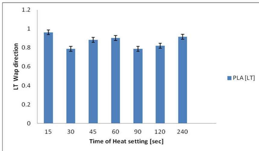
Figure 6. Effect of time of heatsetting on the linearity of load extension in warp direction of knitted Ingeo™ Poly (lactic acid) fabric
