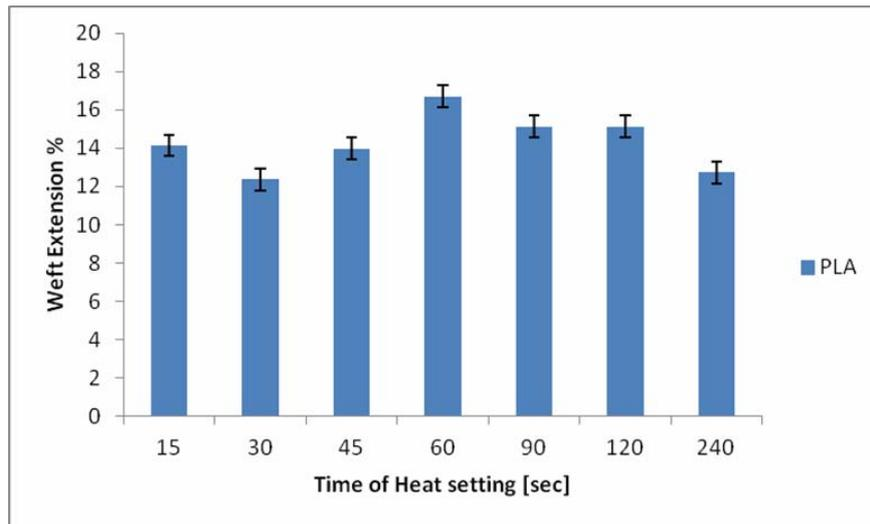
Figure 4. Effect of time of heatsetting on the tensile Extension EM [%] in Weft direction of knitted Ingeo™ Poly (lactic acid) [PLA]
