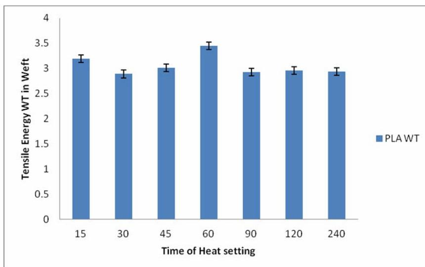
Figure 10. Effect of time of heatsetting on tensile energy WT g.cm/cm<sup>2</sup> in weft direction
