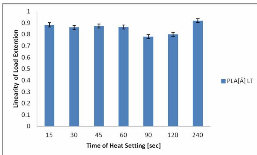
Figure 8. Mean effect of time of heatsetting on the linearity of load extension LT of knitted Ingeo™ Poly (lactic acid) (PLA) fabric
