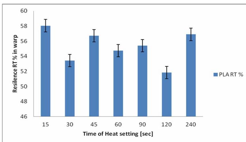
Figure 12. Effect of time of heatsetting on tensile resilience RT [%] in warp direction of knitted Ingeo Poly (lactic acid)
