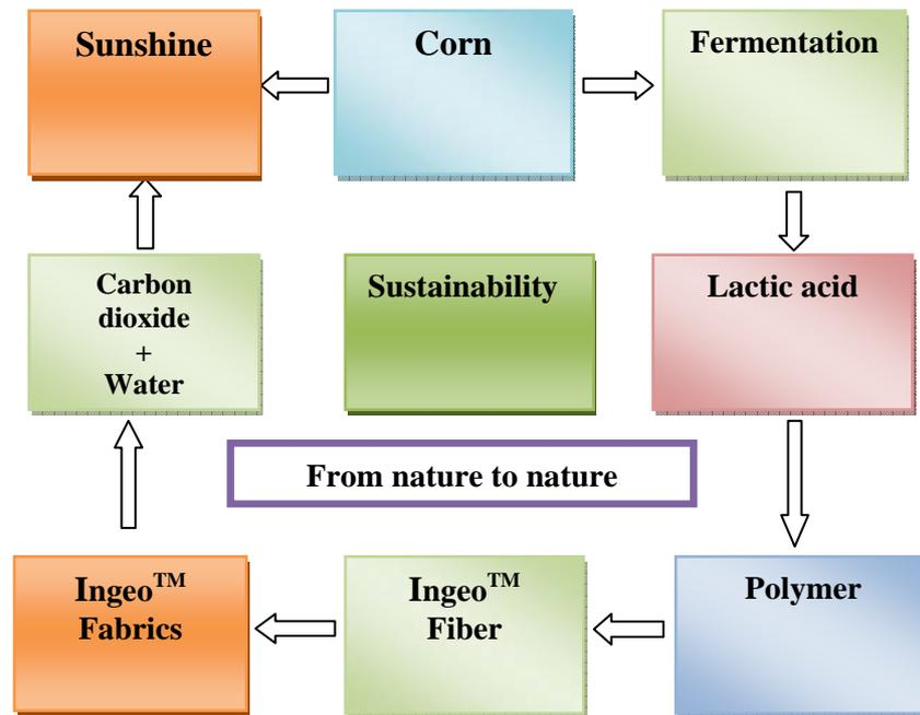
Figure 1. Production cycle of Ingeo™
