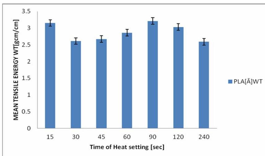
Figure 11. Mean effect of time of heatsetting on tensile energy WT g.cm/cm<sup>2</sup> of knitted Ingeo Poly lactic acid fabric
