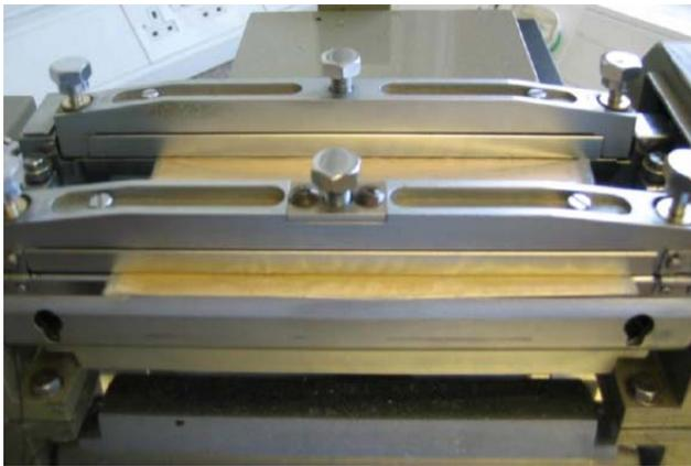
Figure 2. KES-FB 1 tensile tester
