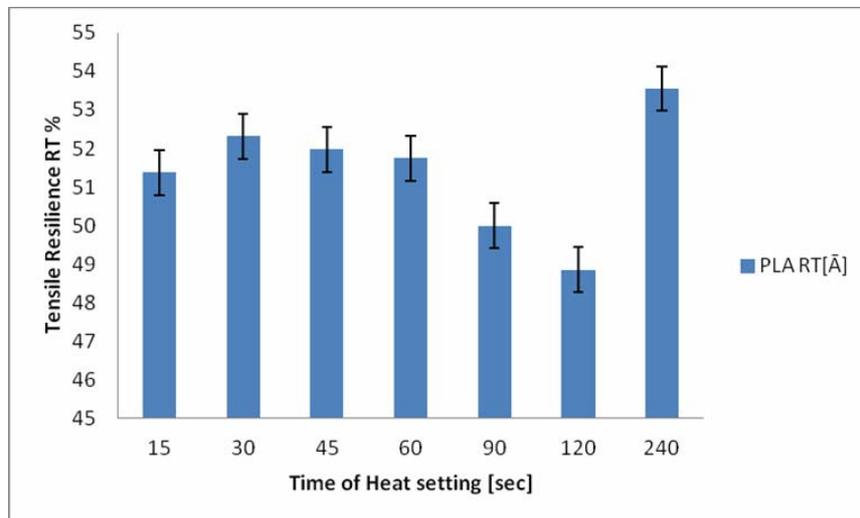
Figure 14. Mean effect of time of heatsetting on tensile resilience RT % on knitted Ingeo Poly (lactic acid) (PLA) fabric
