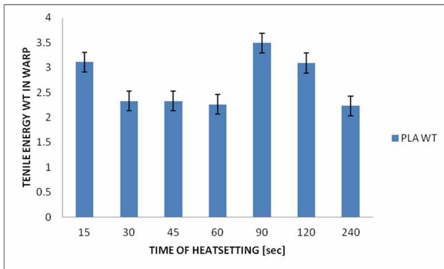
Figure 9. Effect of time of heatsetting on tensile energy WT g.cm/cm<sup>2</sup> in warp direction of knitted Ingeo Poly (lactic acid) fabric
