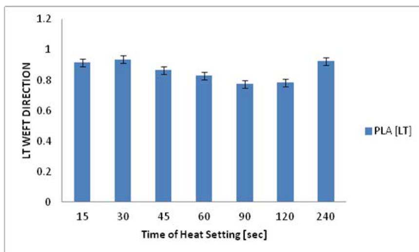
Figure 7. Effect of time of heatsetting on the linearity of load extension in weft direction of knitted Ingeo™ Poly (lactic acid)
