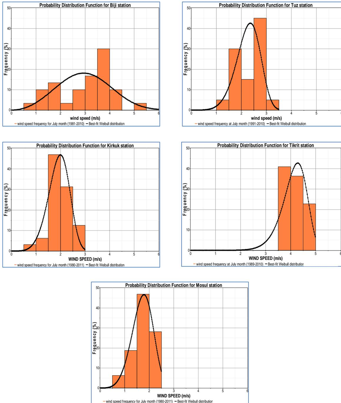
Figure 5. Histogram of the wind speed distributions simulated by Weibull function during July for the sites Biji, Tuz, Tikrit, Kirkuk, Mosul
