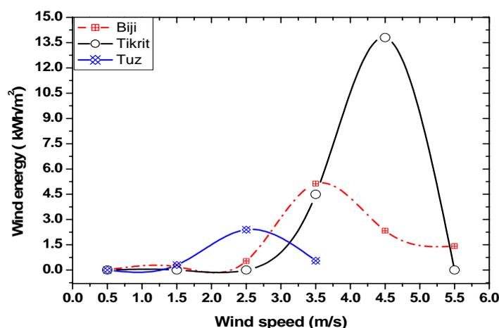
Figure 7. Maximum energy density during July for Tikrit, Biji and Tuz stations
