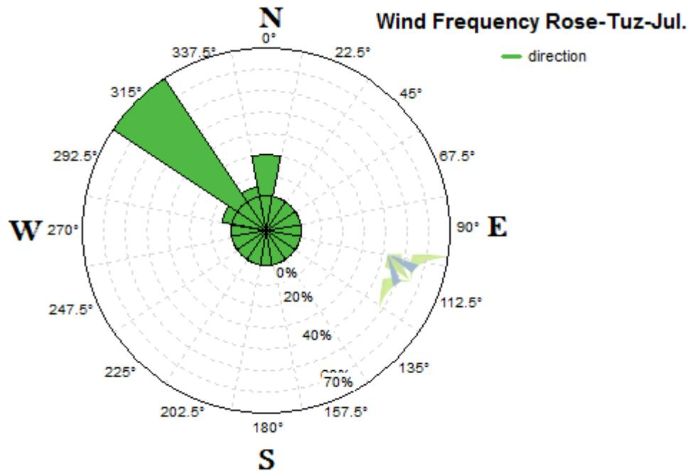
Figure 3. Wind direction frequency (wind rose) at July month for Tuz station (1991-2010)
