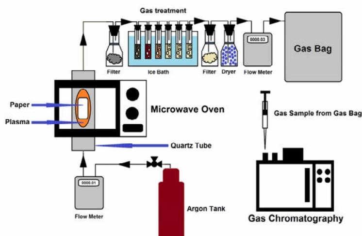
Figure 1. Experimental setup of the microwave plasma reactor for pyrolysis of waste paper
