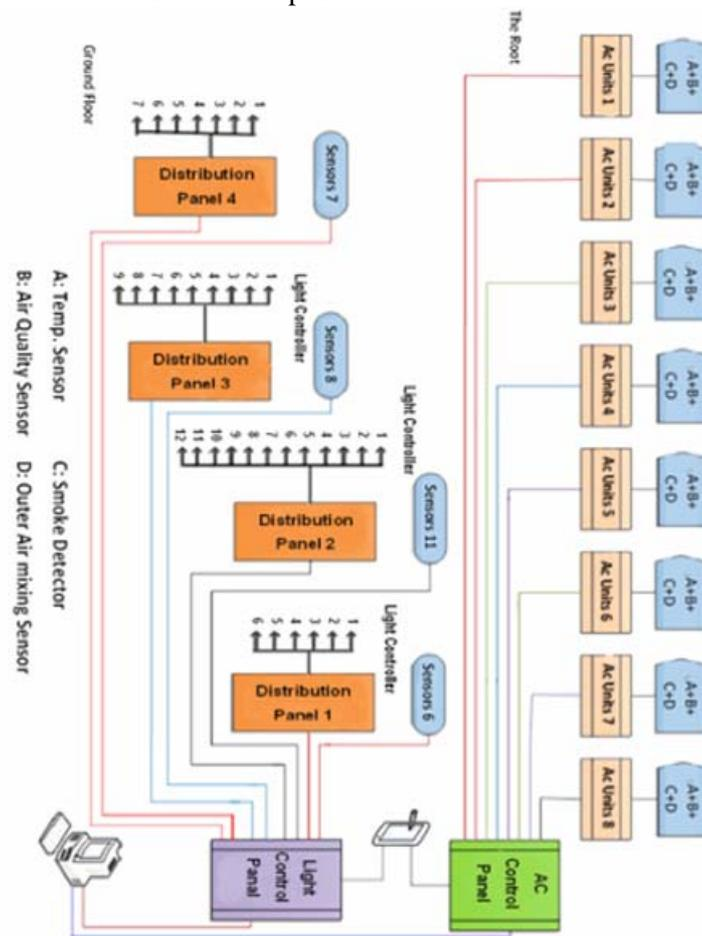
Figure 1. Schematic diagram of the BMS in a typical building
